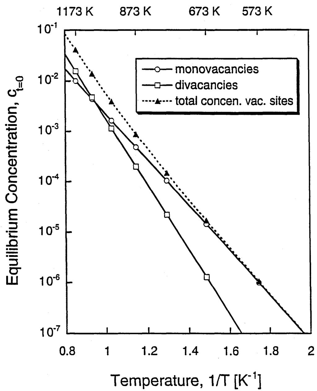
Fig. 5. Vacancy and divacancy concentrations in Fe-39Al as a function of temperature.
