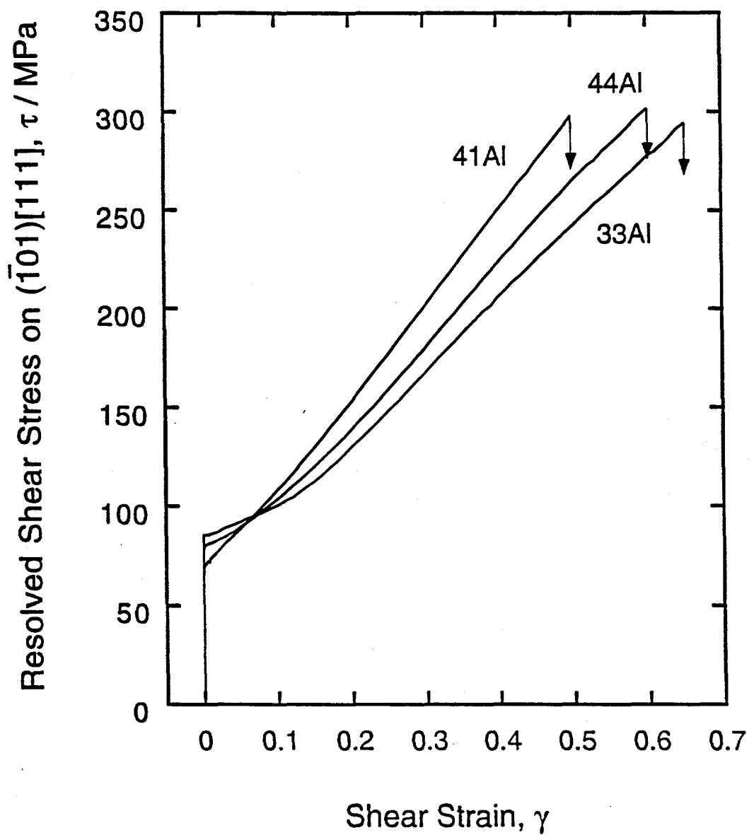
Fig. 1. Resolved shear stress-strain curves of as-homogenized Fe-33, 41 and 44 mol.% Al single crystals.
