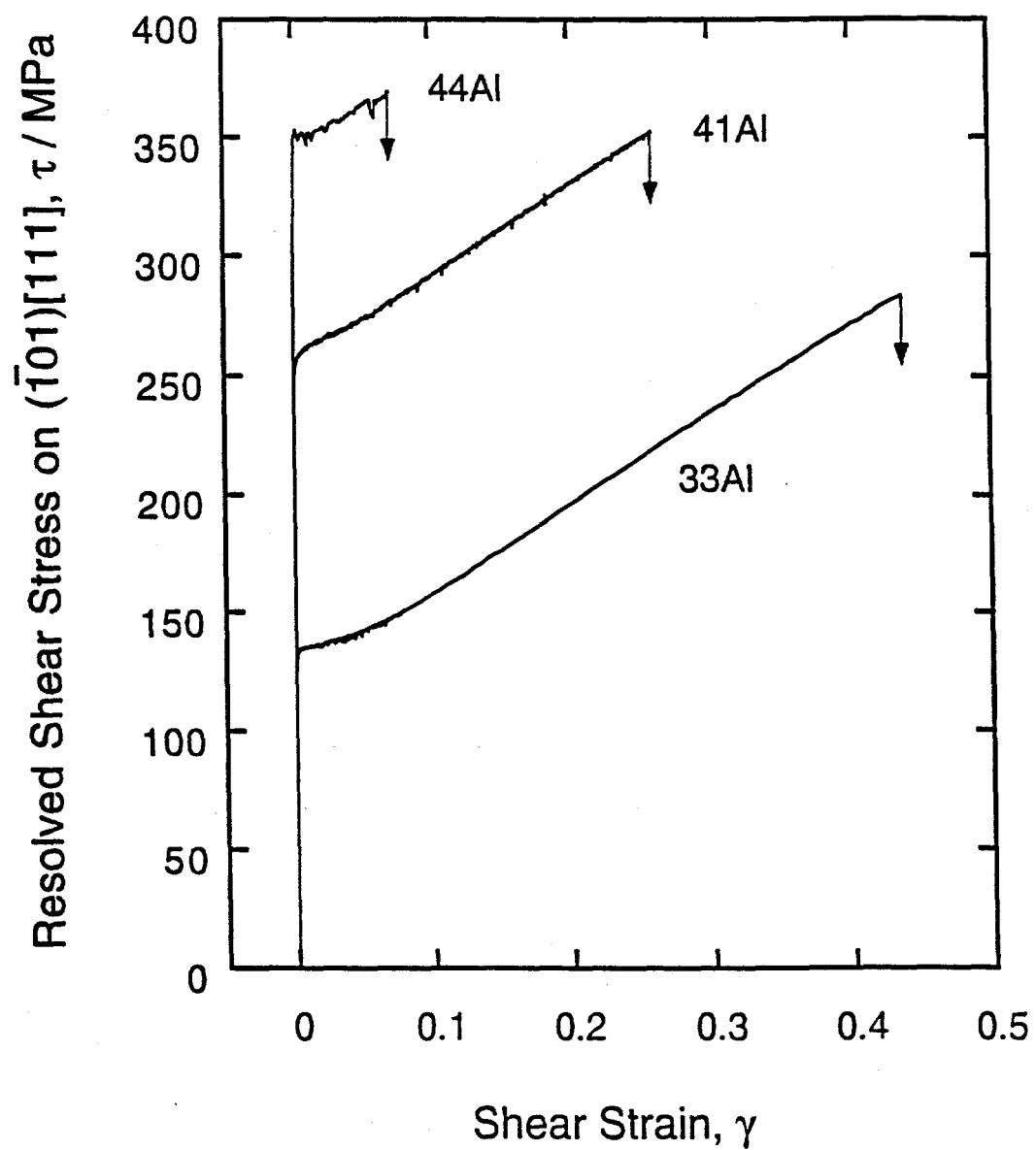
Fig. 2. Resolved shear stress-strain curves of fast-cooled Fe-33, 41 and 44 mol. % Al single crystals.
