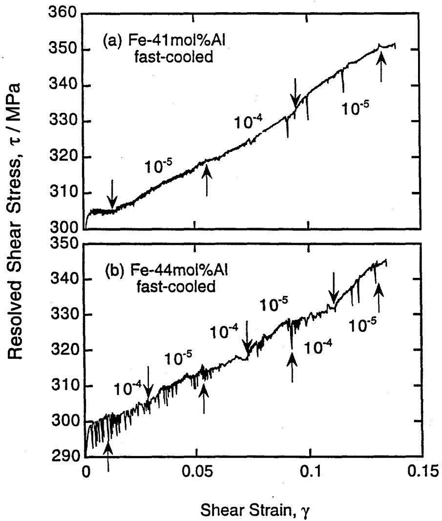
Fig. 4. Highly magnified resolved shear stress-strain curves of fast-cooled (a) Fe-41 mol.% Al and (b) Fe-44 mol.% Al during strain-rate change tests.
