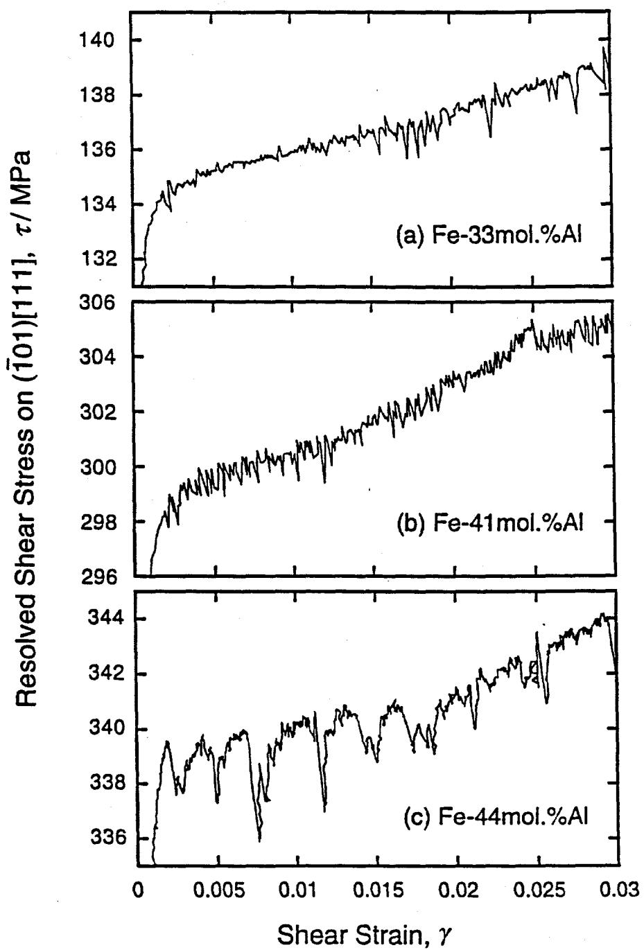
Fig. 3. Serrated flow of fast-cooled tensile specimens. (a) Fe-33mol.%Al. (b) Fe-41mol.%Al. (c) Fe-44mol.Al.
