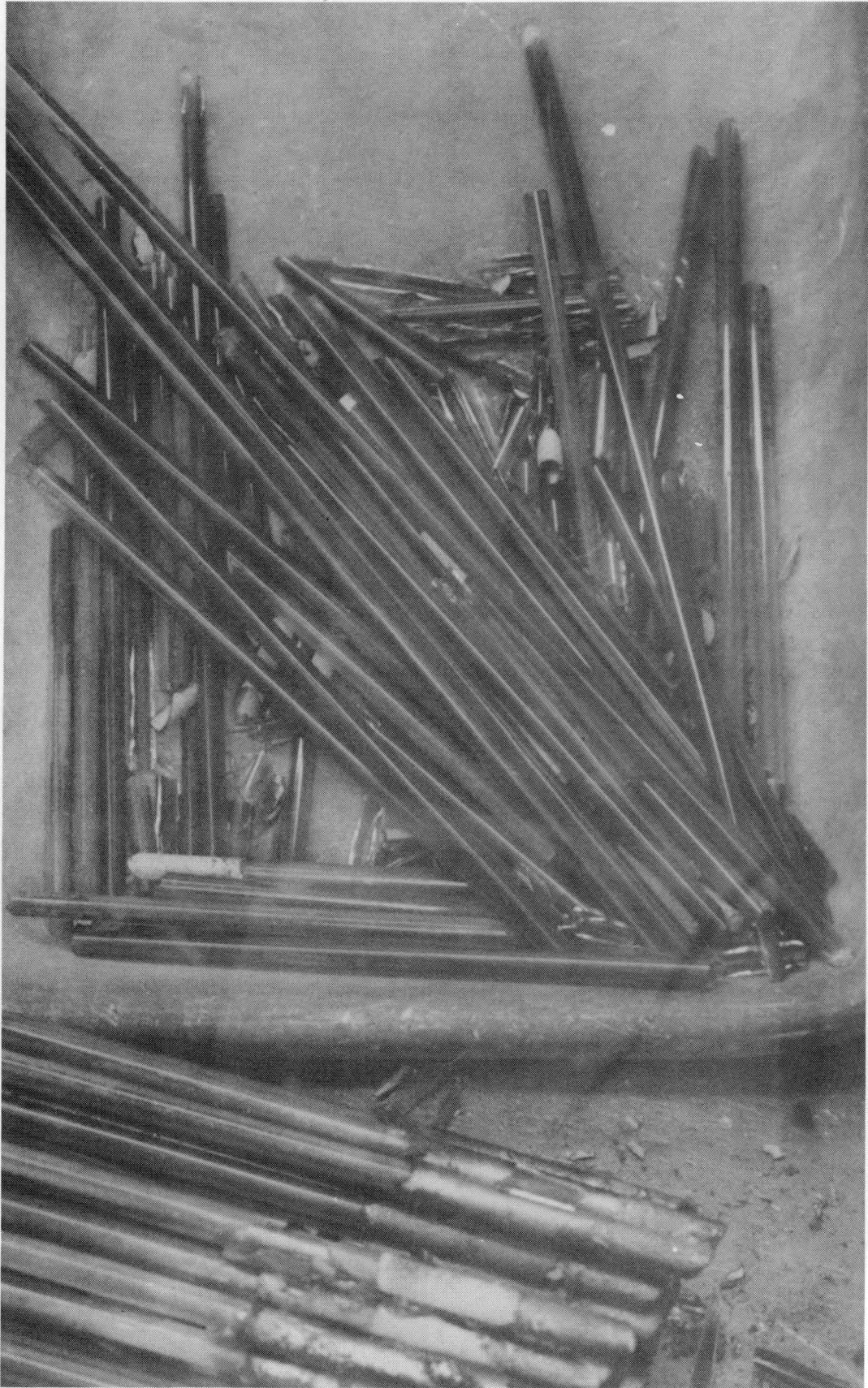
Fig. 17. Glass/Dust Broken Glass from Quartz Molds After Demolding
