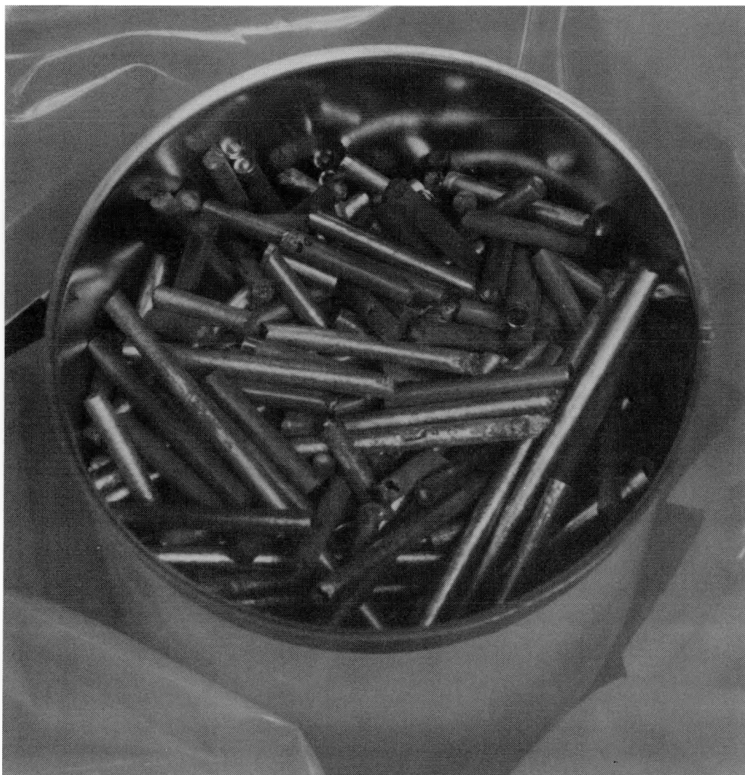
Fig. 6. Slug/Fines Small Pieces of U-Zr Alloy Sheared from Slugs and Chopped Reject Slugs
