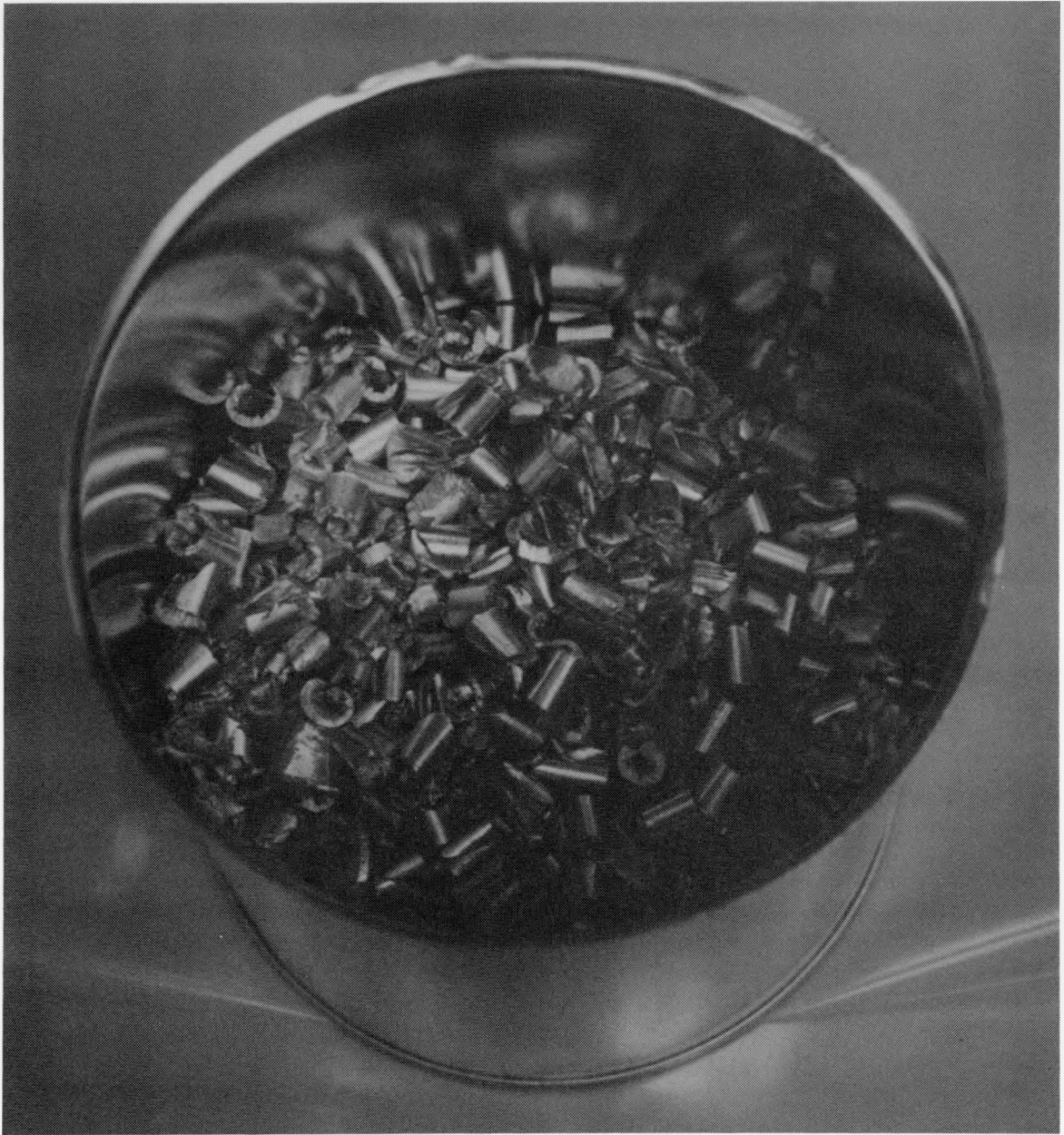
Fig. 7. Zirconium Feed Material Added to Attain Specified Alloy Composition
