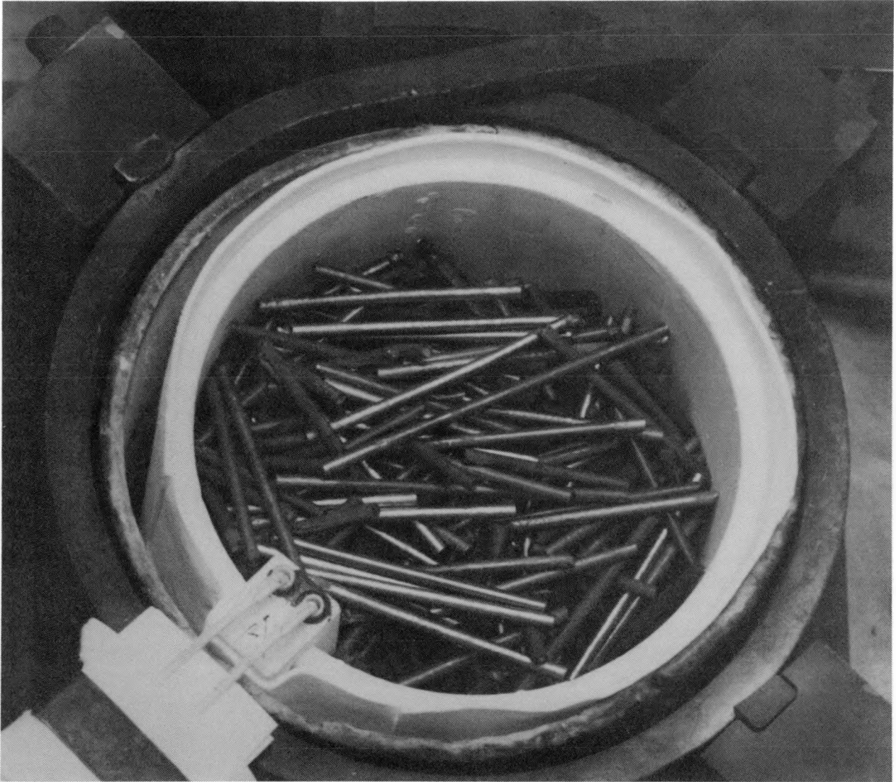
Fig. 8. Coated Crucible Loaded with Feed Material
