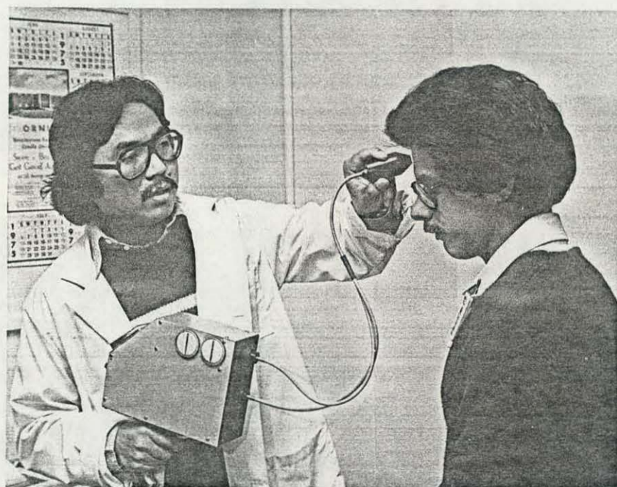
Fig.4. Fiber-optics lightpipe luminoscope for monitoring fluorescent skin contamination.
