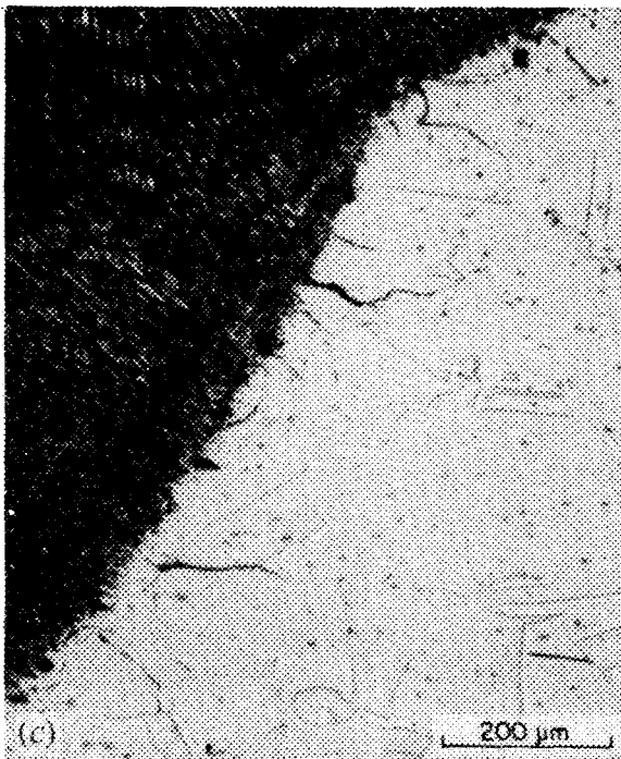
Fig. 20. Photomicrographs of typical hot cracks produced in the heat-affected zone of butt welds in 13-mm-thick plates of four HT-UPS alloys using the shielded metal arc process with 17-14CuMo stainless steel filler metal: (a) alloy AX5 with 0.024% P, (b) alloy AX6 with 0.041% P, (c) alloy AX7 with 0.076% P, and (d) alloy AX8 with 0.043% P.
