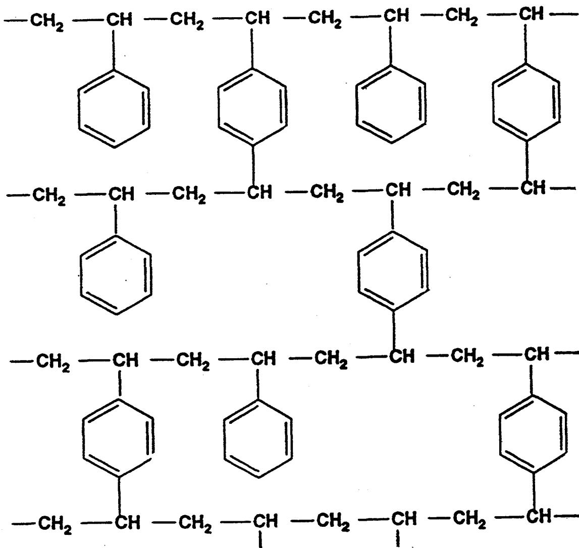
Figure 1. The chemical structure of styrene-divinylbenzene copolymer macroreticular resins such as XAD-2, XAD-4, XAD-16, Chromosorb 102 and Ostion SP-1. Adapted from US Patent 4,224,415, R.M. Patel et al., American Laboratory, Feb. 1990, and G.A. Junk, Symposium on Solid Phase Extraction, American Chemical Society, 205th Annual Meeting, San Francisco, Mar. 28-Apr. 2, 1992.
