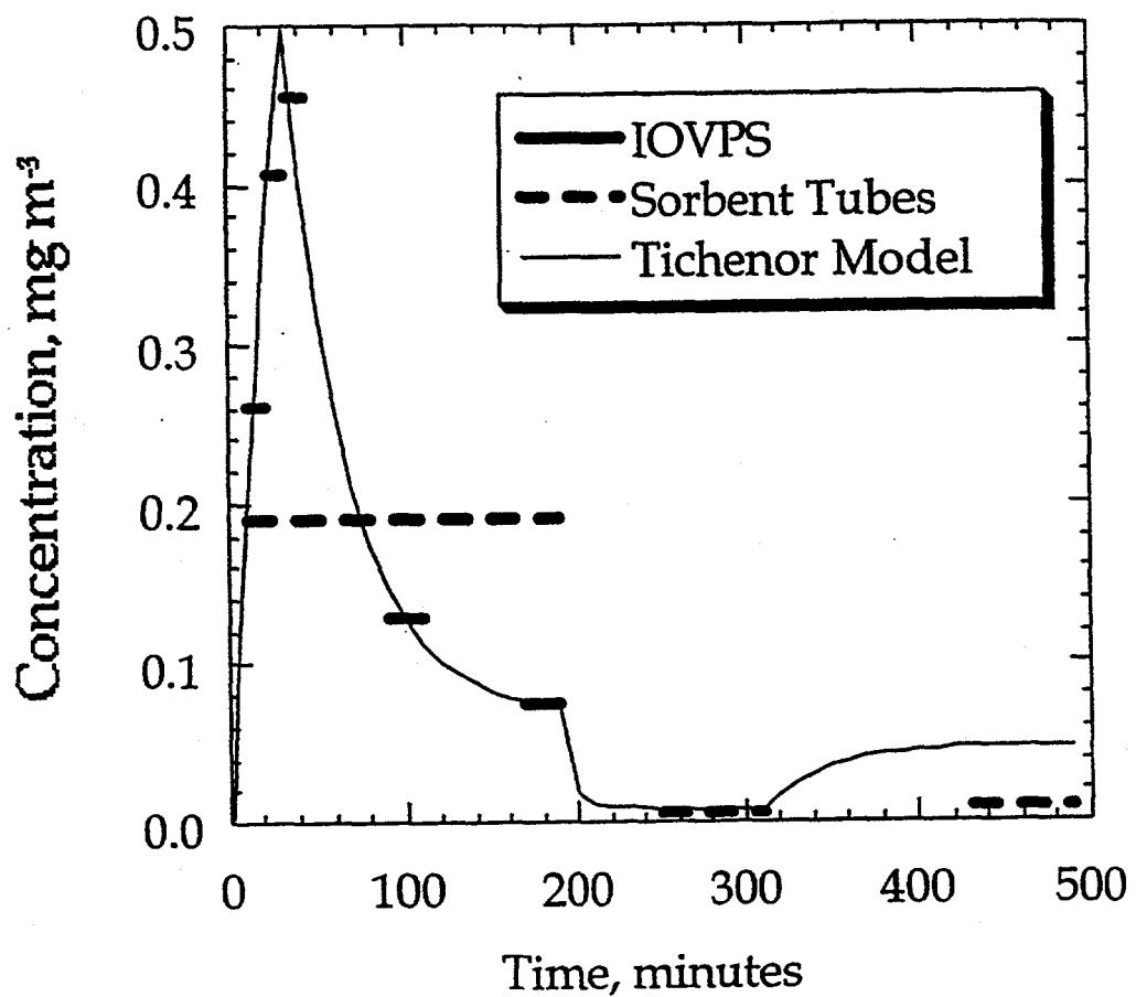
Figure 10. The concentration of gas phase nicotine as a function of time after smoking for the experiment shown in figure 9, as determined from the IOVPS and small co-located XAD-4 sorbent tubes. Just after the fifth IOVPS sample was collected, the chamber was vented for two hours, then resealed for three hours. During the last hour a final sorbent sample was collected to assess re-emission of nicotine from the walls.
