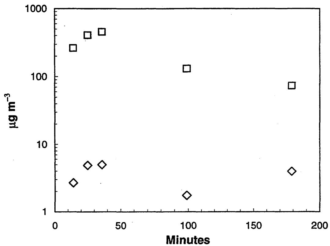
Figure 9. Gaseous (squares) and particulate (diamonds) concentrations of nicotine over a three hour period at 24° C during and after the burning of three cigarettes by machine in a sealed 20  $\text{m}^3$  chamber with stainless steel walls.
