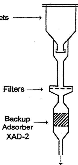
Figure 11. Schematic diagram of the hybrid Integrated Organic Gas and Particle Sampler (IOGAPS). The glass tubes of the Gas and Particle (GAP) Sampler were stripped of their tenax-silicone gum coating, sandblasted and recoated with ground XAD-4.
