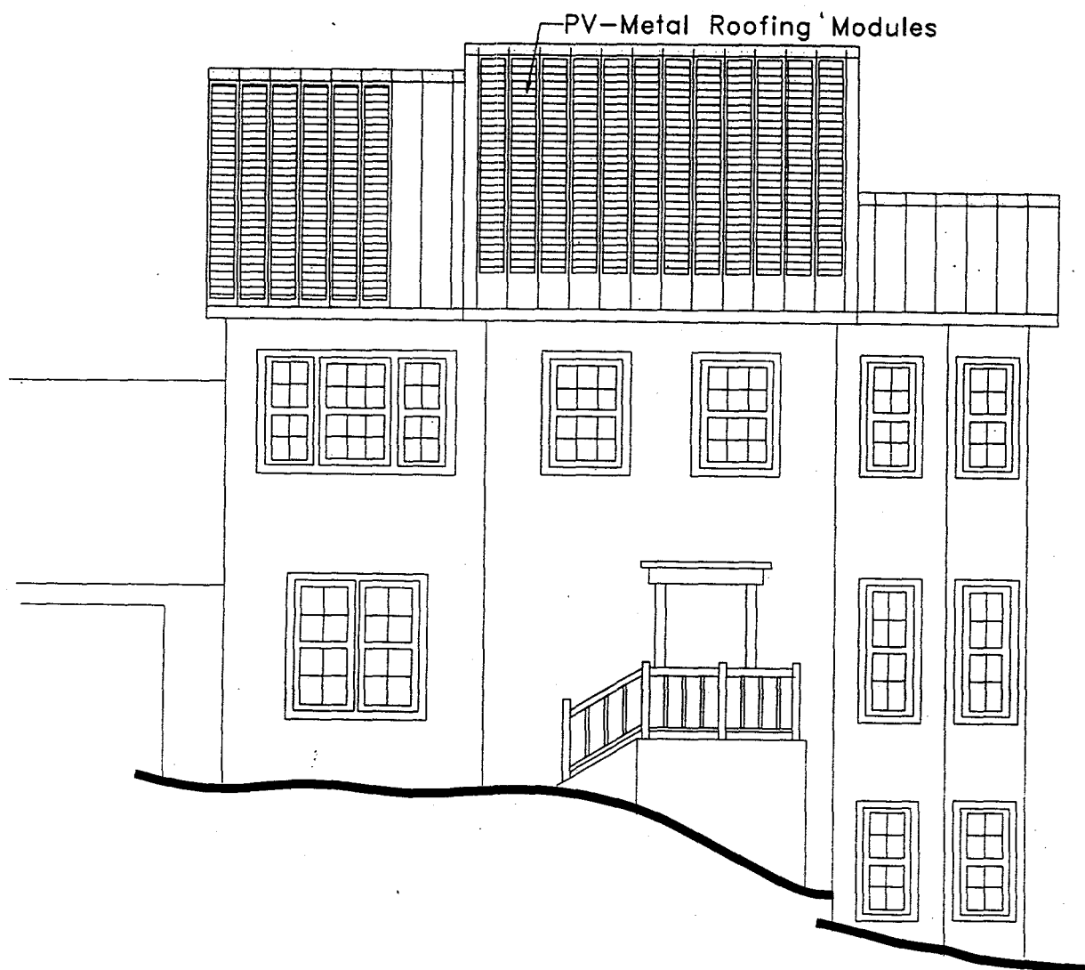
Figure 2.A.3. Design configuration of the 18 BIPV metal roofing modules on the NAHB Research Center 21st Century Townhouse.
