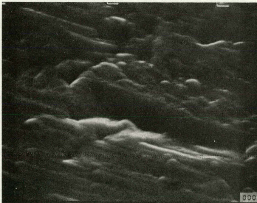
Figure 2-b. SEM micrograph of a-Si film on unpolished stainless steel (5000X).
