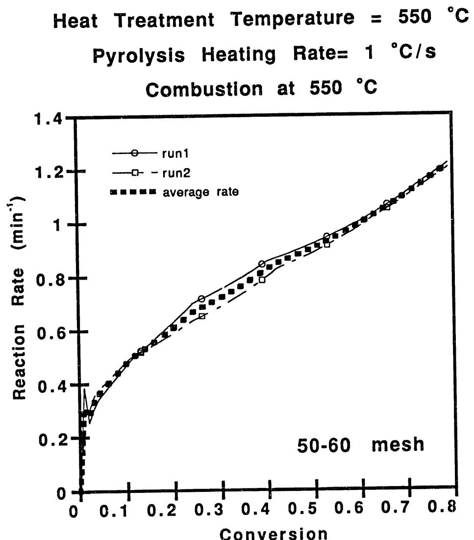
Figure 4: Reaction rates from several combustion runs (21% oxygen) with char particles from the 50-60 mesh fraction.
