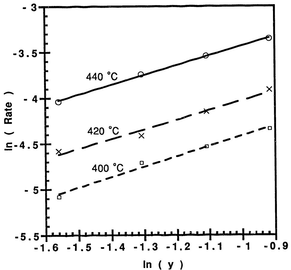
Figure 2: Reaction rates vs. oxygen concentrations at various combustion temperatures.
