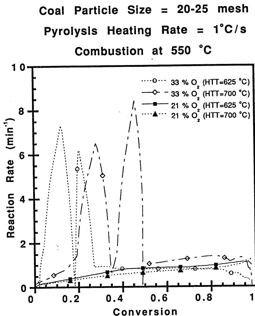
Figure 9: The effect of oxygen concentration on the reactivity rates of char particles from the 20-25 mesh fraction. Note the particle ignitions shown as sharp peaks in reactivity.
