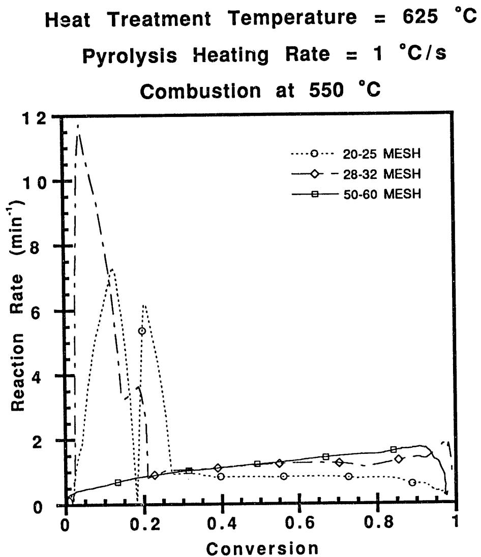
Figure 8: The effect of particle size on the reactivity and ignition patterns of Illinois #6 char particles.
