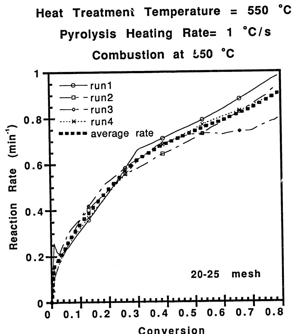
Figure 6: Reaction rates for several combustion runs (21% oxygen) with char particles from the 20-25 mesh fraction.
