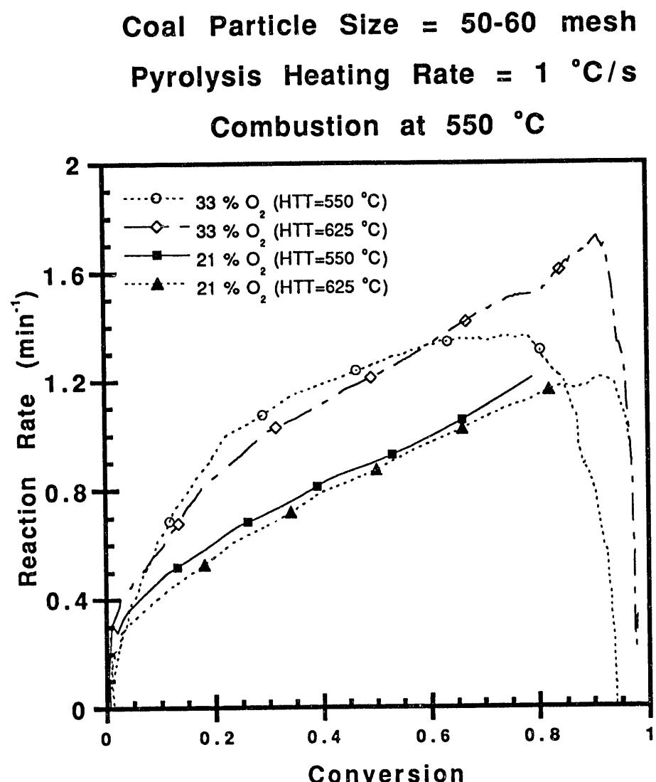
Figure 10: The effect of oxygen concentration on the reactivity rates of char particles that do not exhibit ignitions.
