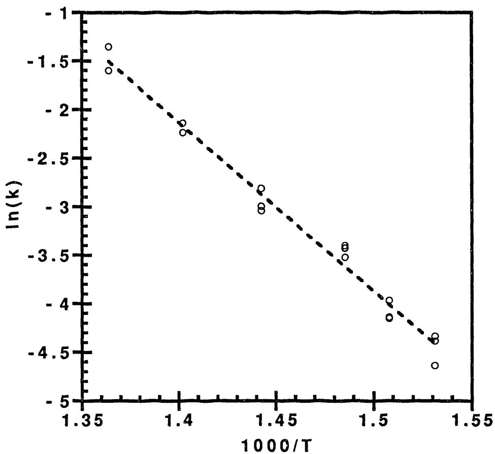
Figure 3: Arrhenius plot of the reaction rate constant for combustion of Illinois #6 chars
