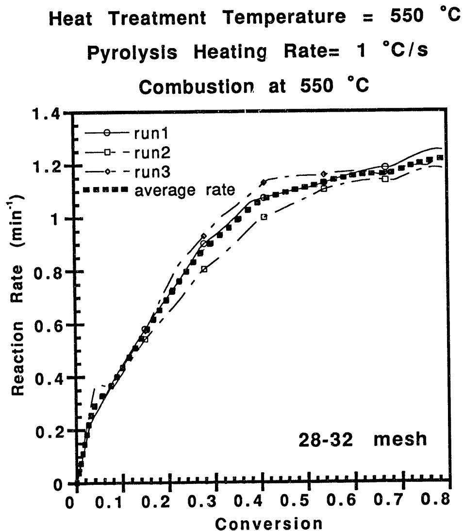
Figure 5: Reaction rates for several combustion runs (21% oxygen) with char particles from the 28-32 size fraction.
