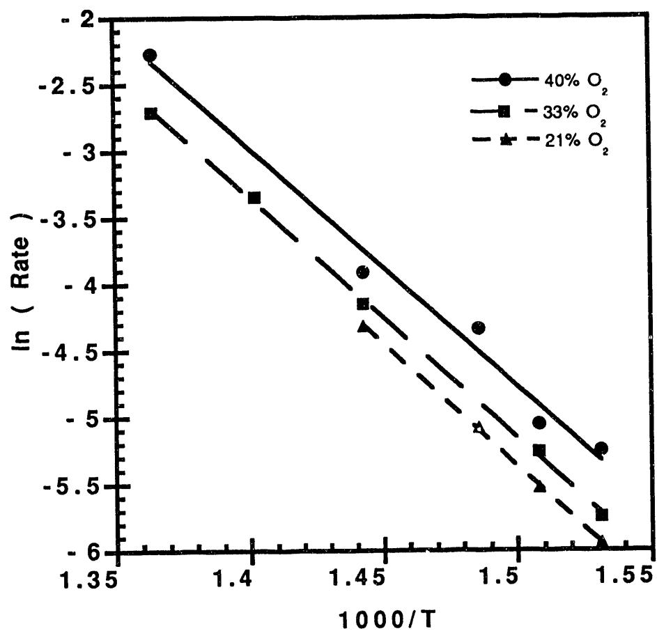
Figure 1: Arrhenius plots for the average combustion rates of Illinois #6 chars at various oxygen concentrations. Reference conversion for calculating the average reaction rates is 0.25.
