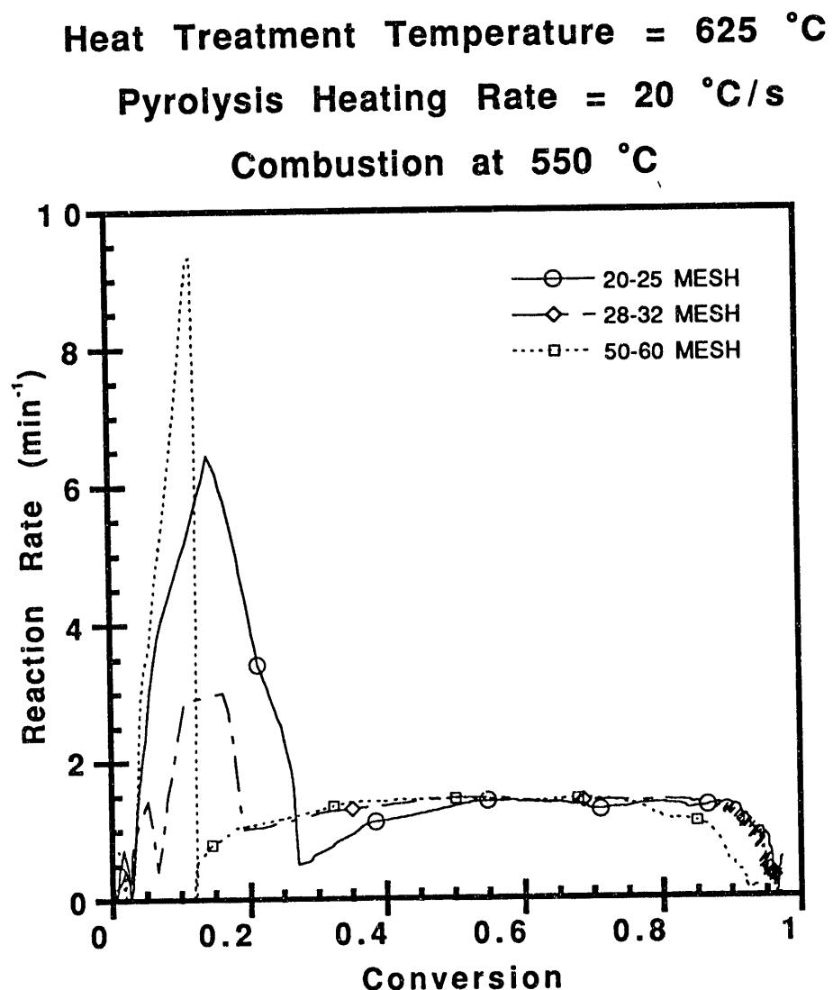
Figure 7: The effect of particle size on the reactivity and ignition patterns of Illinois #6 chars reacted with 33% oxygen.
