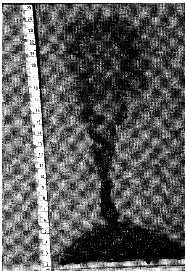
Figure 1. After flowing through sand under the influence of a magnetic field, ferrofluid accumulates symmetrically next to the magnet.
