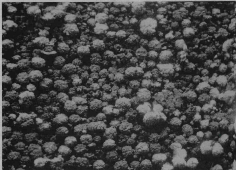
FIGURE 16. " ^{240}\text{PuO}_2 Simulant" Rosettes, as Received
