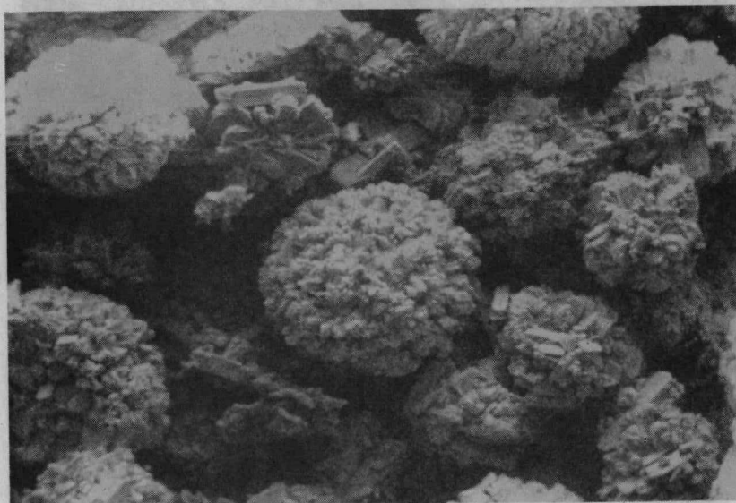
FIGURE 12. Pu(III) Direct-Strike Rosettes (15°C) (All Addition and Digestion Times Reduced One-Half)
