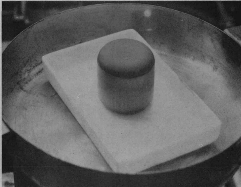
FIGURE 19. DF Pellet 2 After Final Heat Treatment
