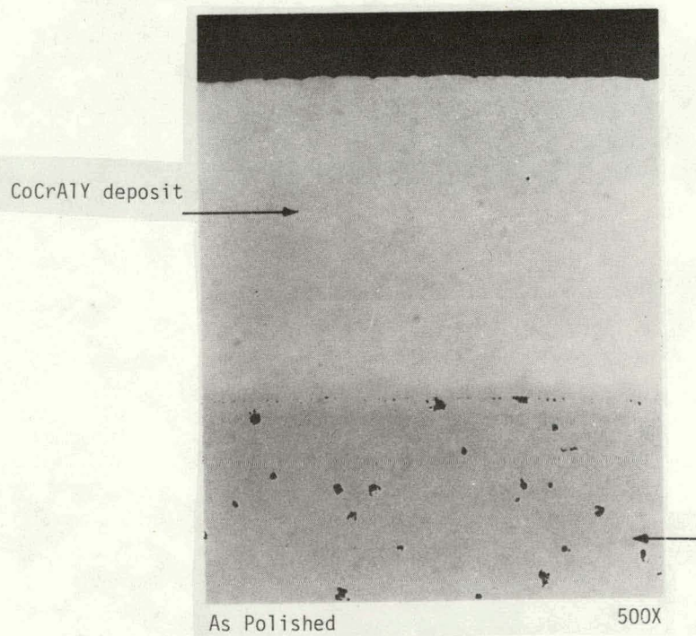
Figure 12 Run #30 Sample # 5035B CoCrAlY sputter deposited on a 1/8" dia. MAR-M-509 pin. Vacuum heat treated 4 hrs at 1080°C.
