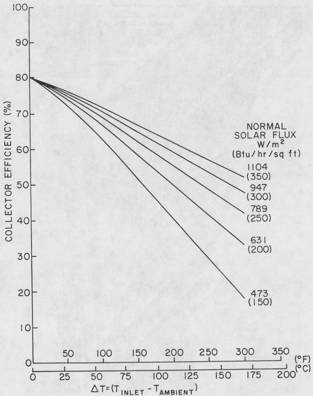
Figure 2.2.2. Collector Simulator Test Performance
