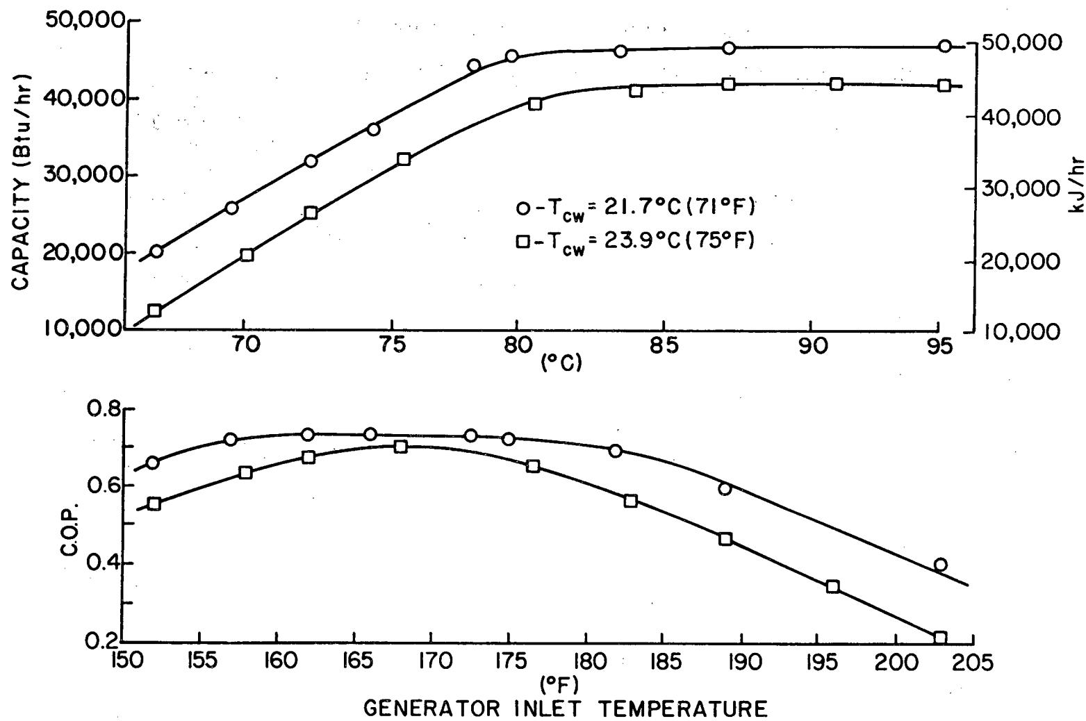
Figure 2.3.3. Modified Charge Arkla Chiller Performance Characteristics
