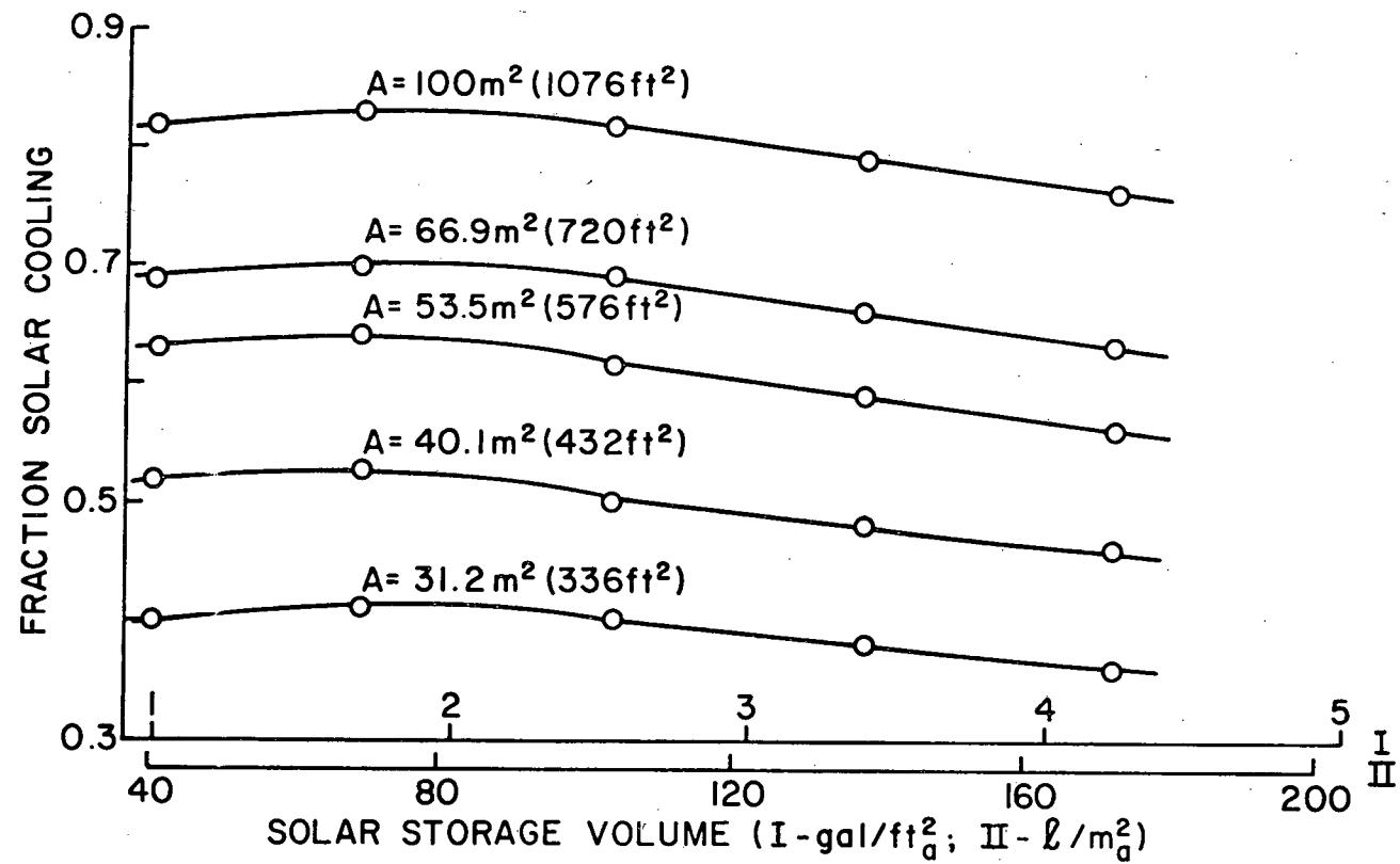
Figure 3.5.2. Solar Storage Volume Effects -- Washington, D.C. System
