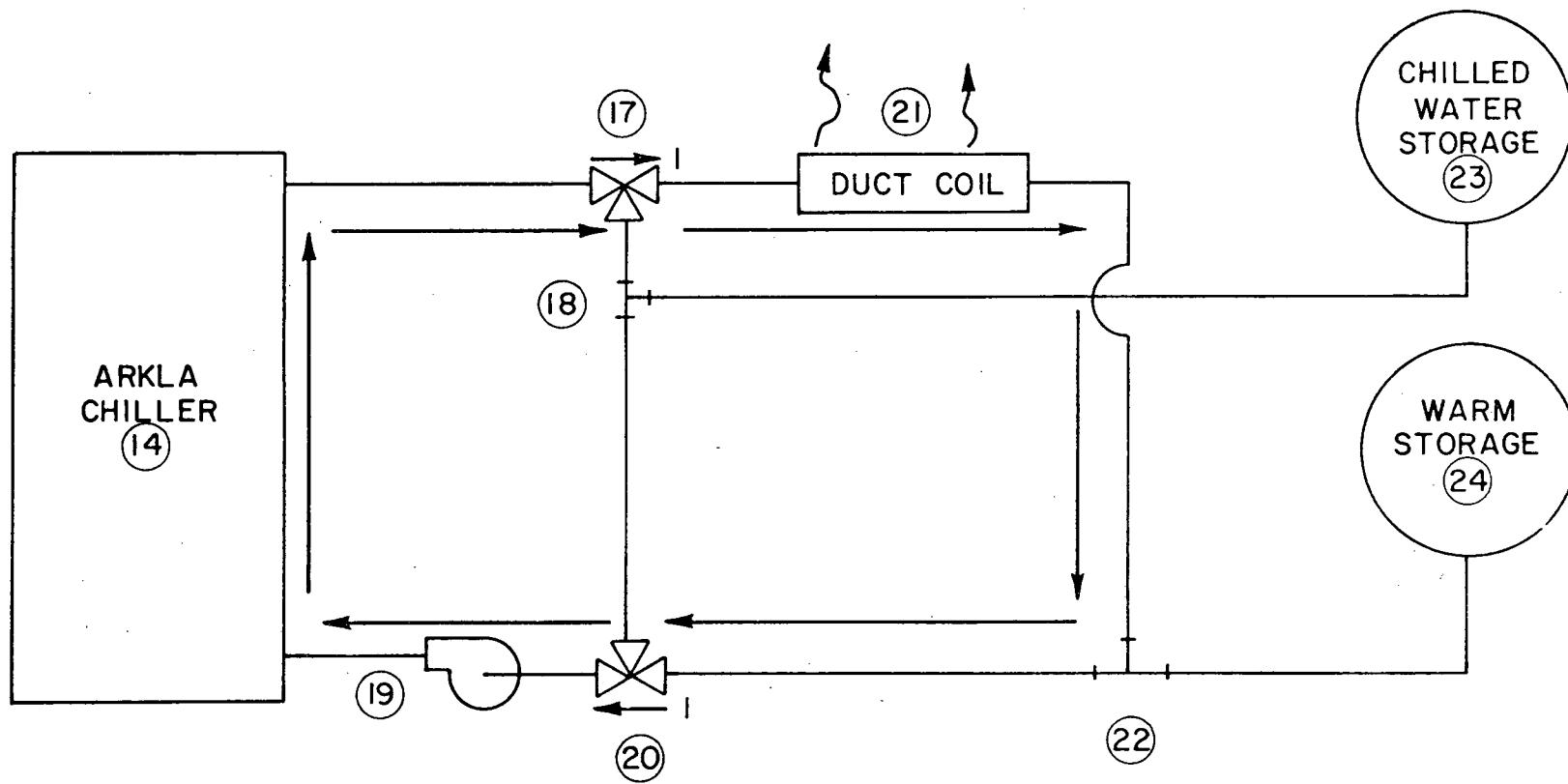
Figure 2.1.6. Chilled Water Storage Operational Modes,
