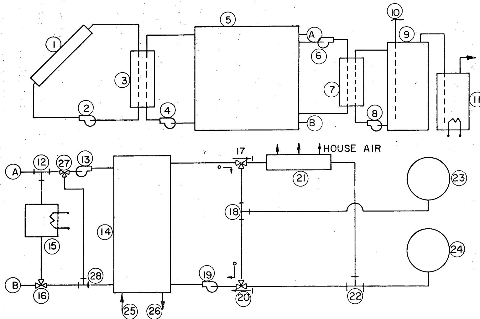
Figure 2.1.1. Solar Cooling System with Chilled Water Storage
