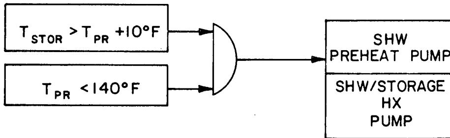
Service Hot Water Preheat System Control Logic
