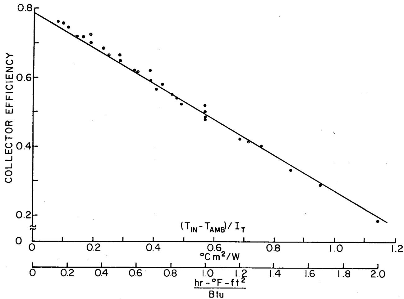
Figure 2.2.3. Normalized Collector Simulator Test Performance
