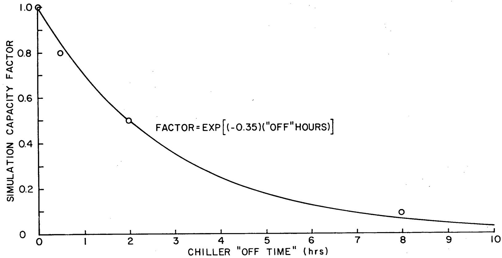
Figure 2.3.4. Chilled Transient Response Characteristics
