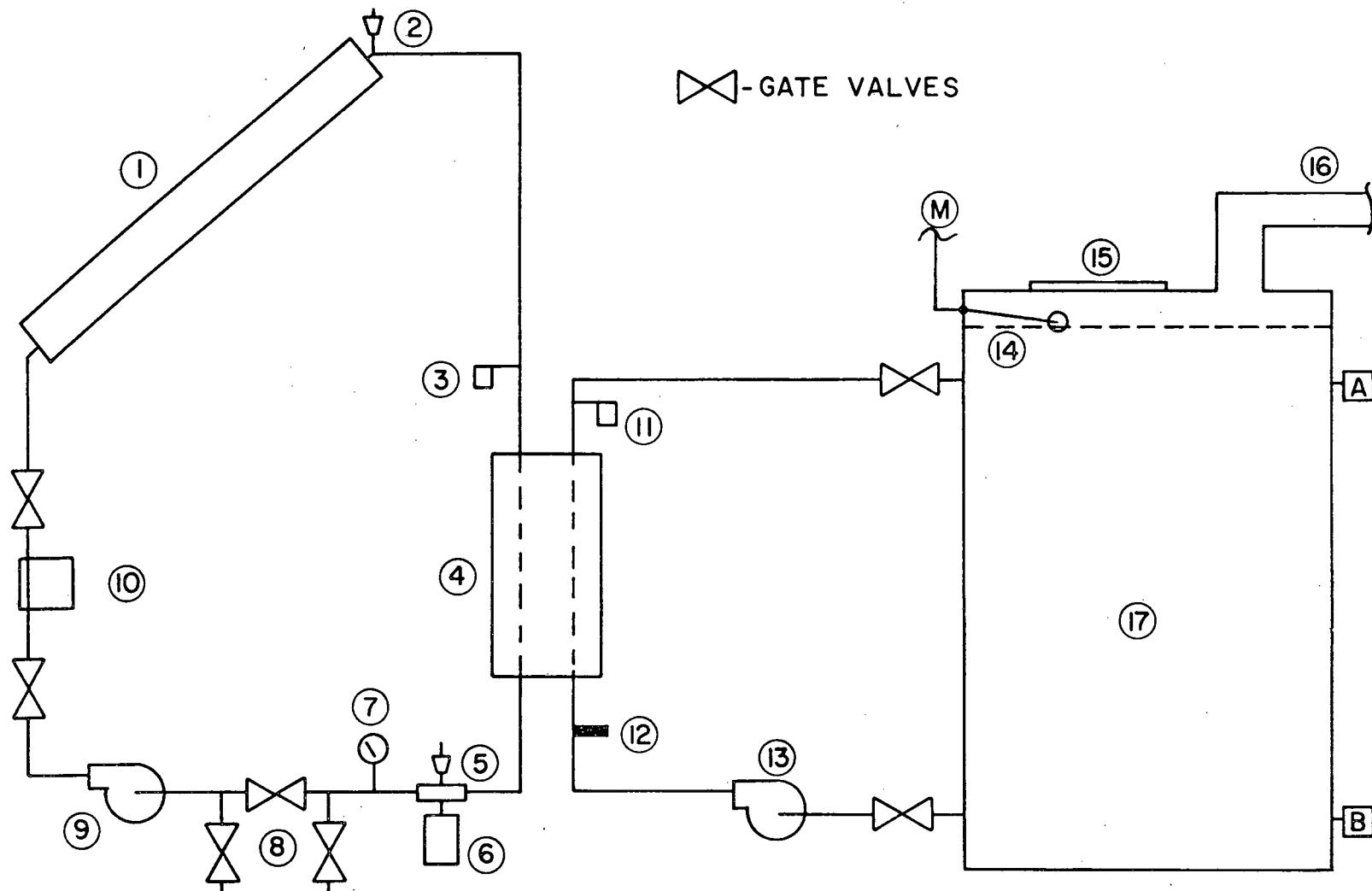
Figure 4.6.1. Recommended Design Schematics of a Residential Solar Operating Air Conditioning System, Collector/Storage System
