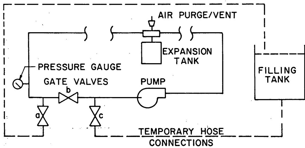
Figure 4.6.4. Closed Hydronic System Fill/Drain
