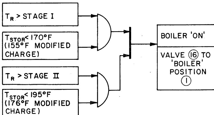
Figure 2.1.4. Auxiliary Boiler Control Logic
