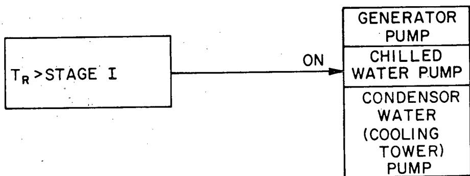
Figure 2.1.5. Chiller Control Logic
