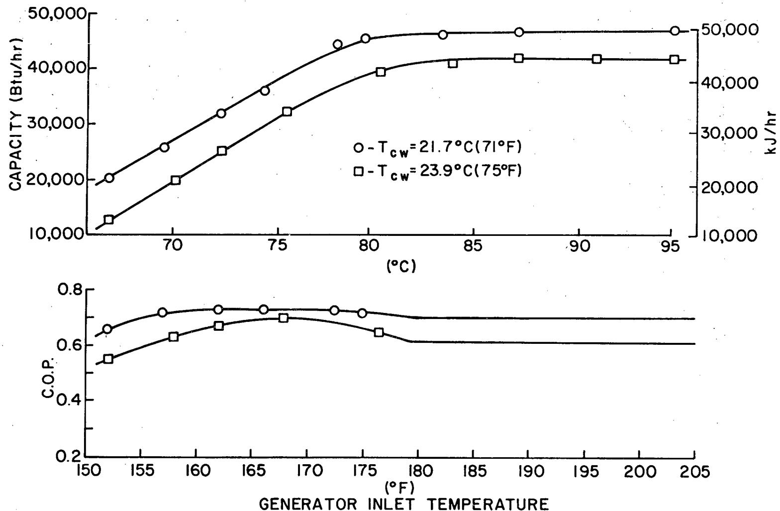
Figure 2.6.1. Performance Characteristics of Modified Charge Arkla Chiller with Tempering Valve
