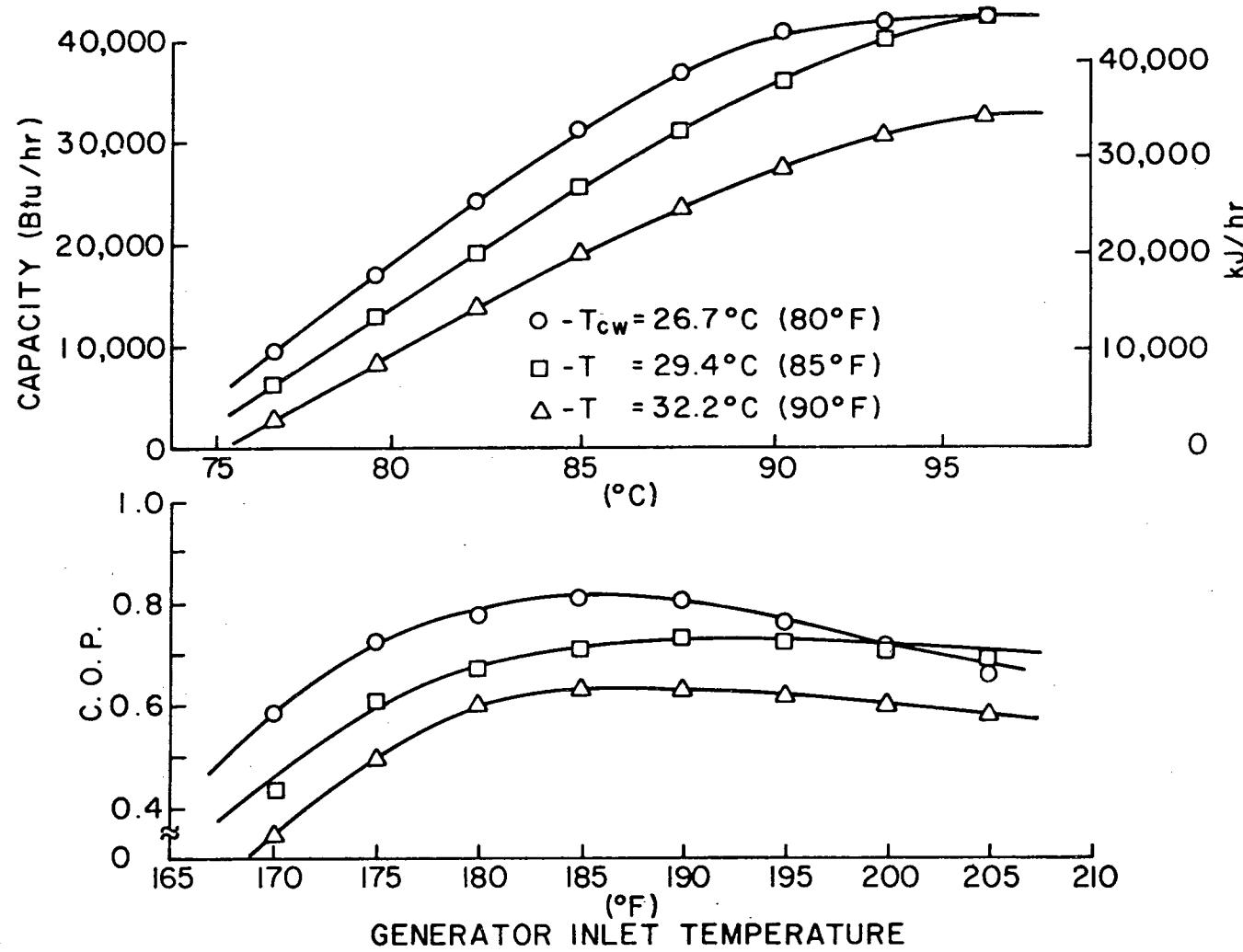
Figure 2.3.2. Standard Arkla Chiller Performance Characteristics
