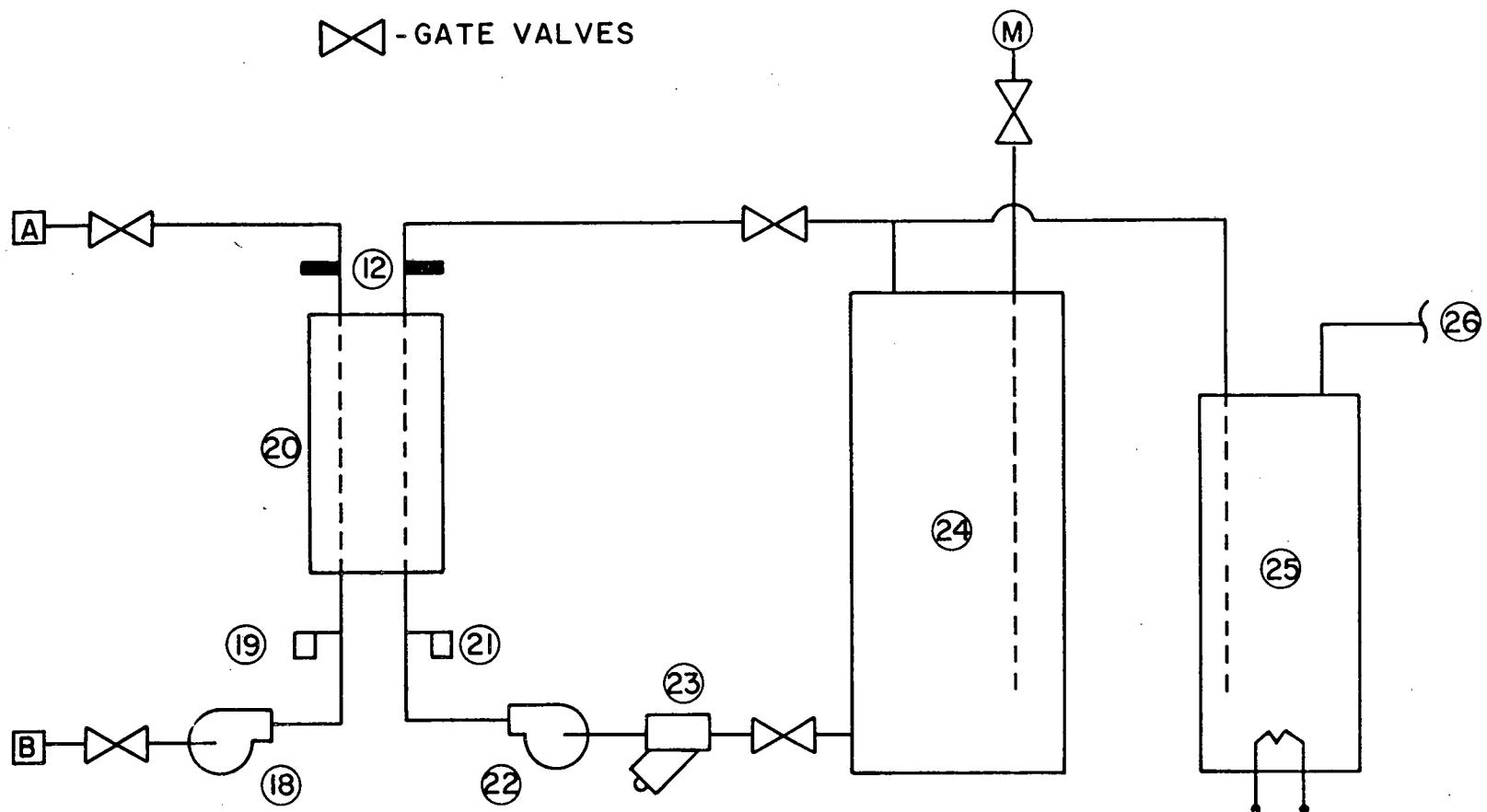
Figure 4.6.2. Recommended Design Schematics of a Residential Solar Operated Air Conditioning System, Service Hot Water Preheat System
