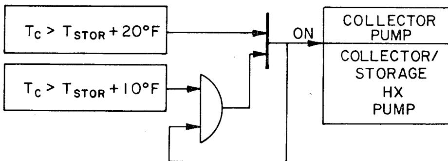
Figure 2.1.2 Collector/Storage Control Logic
