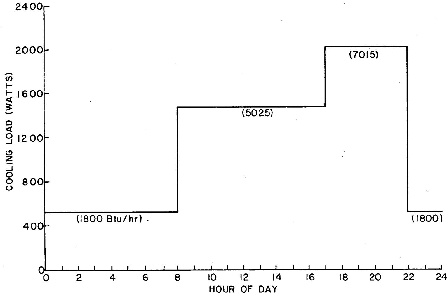
Figure 2.5.1. Building Cooling Load: Internal Heat Generation
