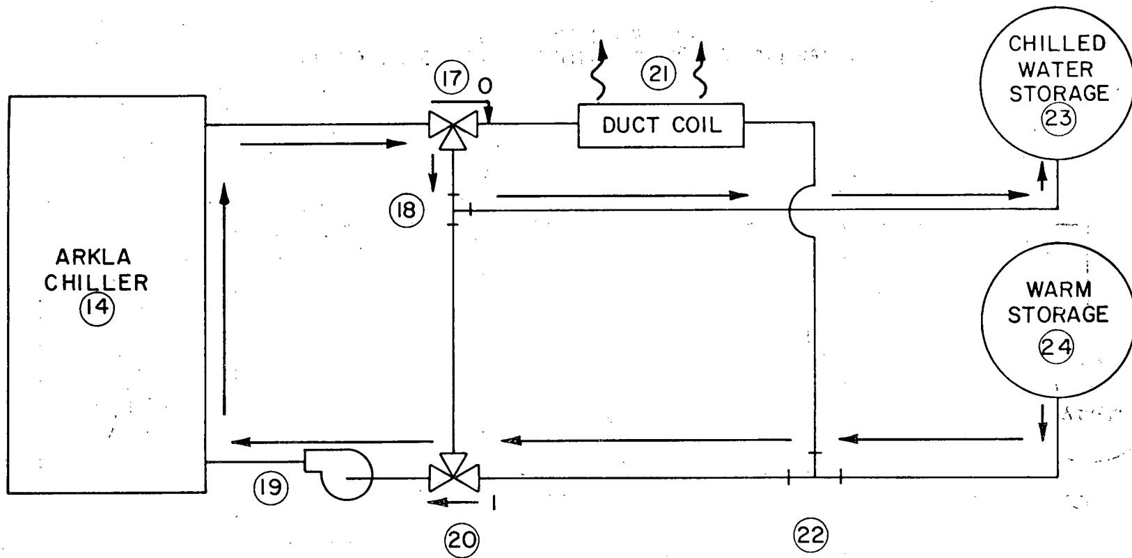
figure 2.1.7. Chilled Water Storage Operational Modes,
