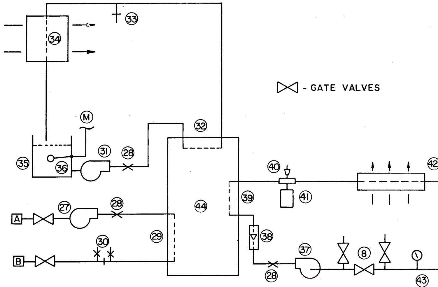
Figure 4.6.3. Recommended Design Schematics of a Residential Solar Operated Air Conditioning System, Absorption Chiller System
