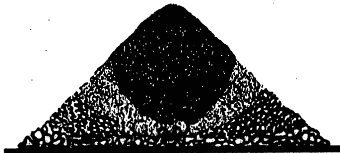
Segregation of Different Sizes of Coal in Conical Pile.
