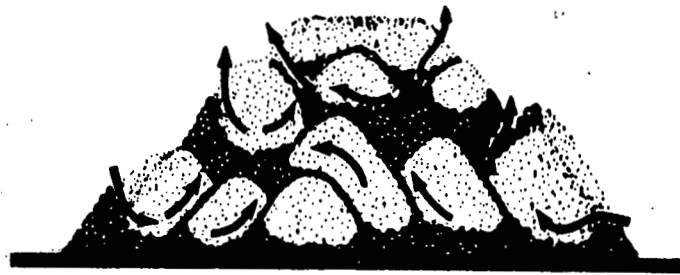
Haphazard Stacking, Showing Air Circulation
