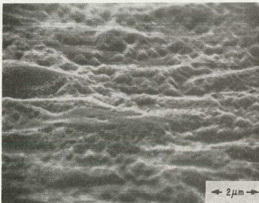
Figure 42. SEMs of n + -silicon surface after dissolution of Ag and glass film. Film contained 15 vol pct lead borosilicate glass and was fired for 2 min at 800°C.
