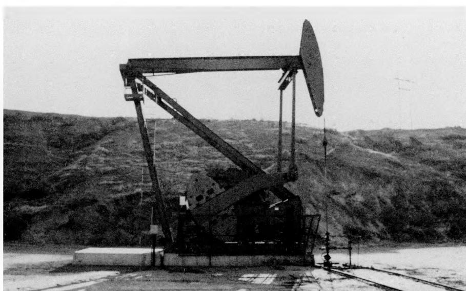
*Optimization of oil well artificial lift units, as shown in this photograph, is maintained at Naval Petroleum Reserves in California by timed pump-off controllers.*
