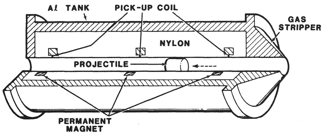
Figure 2. Cutaway View of MAVIS
