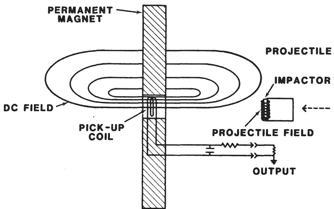
**Figure 3.** MAVIS Circuitry and Magnetic Fields
