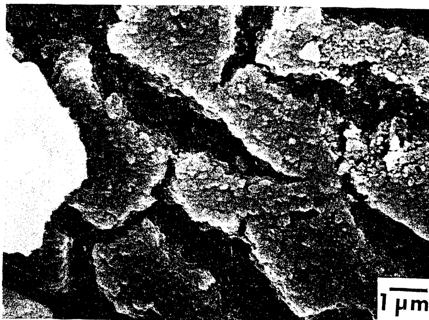
Figure 3.14a SEM micrograph of a thick area in a single layer LSC film spin-coated onto a 0.02 micron pore size Anotec filter and fired at 800°C. Shrinkage cracking and exposure of the underlying filter surface have occurred.
