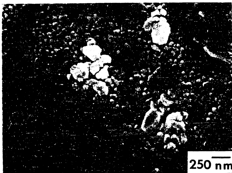
Figure 3.19a SEM micrograph of a four layer LSC film dip-coated onto a 0.02 micron pore size Anotec filter and fired at 700°C. Shrinkage cracking and inhomogeneous precipitation are present.
