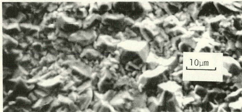
Figure 11. SEM Photographs of Surfaces of GaAs Films Deposited by MO-CVD at 650°C onto Etched Surfaces of Mo Sheet Substrates. a) No HCl Present (film 35 \mu m thick); b) HCl Flow Rate 5 ccpm (film 29 \mu m thick); c) HCl Flow Rate 10 ccpm (film 45 \mu m thick).
