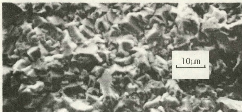
Figure 12. SEM Photographs of Surfaces of GaAs Films Deposited by MO-CVD at 675°C onto Etched Surfaces of Mo Sheet Substrates. a) No HCl Present (film 26 \mu m thick); b) HCl Flow Rate 5 ccpm (film 29 \mu m thick); c) HCl Flow Rate 10 ccpm (film 33 \mu m thick).
