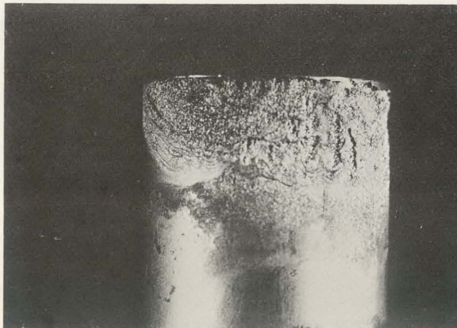
Figure 18. O.D. surface of AL-6X control specimen (no cleaning) after a 7-month exposure, showing severe crevice corrosion under flexible connector. 2.5X Magnification. Neg. No. S-1852
