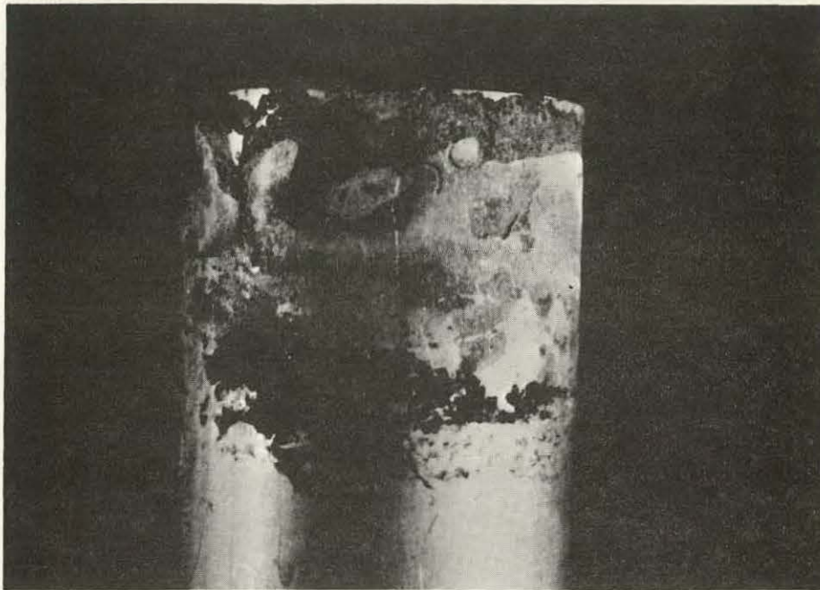
Figure 13. O.D. surface of 5052 aluminum control specimen (no cleaning) after a 7-month exposure, showing crevice corrosion under flexible connector. 2.4X Magnification. Neg. No. S-1844
