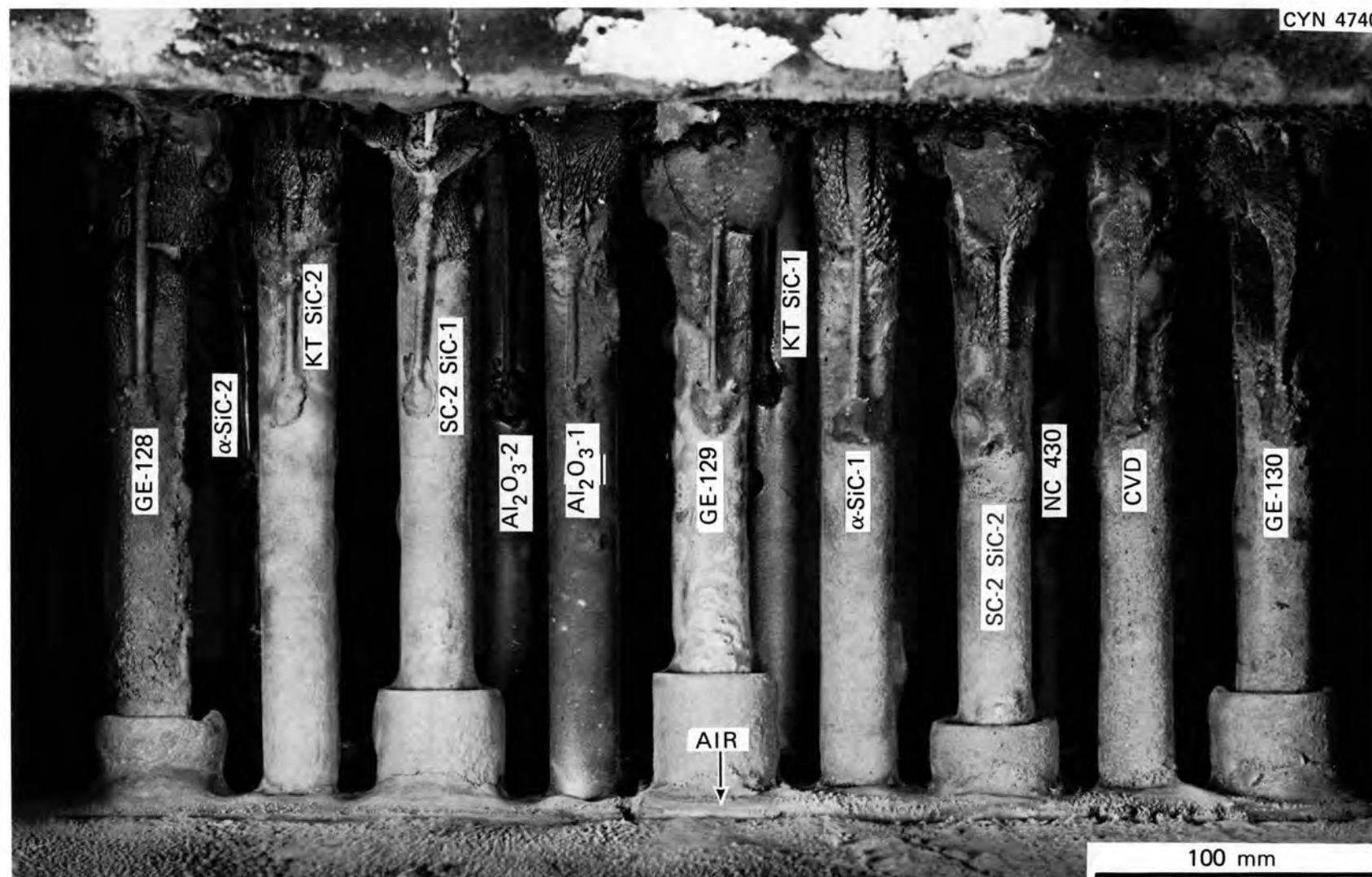
Fig. 15. Post-test tube array illustrating condition of downstream surfaces of ceramic tubes after long-term exposure.
