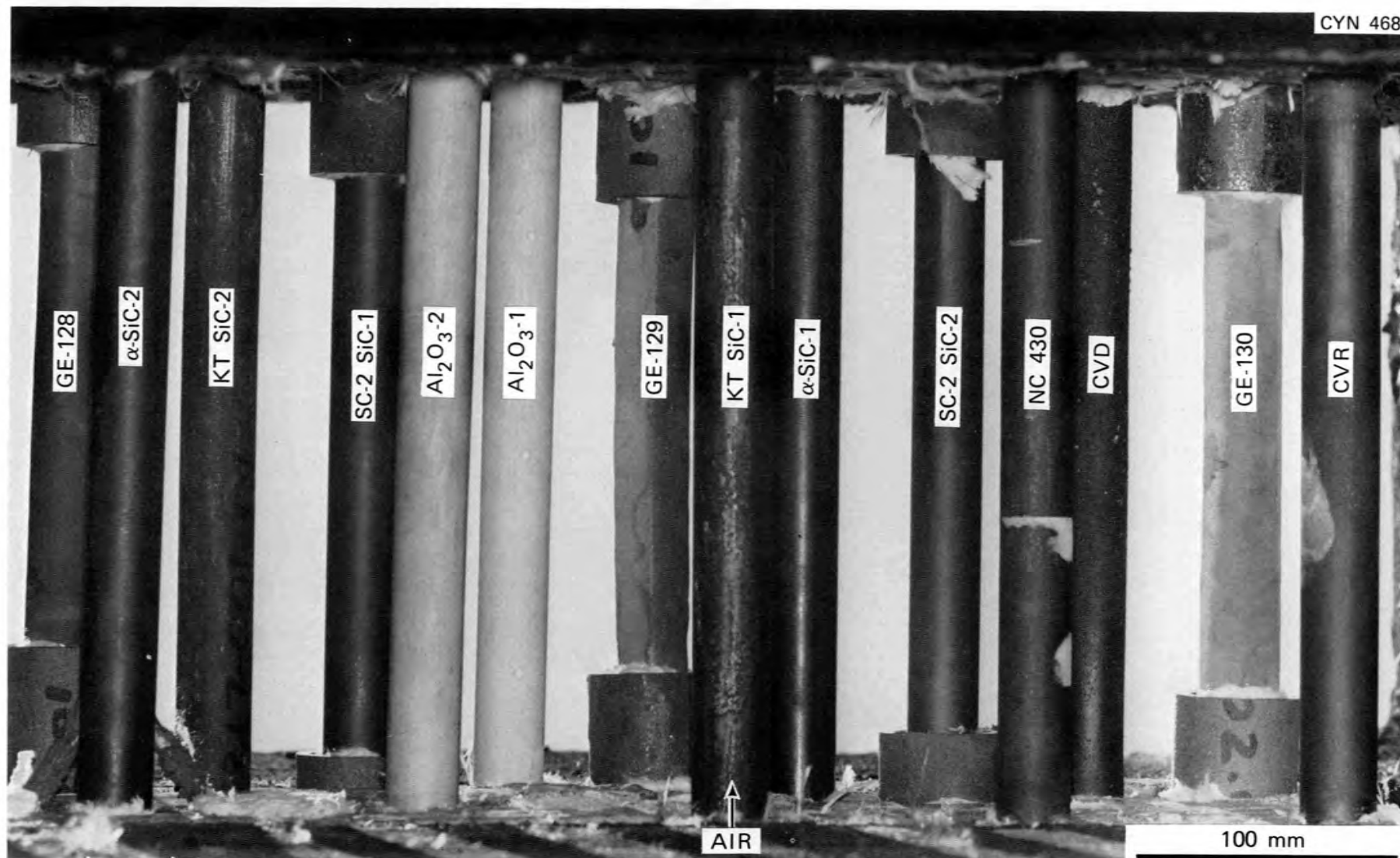
Fig. 5. Upstream surface of pretest ceramic tubes mounted in flue gas duct on the Refractory Test Facility. Flue gas flow direction into the page.
