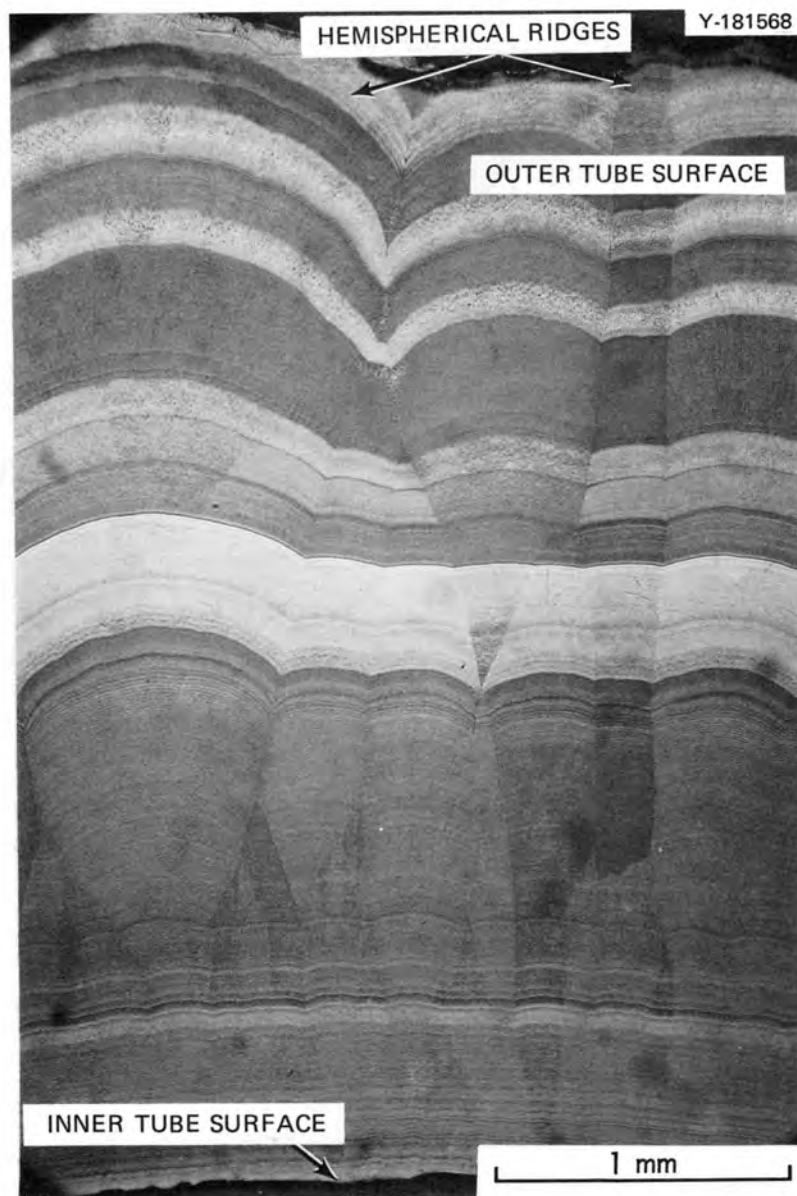
Fig. 25. Micrograph of as-received CVD SiC illustrating lack of uniformity along outer surface.
