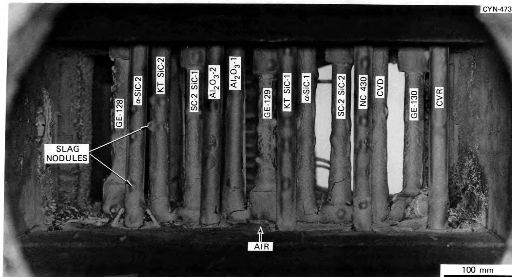
Fig. 14. Post-test tube array illustrating residual slag nodules on upstream surfaces of ceramic tubes after long-term exposure.
