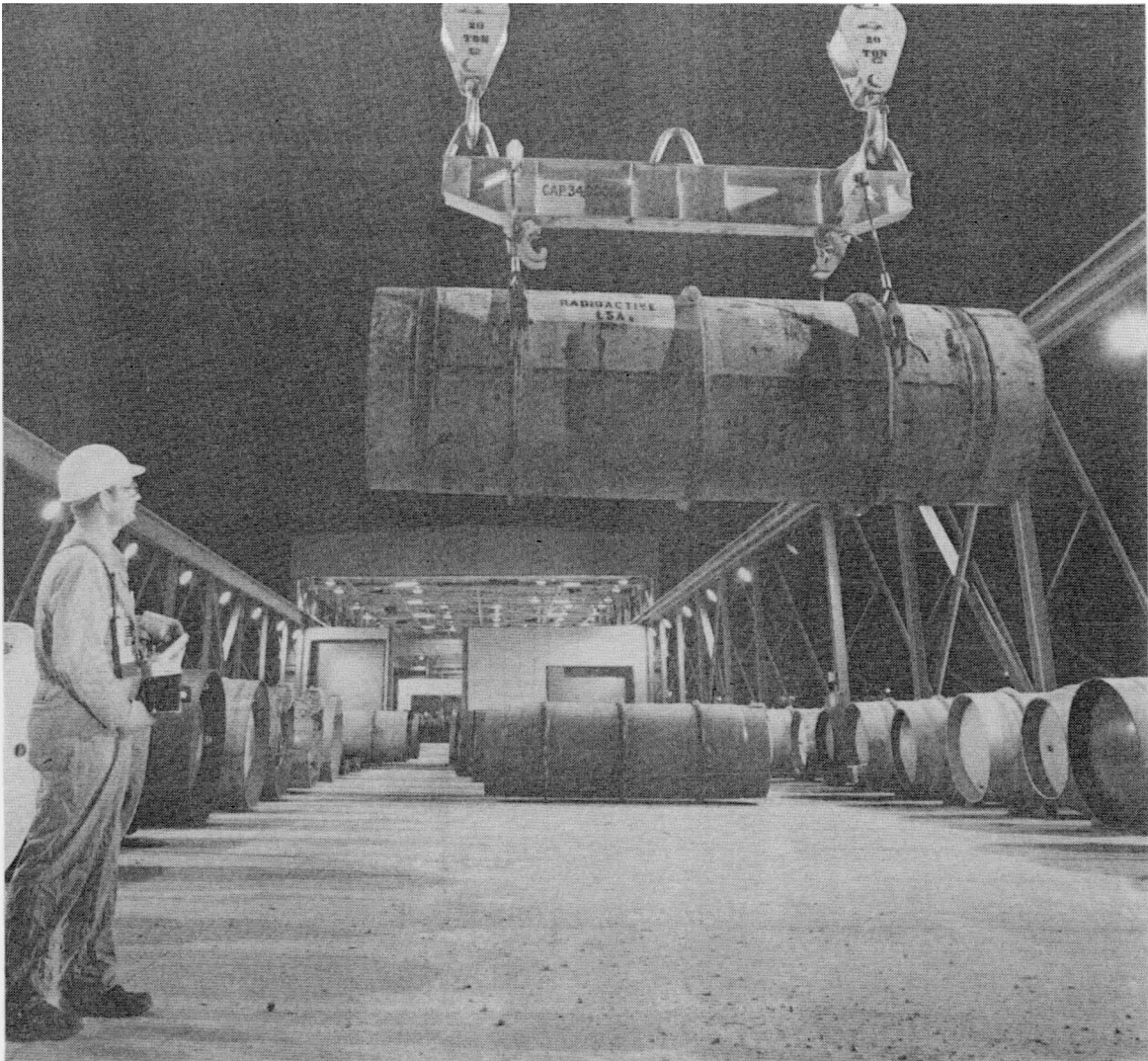
Fig. 31. Overhead double-hook crane moving a 14-ton cylinder.
