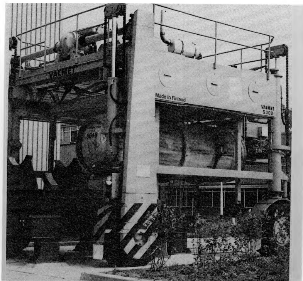
Fig. 30. Urenco on-site feed cylinder transporter.
