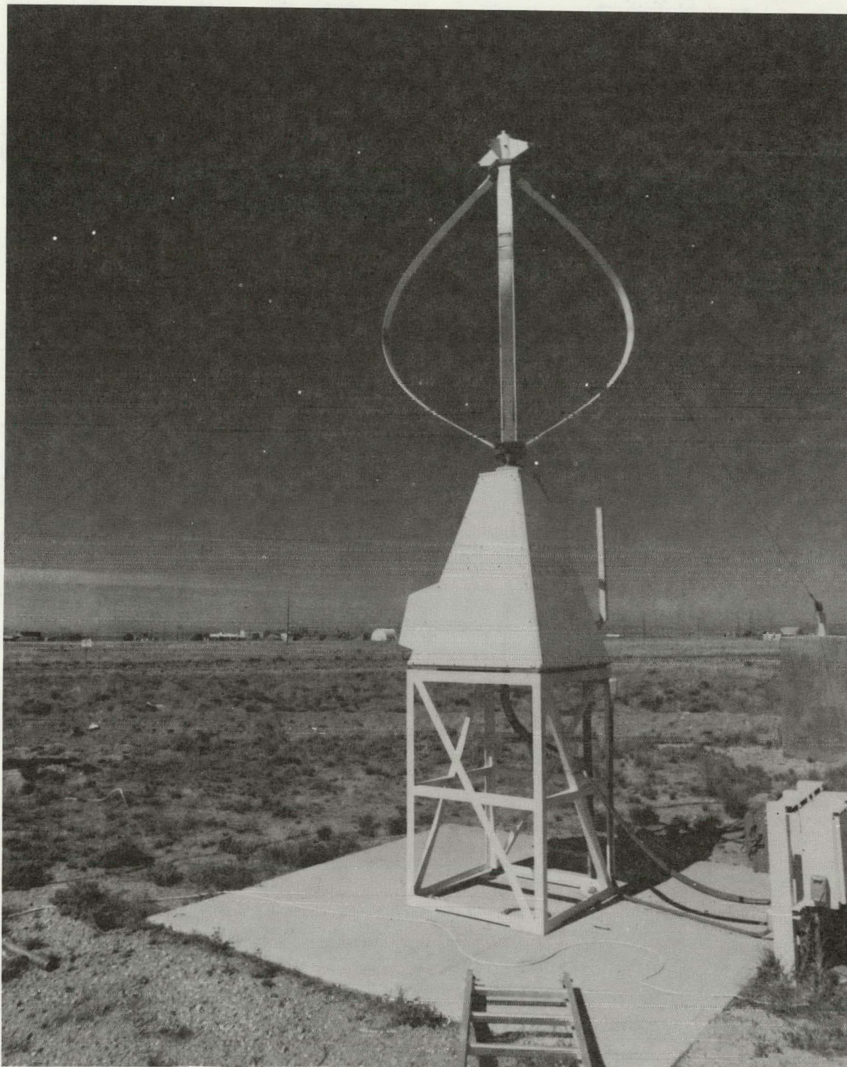
This Sandia National Laboratories experimental 2 meter Darrieus wind turbine serves as an aerodynamic blade flutter research test unit, and a wind tunnel model to demonstrate equivalence and credibility to data collected during field tests. This lift-driven airfoil test bed is so designed that the mechanical arrangement is less compact than an operational unit, thus giving more experimental flexibility.
