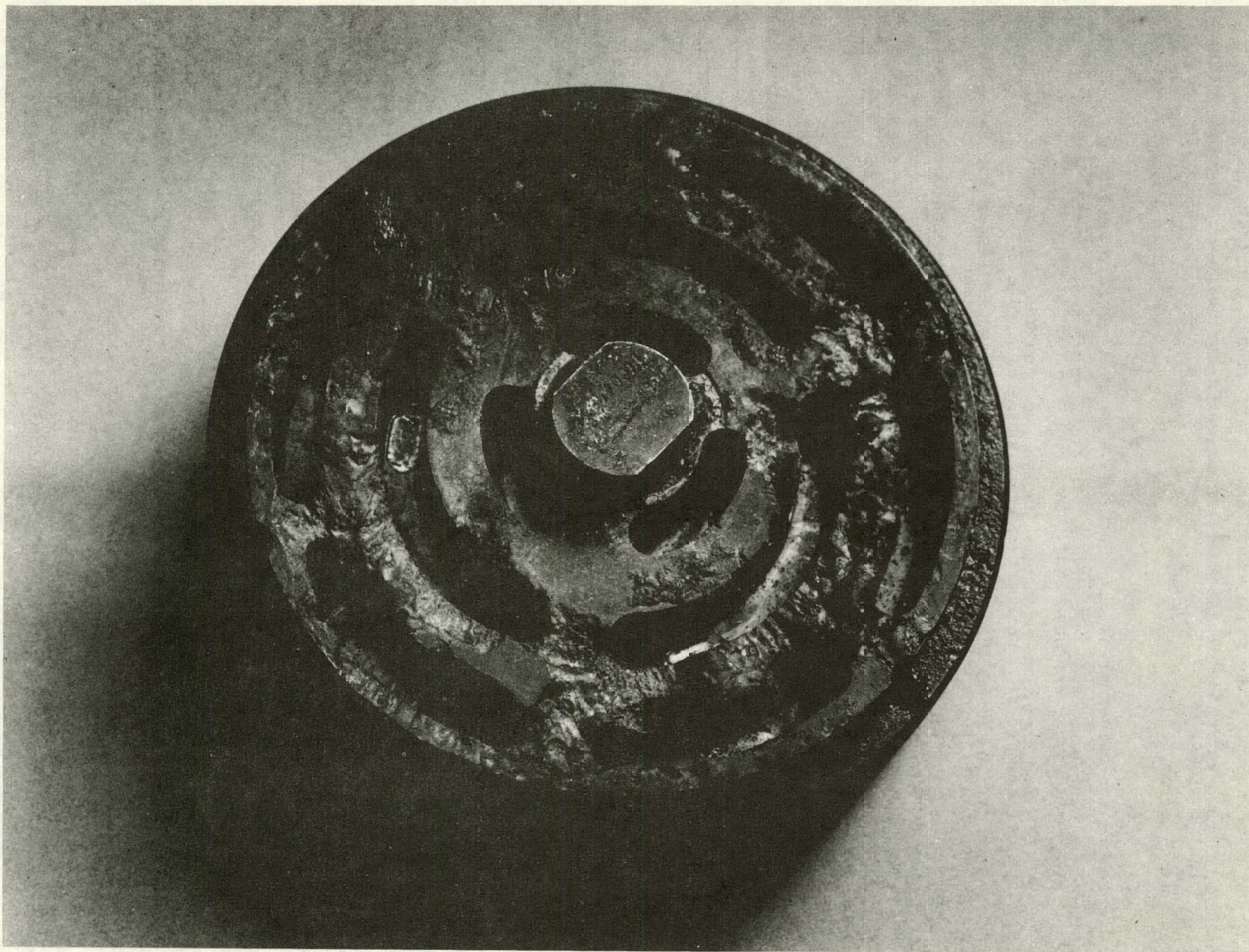
Figure 8: Corroded suction valve seat from second-stage compressor
