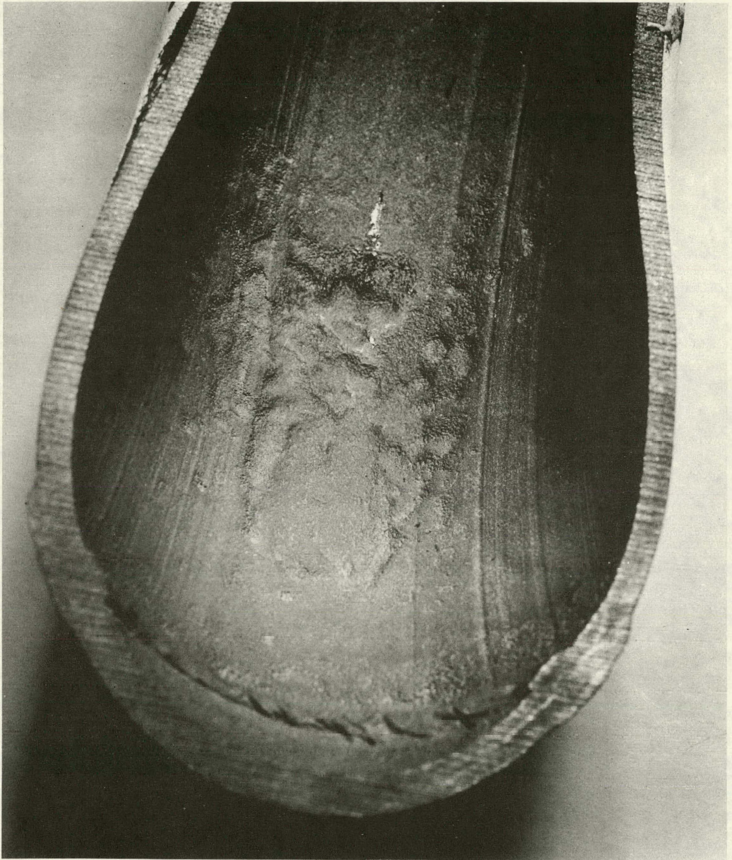
Figure 16: Corroded 4"-diameter pipe elbow from first-stage piping
