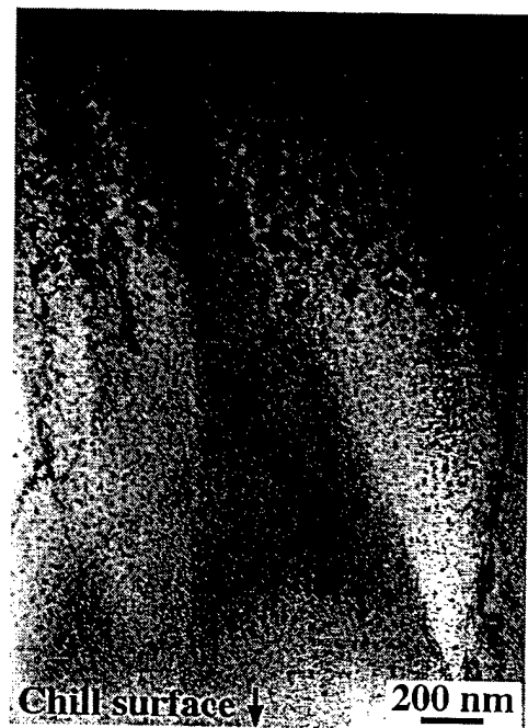
Figure 4. TEM of the chill-side of the melt-spun ribbon. The Laves phase particles become more abundant and larger towards the air-side.
