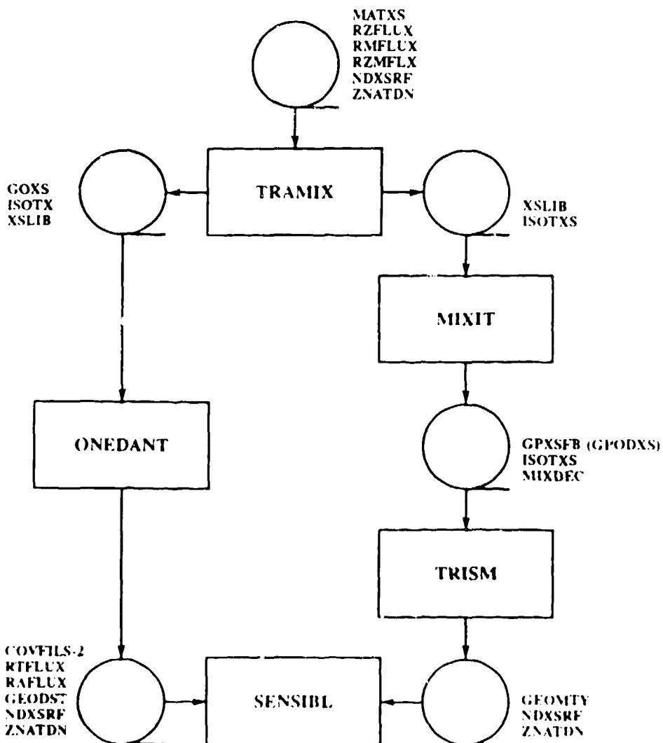
Figure 2. Flow Diagram of the AARE Cross-Section Sensitivity and Uncertainty Path
