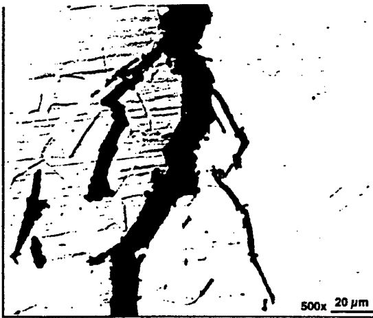
Fig. 5. Typical cracks observed in 304L SS cladding.
