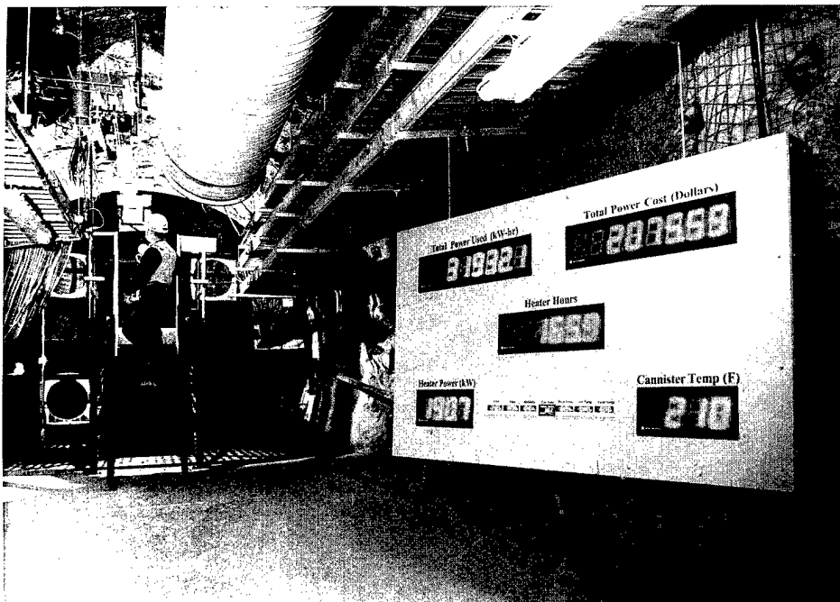
A data display board shows the total power used, the total power cost, heater hours and a representative canister temperature in the heated drift. The Drift-Scale Test is heating a tunnel segment to temperatures of up to 200 degrees Celsius (392 degrees Fahrenheit), simulating the temperatures expected in a geologic repository.
