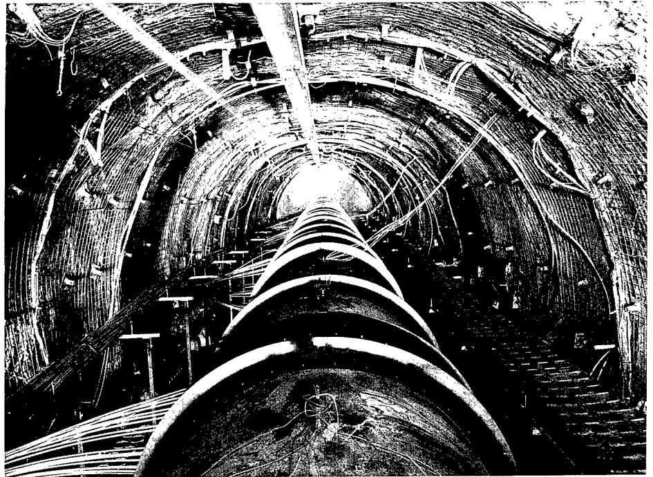
Canisters are used to simulate repository emplacement containers in the Drift-Scale Test. There are 30 electric heaters within each canister. This test will span 8 years.
