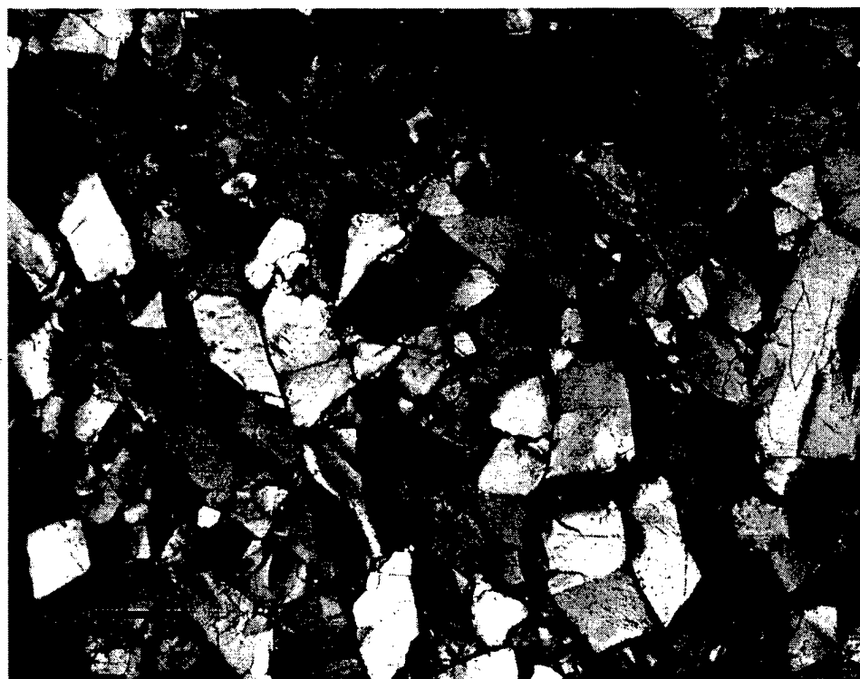
Figure 15. X-0535 Pressed to 4% Porosity (med. res.)
