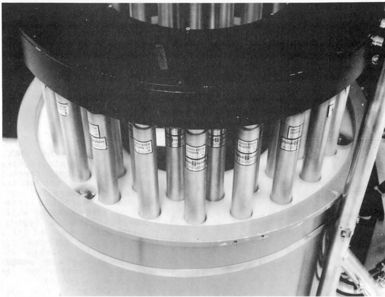
Fig. 19. Photograph of the ^3\text{He} detector ring in the AWCC. The detector ring has been partially removed from the polyethylene shielding in which it is housed so it would be more easily seen in the picture.
