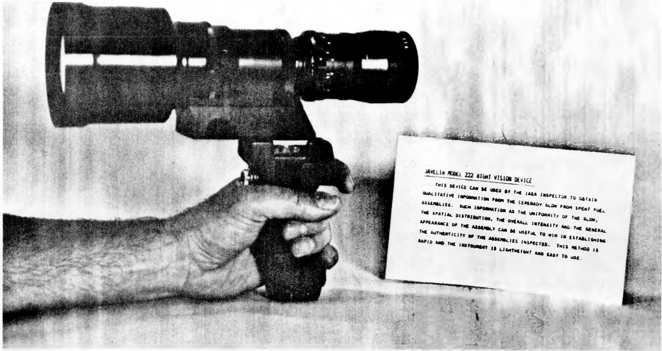
Fig. 16. Hand-held night-vision camera for observing the Cerenkov glow from spent fuel.
