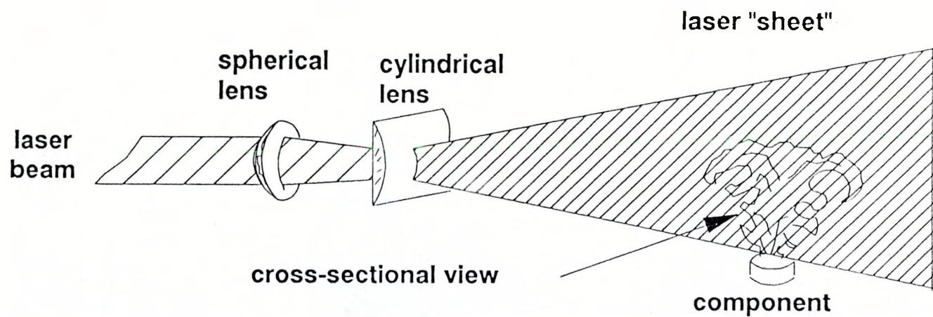
The igniters were filmed using sheet lighting from the copper vapor laser.
