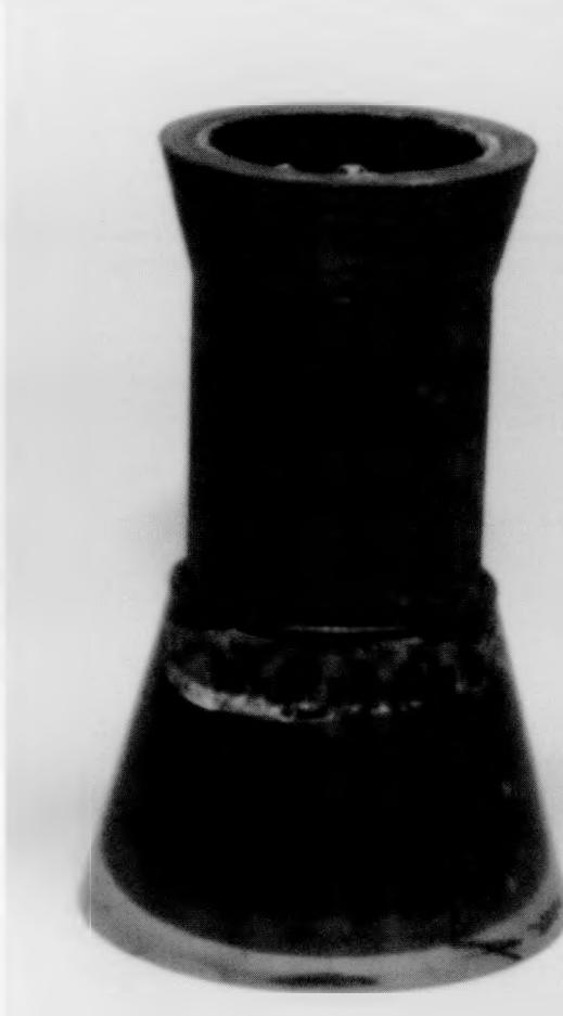
Figure 11. Pinned cylindrical shear joint for a graphite/epoxy tube.
