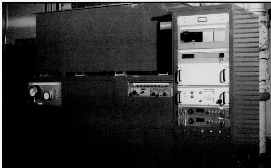
Figure 4. Completed modulator system. It includes interlocks, a triggering system, a recirculating copper-sulphate system for the ballast resistor, and heat exchangers for same. This modulator was designed and built in FY 89 to fill a need for an electron-gun driver.
