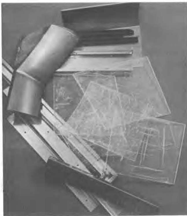
FIGURE 6. Stainless Steel, Plexiglas and Neoprene Decontaminated by Vibratory Finishing
