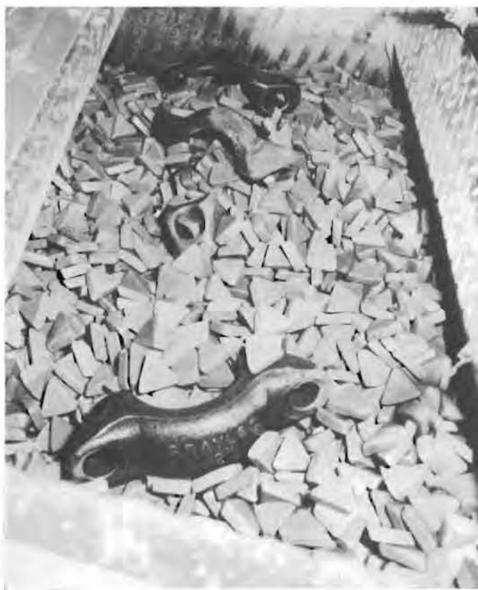
FIGURE 13. Pipe Clamps from the Hanford N-Reactor Being Decontaminated in a Vibratory Finisher
