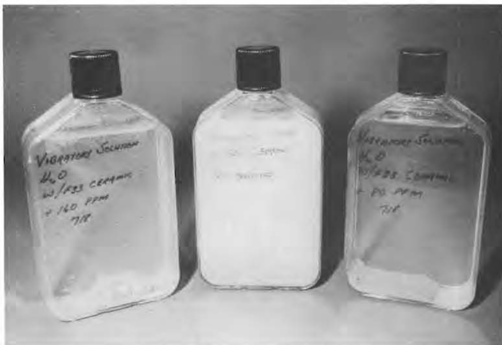
FIGURE 30. Clarification of Vibratory-Finishing Waste Using Polyelectrolytes
