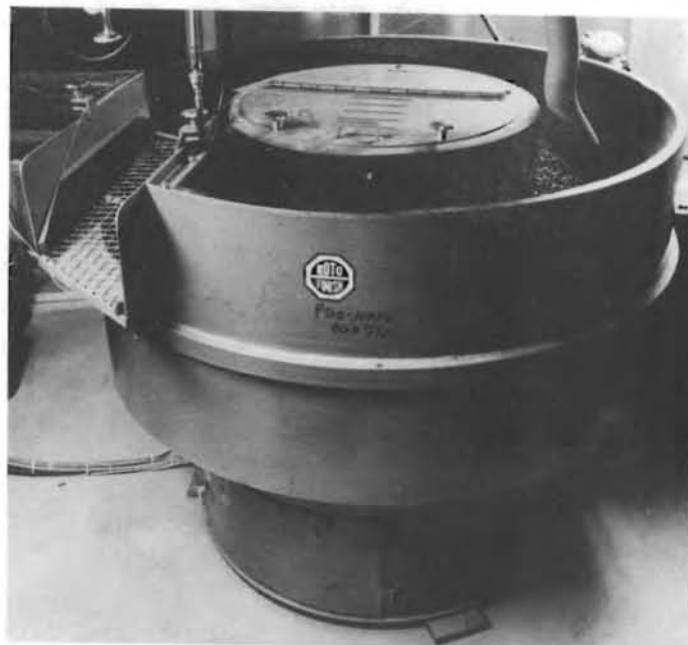
FIGURE 10. Twelve-Cubic-Foot Annular Vibratory Finisher Equipped with a Separator Screen
