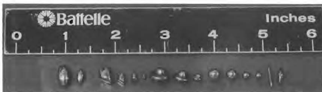
FIGURE 12. Metal Media Used for Vibratory Finishing
