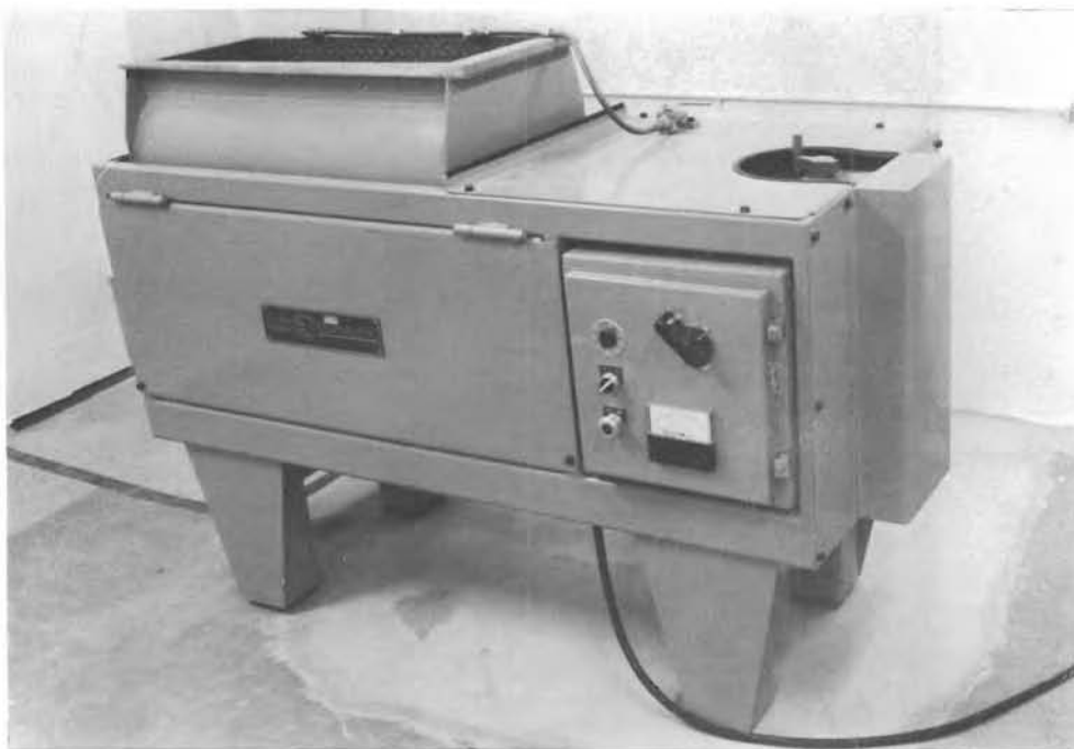
FIGURE 7. Standard Batch Tub-Type Vibratory Finisher with a 4-ft 3 Capacity
