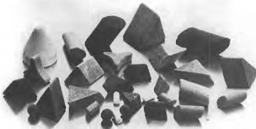
FIGURE 11. Ceramic Media Used in Vibratory Finishing
