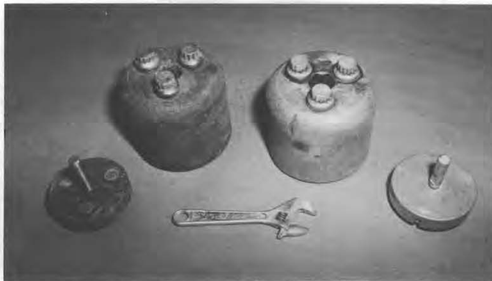
FIGURE 15. Process-Tube End Caps and Inserts Before (Left) and After (Right) Decontamination by Vibratory Finishing
