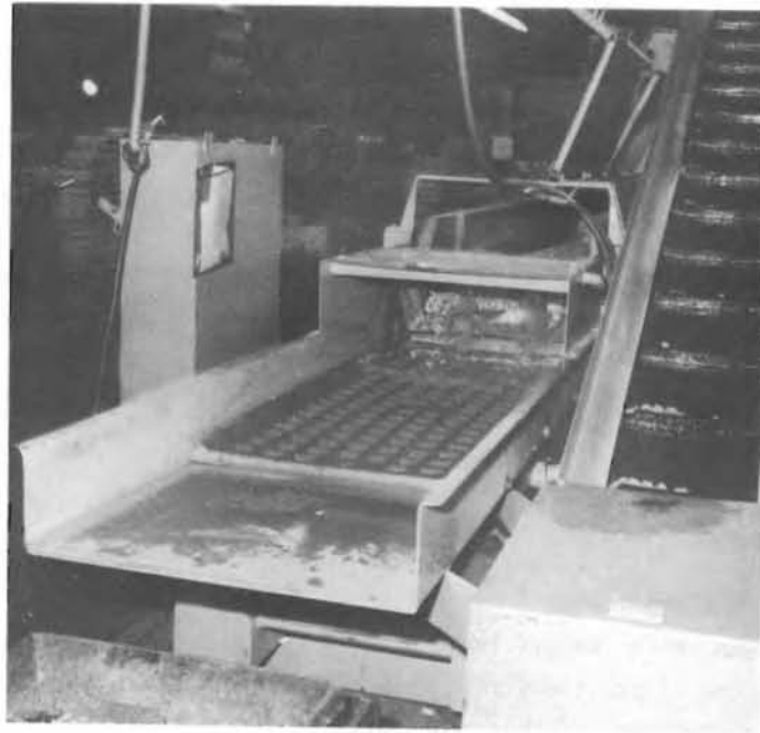
FIGURE 9. Flow-Through, Tub-Type Vibratory Finisher
