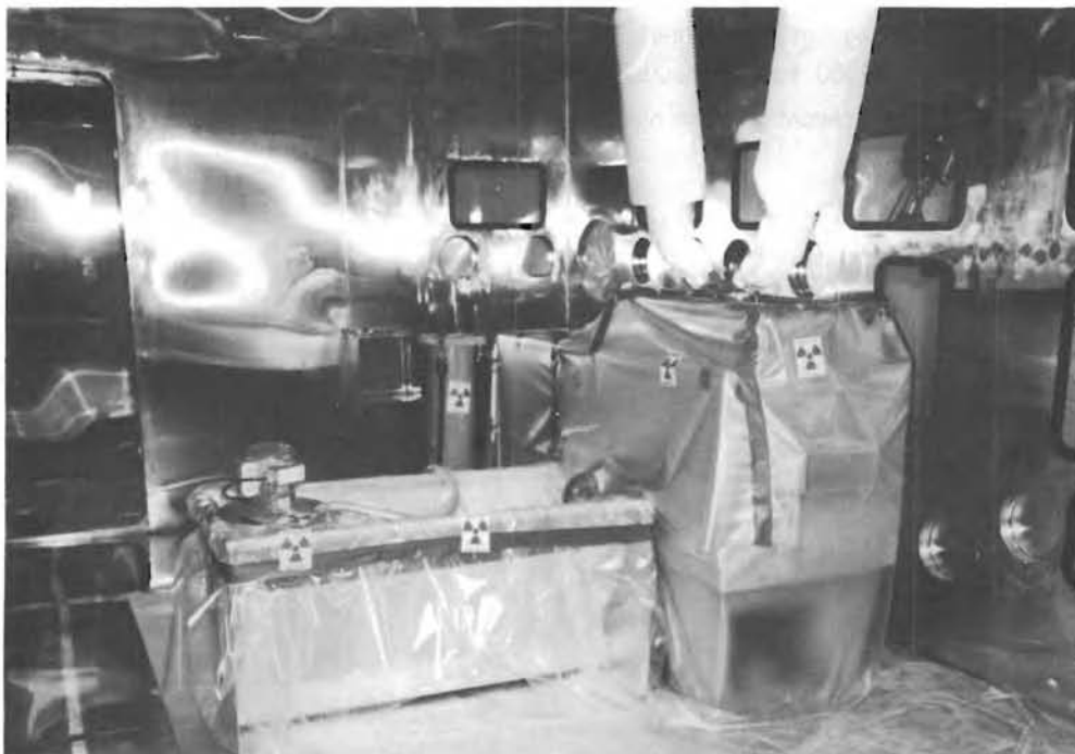
FIGURE 19. Four-Cubic-Foot, Tub-Type Vibratory-Finishing System with Recirculating Compound System Installed in the Stainless Steel, Walk-in Glove Box
