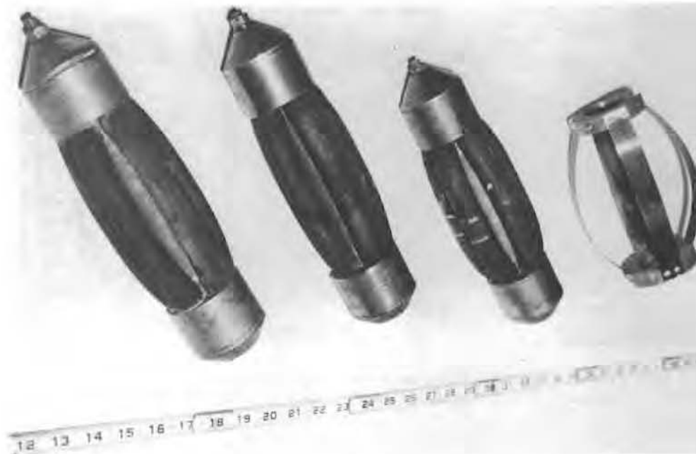
FIGURE 18. Ball-Channel Inspection Tools Used at Hanford N-Reactor After Decontamination by Vibratory Finishing
