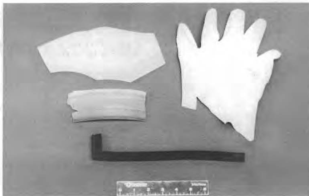
FIGURE 22. Plutonium-Contaminated Nonmetallic Material Decontaminated by Vibratory Finishing (a)
