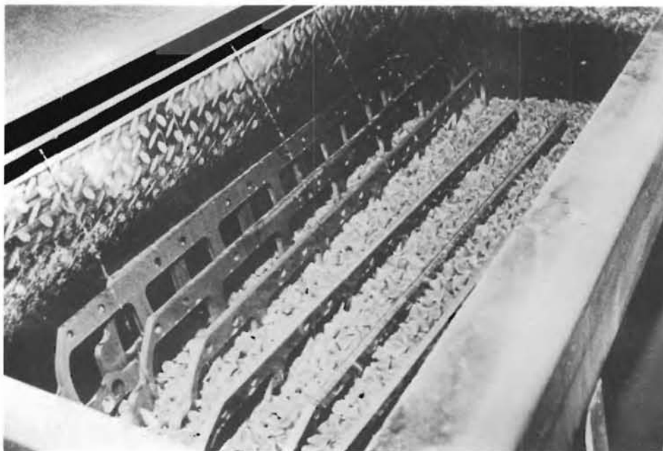
FIGURE 5. Gaskets That Demonstrate the Ability to Clean and Deburr Holes
