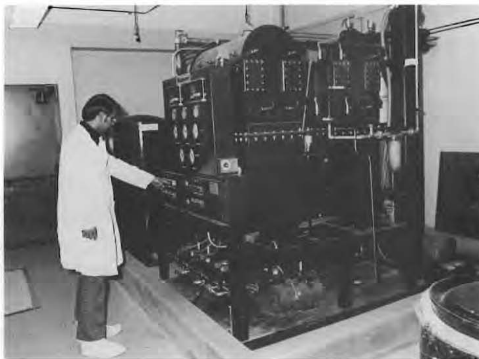
FIGURE 29. Dual-Phase Vacuum Evaporator Used to Heat Liquid Waste from Vibratory-Finishing Decontamination
