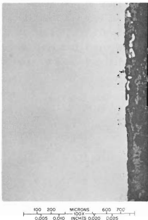
FIGURE 2: Haynes Alloy 25 Specimens Exposed for 6000 Hr to ^{90}\text{SrF}_2 Containing \text{Zr}+\text{ZrF}_4
