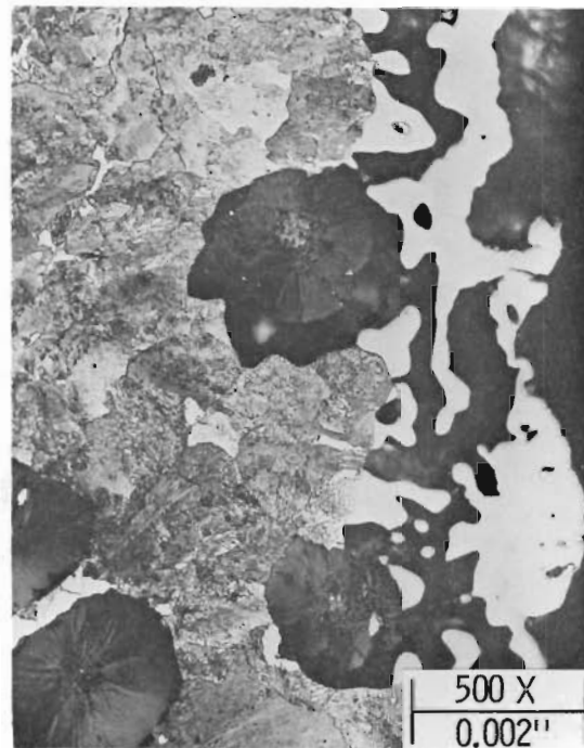
FIGURE 4: Pearlitic Anneal Ductile Cast Iron Specimen Exposed to WESF-grade Nonradioactive \text{SrF}_2 for 4400 Hr at 800°C
