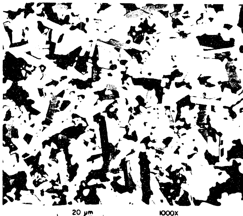
Fig. 5. Microstructure of a 93% dense \text{YBa}_2\text{Cu}_3\text{O}_7 sample. Polarized light.
