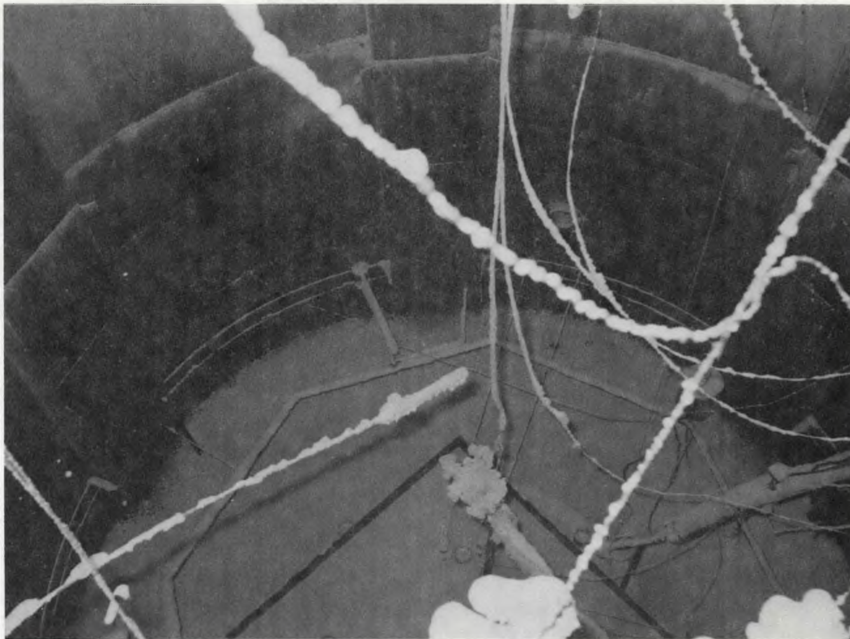
FIGURE 4-2. Post-Test View of Aerosol on Bottom Head and Lower Side Walls.
