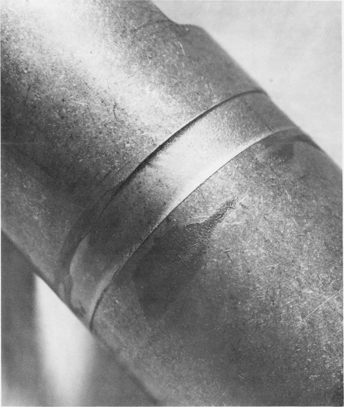
Fig. 2. Tube test specimen after a severe fretting wear test
