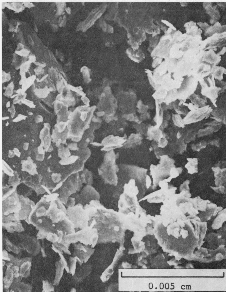
Fig. 4. Debris produced by fretting wear between Alloy 800H test specimens
