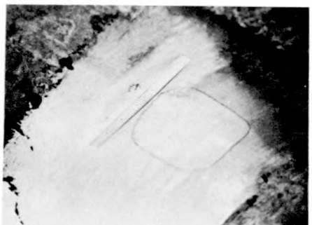
ETCHED ID AREA SHOWING HEAT-AFFECTED ZONE
