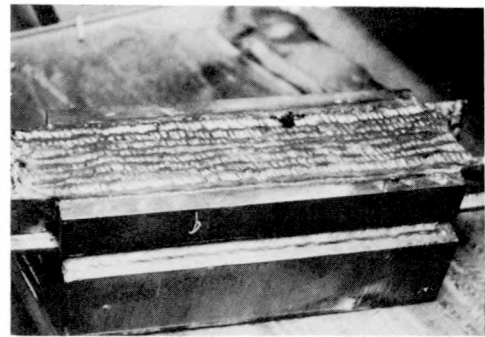
(f) TYPICAL COMPLETE WELD
