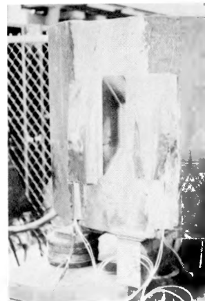
V-8 CAVITY — PROTECTIVE COVERS FOR EXTERIOR GAGES
