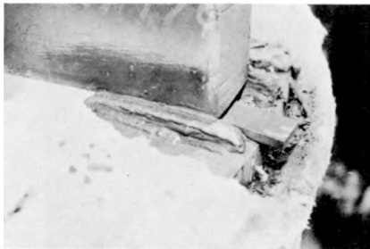
(e) BRACE RESTRAINT END WELDMENT
