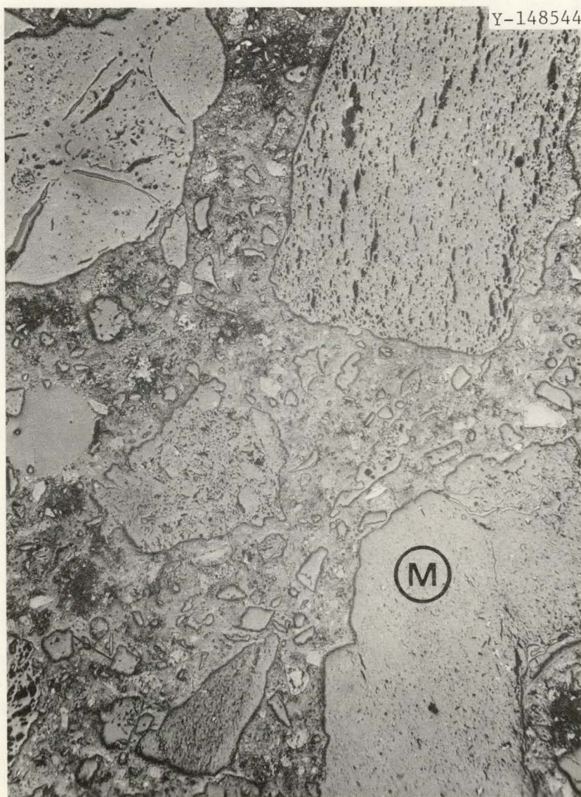
Fig. 2. Reflected-Light Photomicrograph of the Unaltered Zone Showing Mullite Grog Particles (M) Bonded with a Matrix Material Containing Gehlenite, Quartz, and a Siliceous Glassy Phase. 50 \times .
