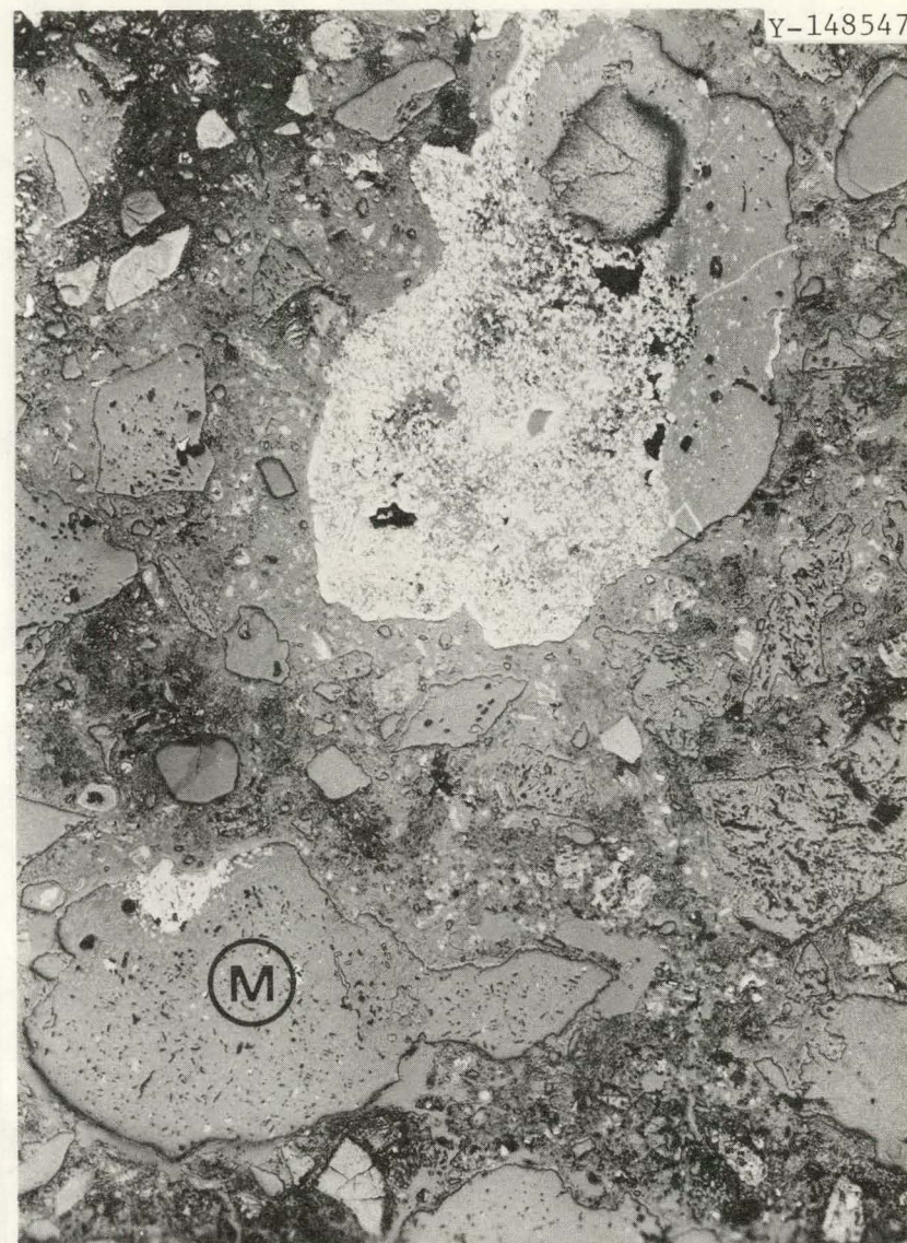
Fig. 3. Reflected-Light Photomicrograph of the Unaltered Zone Showing Mullite Grog Particles (M) Bonded with a Matrix Material Containing Gehlenite, Quartz, and a Siliceous Glassy Phase. Highly reflecting phases are rutile and hematite. 100 \times .
