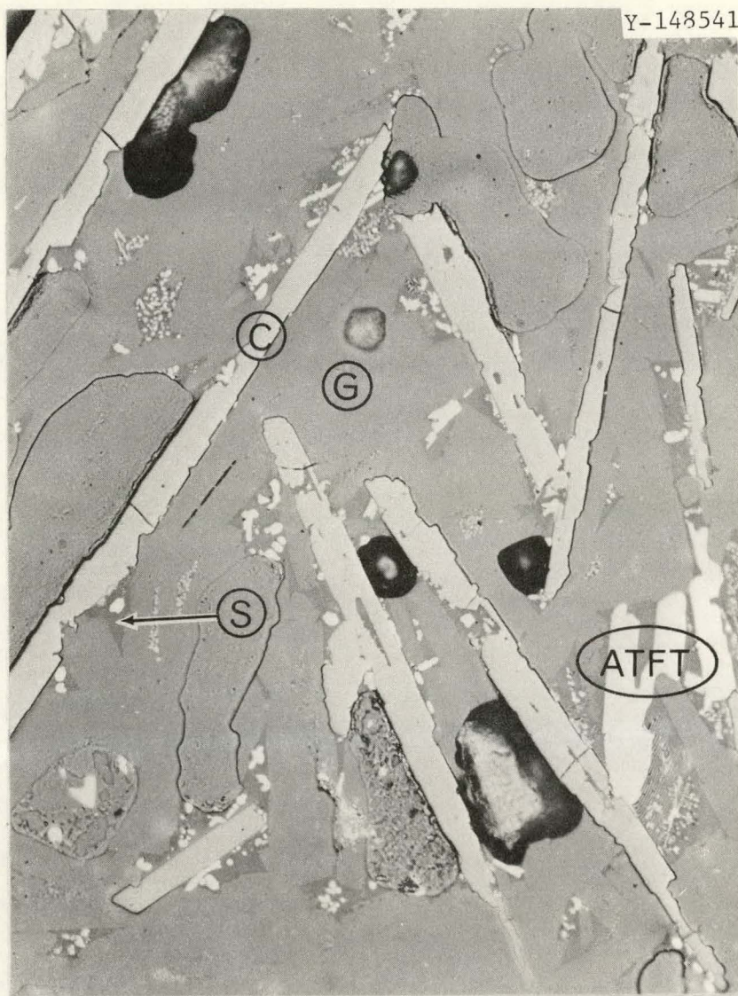
Fig. 6. Reflected-Light Photomicrograph of the Altered Zone Showing Long Corundum Crystals (C) in a Matrix Containing Gehlenite (G) and a New Siliceous Glassy Phase (S). Highly reflecting phase is an Al-Ti-Fe oxide compound (ATFT). 500 \times .
