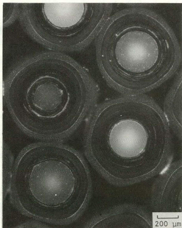
Fig. 3-19. Representative photomicrographs of TRISO-coated \text{ThO}_2 batch 6252-17-010 for capsule HT-34: bright field and polarized light
