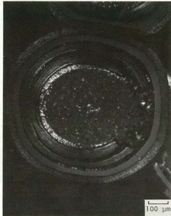
Fig. 5-10. Photomicrographs of kernel migration of a particle irradiated at 1490°C to a burn-up of 10.5% FIMA: (a) bright field; (b) polarized light
