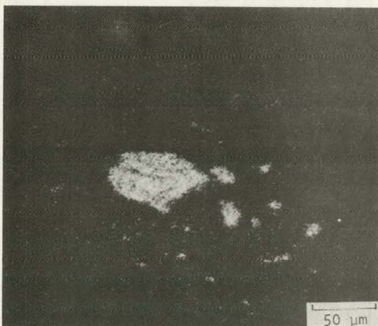
Fig. 5-13b. Results of electron microprobe of center of kernel of sample 17 irradiated at 1430°C to a burnup of 10.9% FIMA: (a) optical micrograph; (b) Mo L\alpha ; (c) Ru L\alpha
