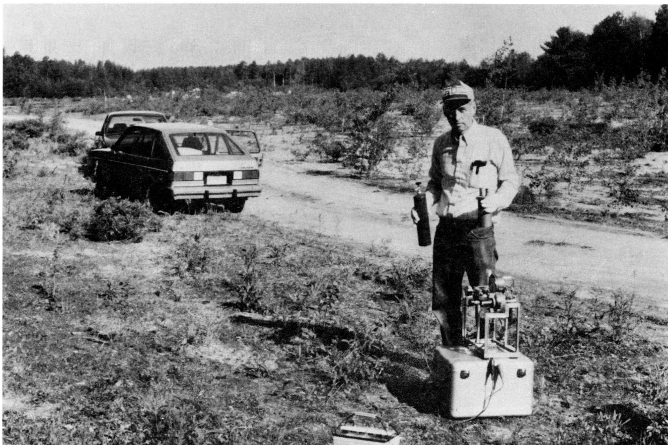
Fig. 7. Savannah River Laboratory air sampler. The view is of the field looking upwind toward the release point.
