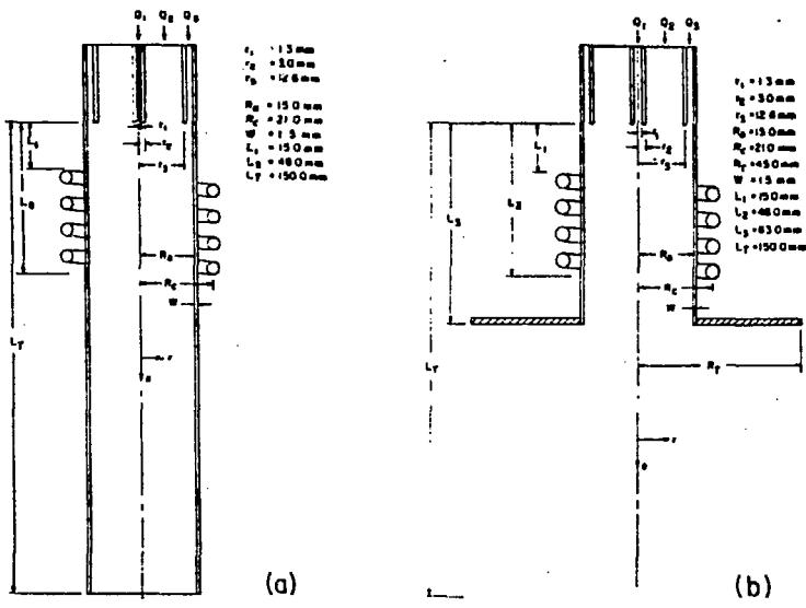
Figure 1: TORCH GEOMETRIES USED FOR THE (a) CONFINED AND (b) FREE PLASMA CALCULATIONS.
