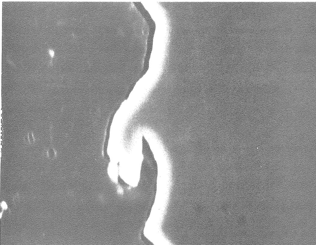
FIGURE 23. 7075-T6 Aluminum Cross-Sectioned Transverse to Abrading Direction.
