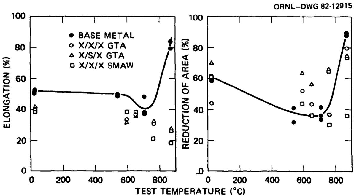
Fig. 12. Ductility parameters of Hastelloy X base metal and weldments.
