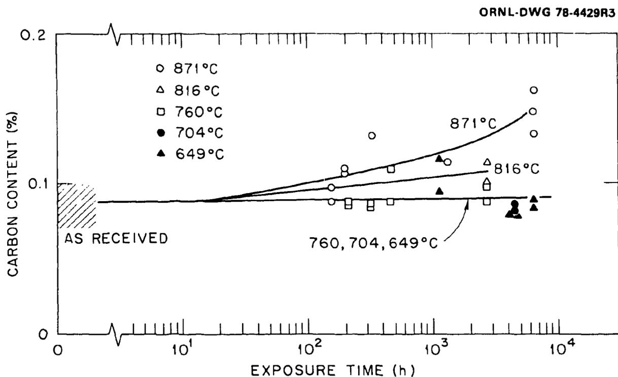
Fig. 25. Carbon content of Hastelloy X exposed to HTGR helium.
