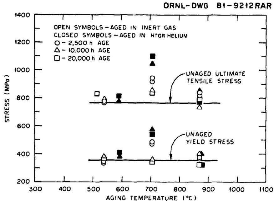
Fig. 4. Influence of aging on yield and ultimate tensile stresses of Hastelloy X base metal (heat 4936) at 25°C.
