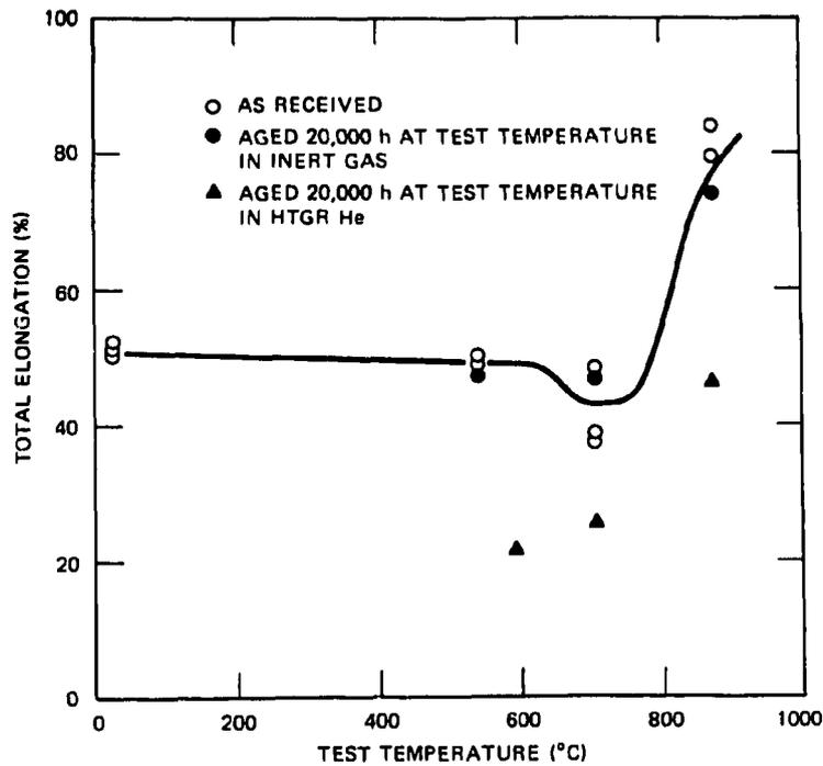
Fig. 8. Influence of aging on elongation of Hastelloy X (heat 4936) aged and tested at the same temperature.
