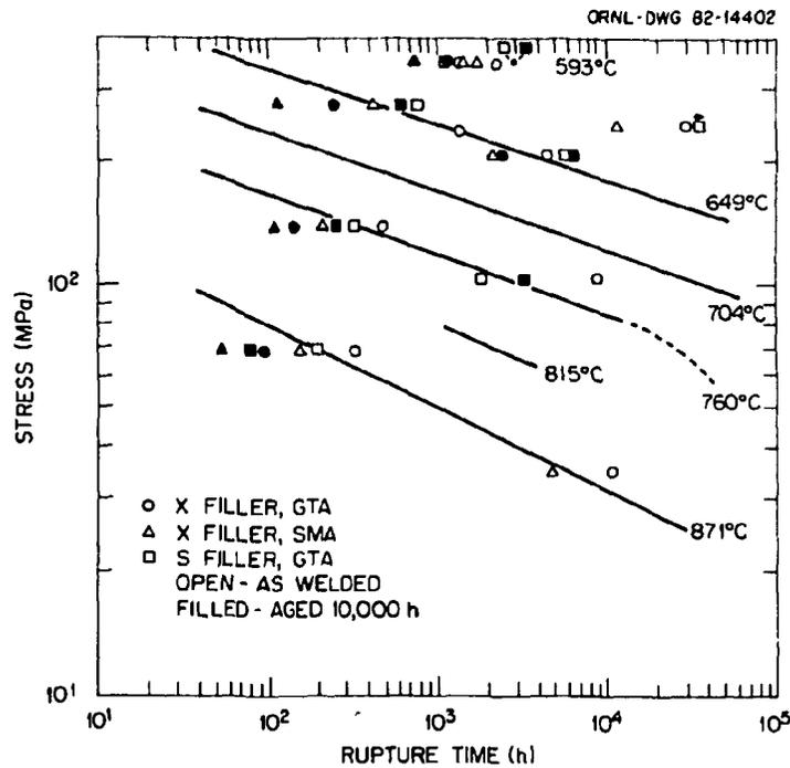
Fig. 27. Comparison of times to rupture for Hastelloy X base metal and three weldments. All tests were conducted in HTGR helium; the lines represent base metal.
