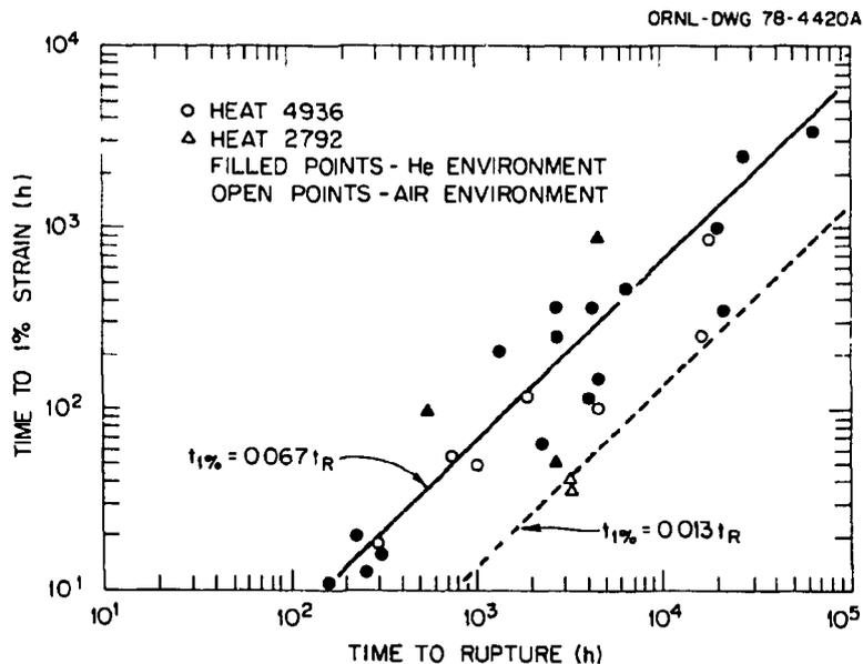
Fig. 22. Time to 1% strain as a function of rupture life for Hastelloy X.
