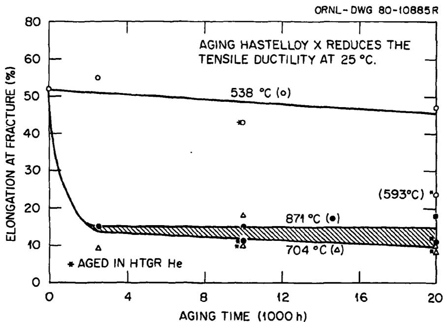
Fig. 6. Aging Hastelloy X (heat 4936) reduces the tensile ductility at 25°C.
