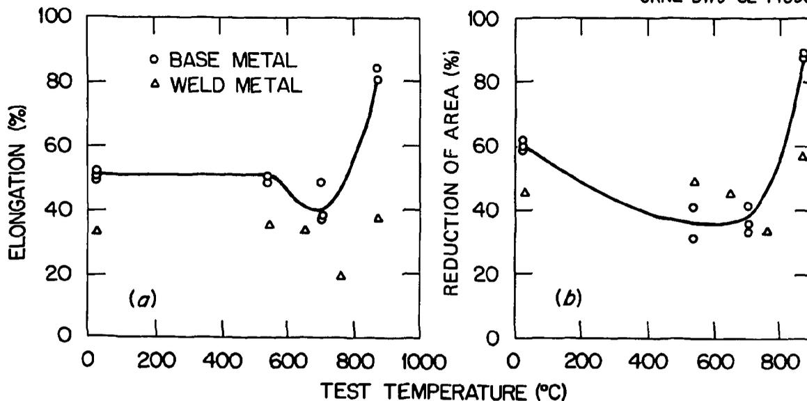
Fig. 10. Comparison of ductility parameters of Hastelloy X base (heat 4936) and weld (heat 4345) metal samples.
