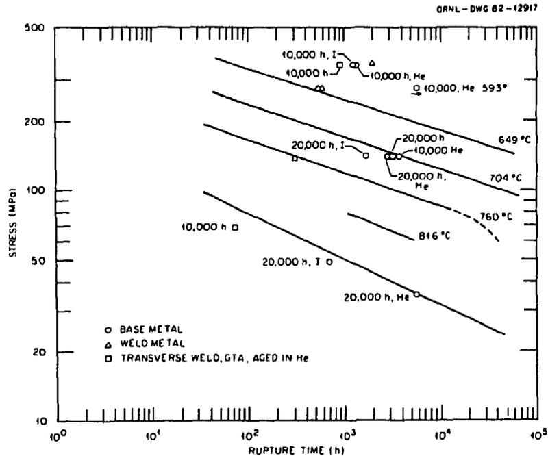
Fig. 31. Comparison of stress-rupture properties of Hastelloy X in a number of conditions. The lines represent as-received Hastelloy X base metal.
