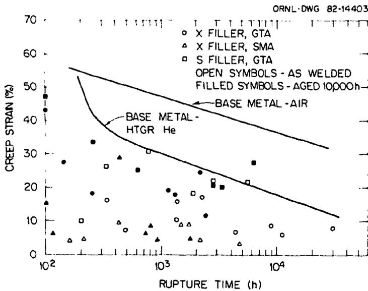
Fig. 29. Comparison of fracture strains for Hastelloy X base metal and three weldments. All weldment tests were conducted in HTGR helium.
