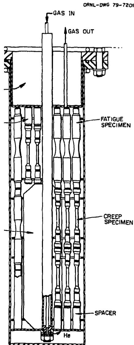
Fig. 3. Environmental exposure chamber.
