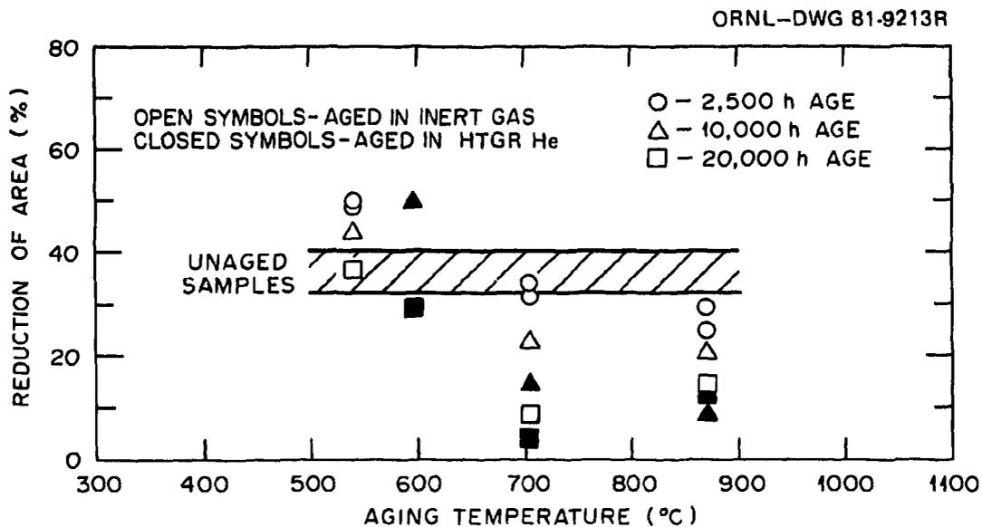
Fig. 5. Influence of aging on reduction of area of Hastelloy X (heat 4936) tested at 25°C.
