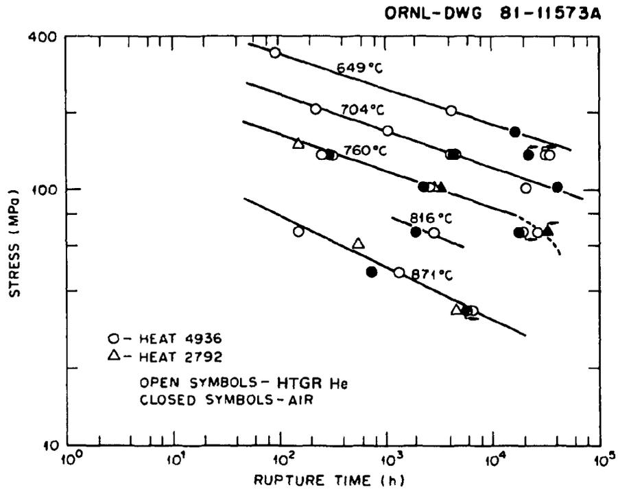
Fig. 20. Stress-rupture properties of Hastelloy X. Arrows with data points indicate that tests are still in progress.
