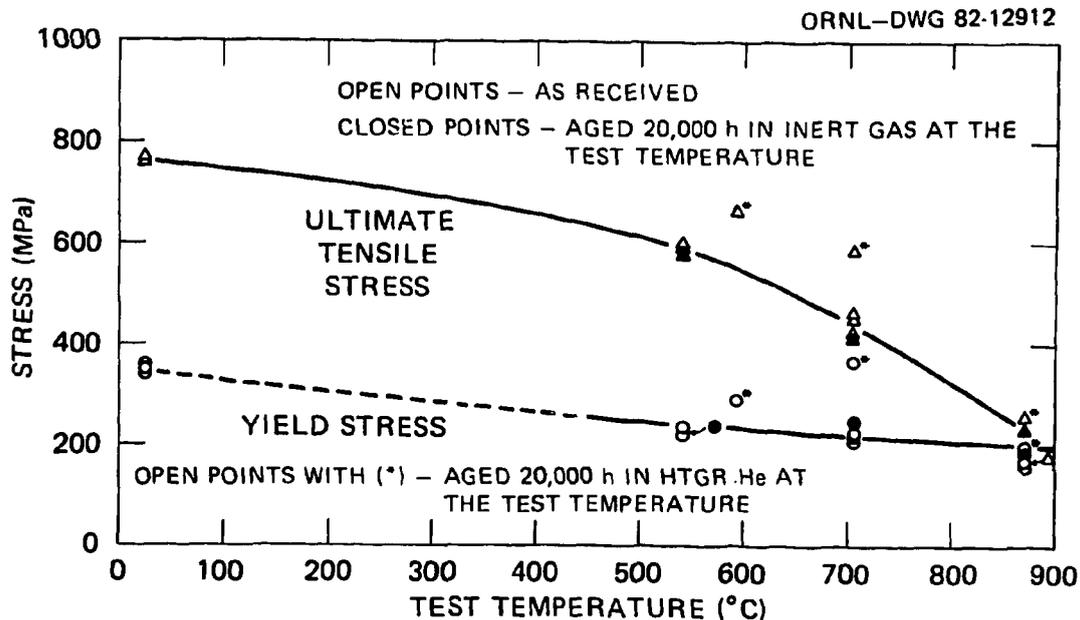
Fig. 7. Influence of aging on yield and tensile strengths of Hastelloy X (heat 4936) aged and tested at the same temperature.
