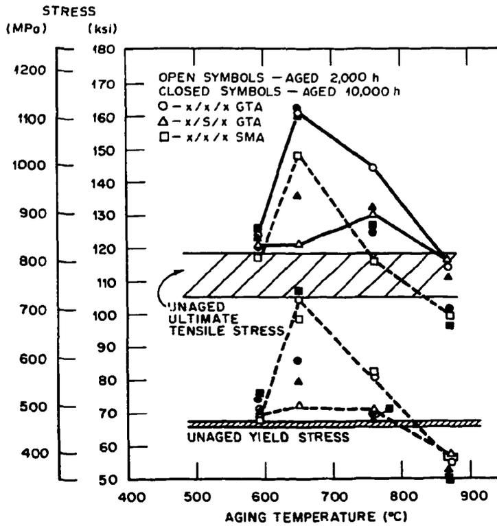
Fig. 14. Influence of aging on the yield and ultimate tensile stresses of three Hastelloy X weldments measured at 25°C.
