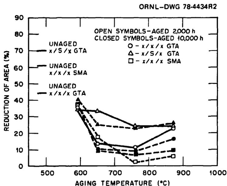
Fig. 15. Influence of aging on the reduction of area of three Hastelloy X weldments measured at 25°C.
