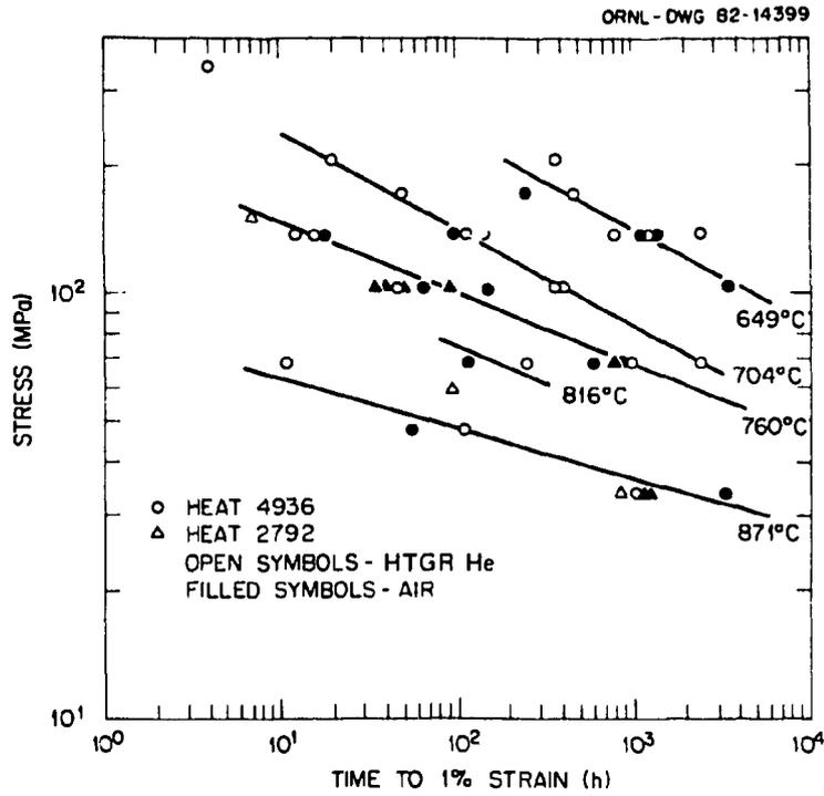
Fig. 18. Time to 1% strain as a function of stress for Hastelloy X.
