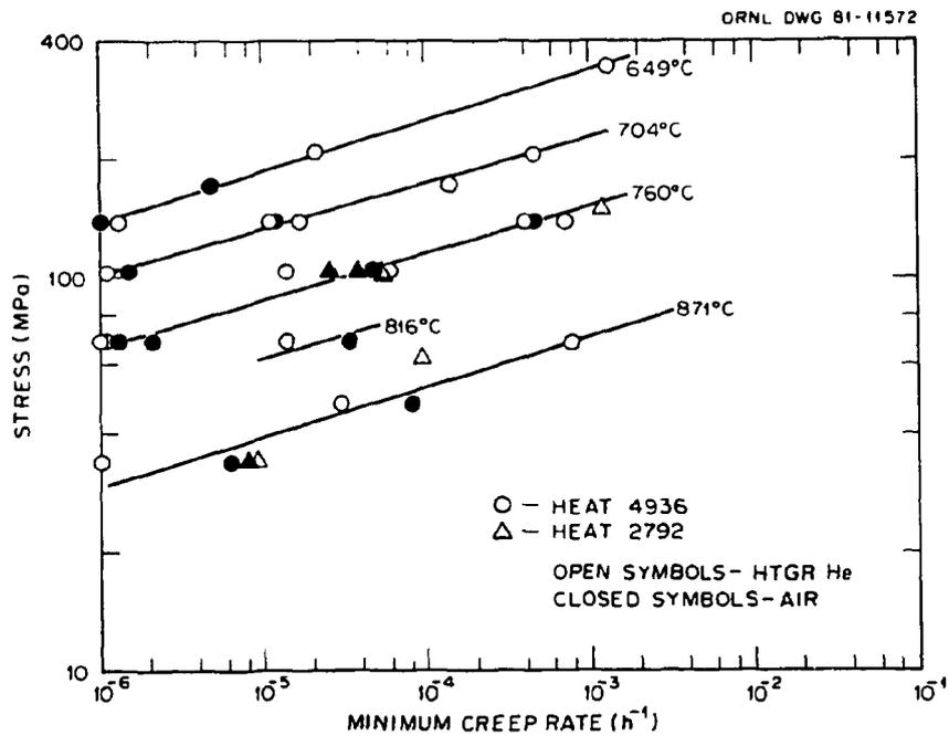
Fig. 21. Minimal creep rate for Hastelloy X under various experimental conditions.
