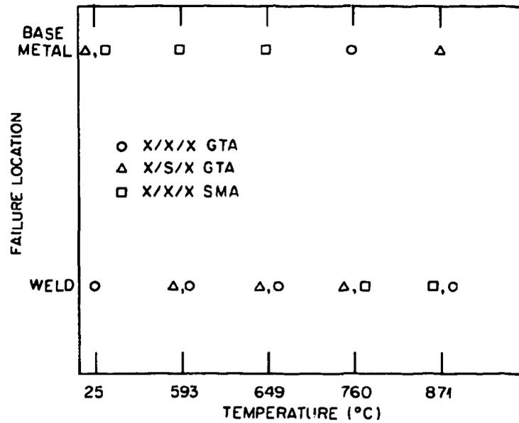
Fig. 13. Fracture location in transverse weldments does not follow a consistent pattern.
