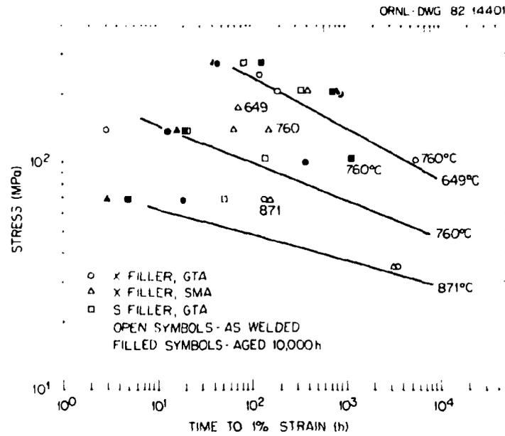
Fig. 26. Comparison of time to 1% strain for Hastelloy X and three weldments. The lines are taken from the base metal.
