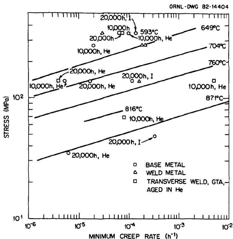
Fig. 30. Comparison of the creep rate of Hastelloy X in a number of conditions. The lines represent as-received Hastelloy X base metal.
