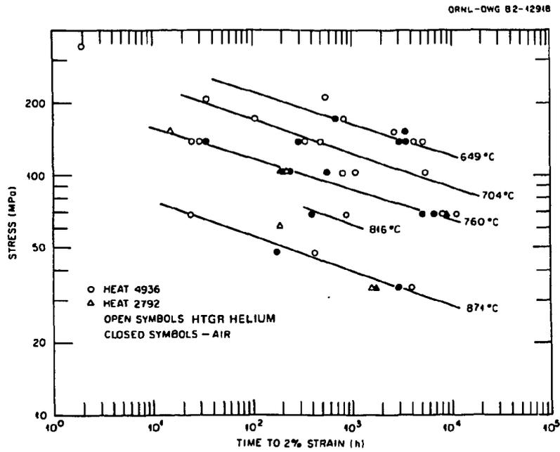
Fig. 19. Time to 2% strain as a function of stress for Hastelloy X.
