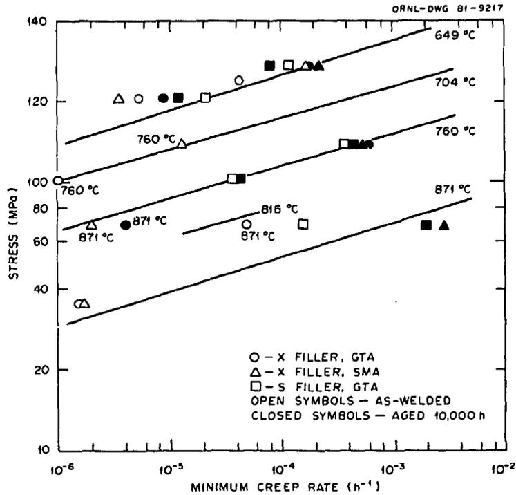
Fig. 28. Comparison of minimum creep rates of Hastelloy X base metal and three weldments. All tests were conducted in HTGR helium; the lines represent base metal.
