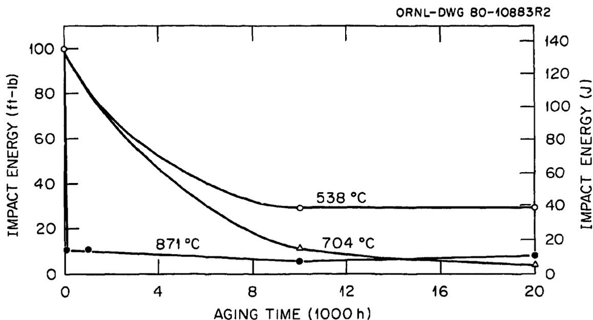
Fig. 16. Effect of aging on impact properties of Hastelloy X at 25°C.
