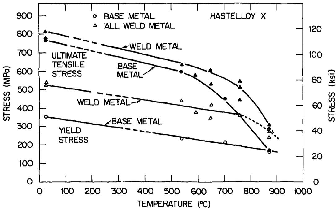
Fig. 9. Comparison of tensile strength parameters of Hastelloy X base (heat 4936) and weld (heat 4345) metal samples.
