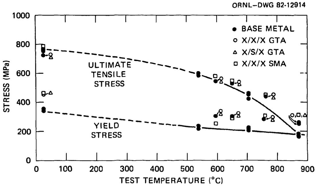
Fig. 11. Yield and tensile stresses of base metal and weldments.
