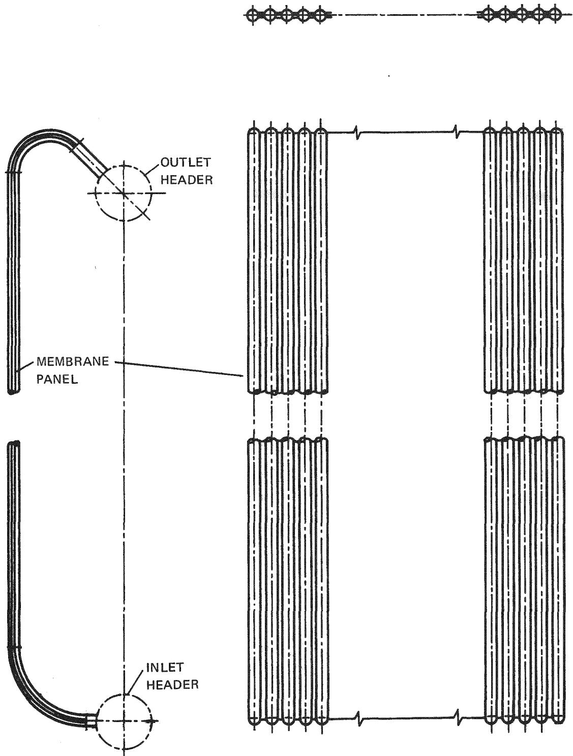
Figure 3-3. SRE Membrane Panel Arrangement
