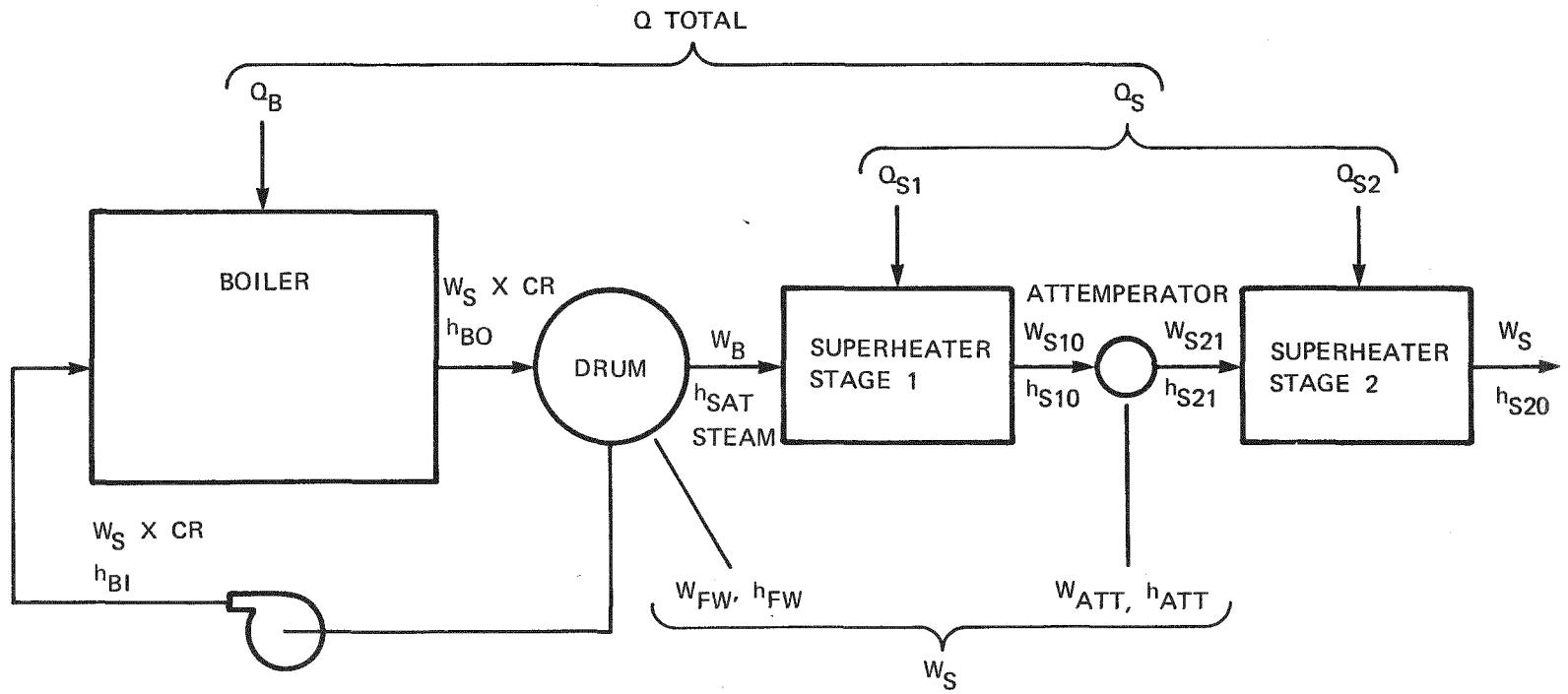
Figure A-1. Solar Boiler Flow Diagram
