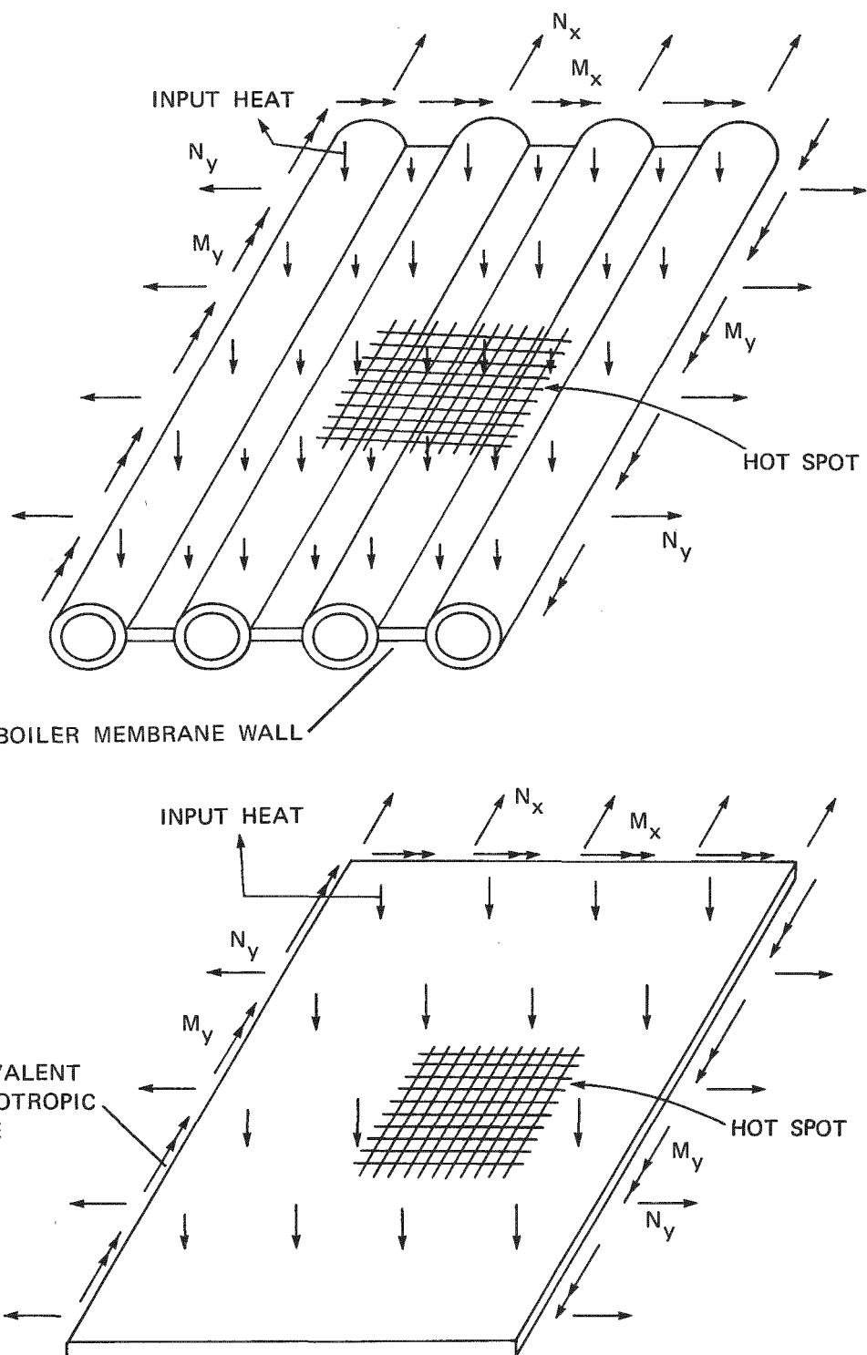
Figure D-6. Boiler Section Panel Modeling
