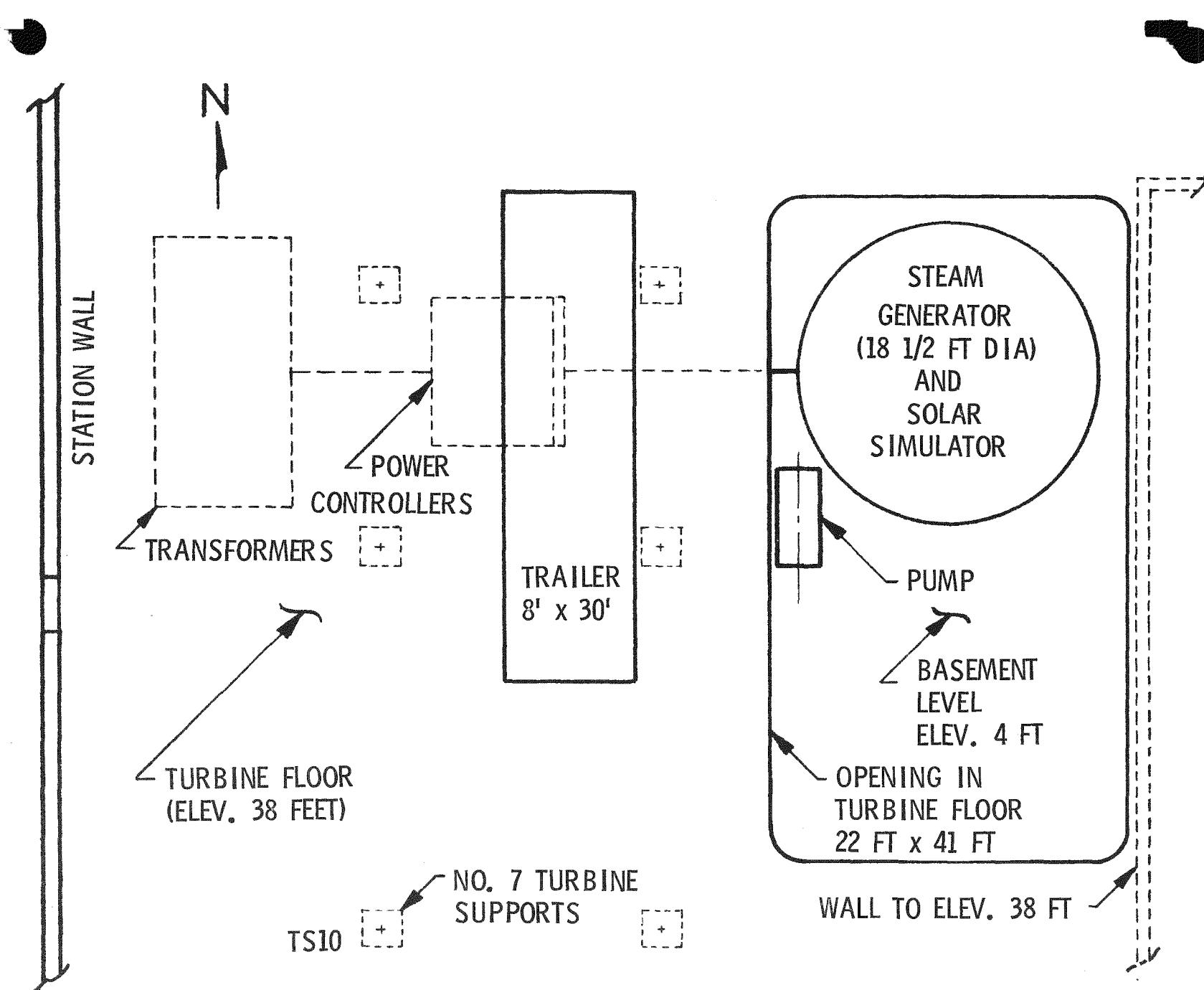
Figure 6-2. Plan of Test Installation Steam Generator
