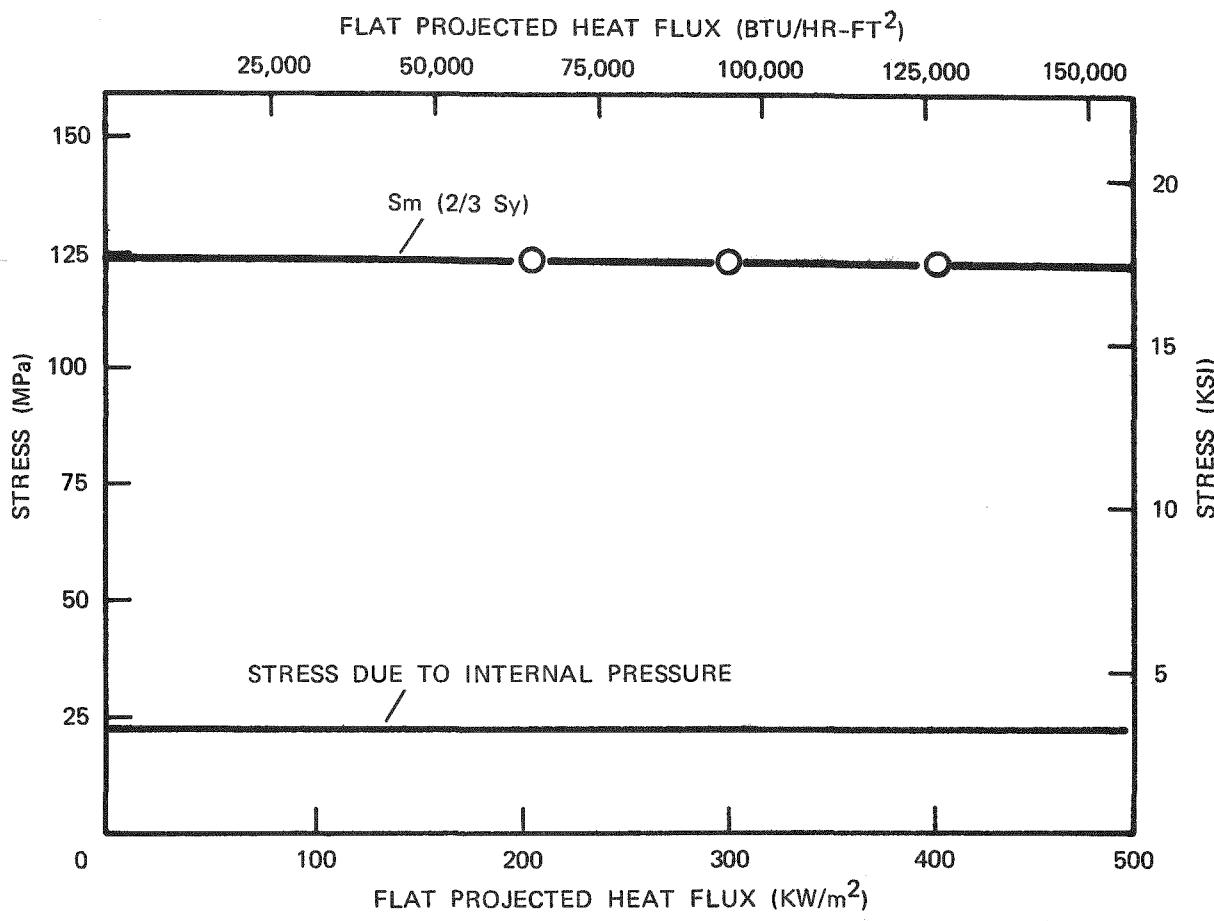
COMPARISON OF THE PRESSURE STRESS TO THE ALLOWABLE STRESS
