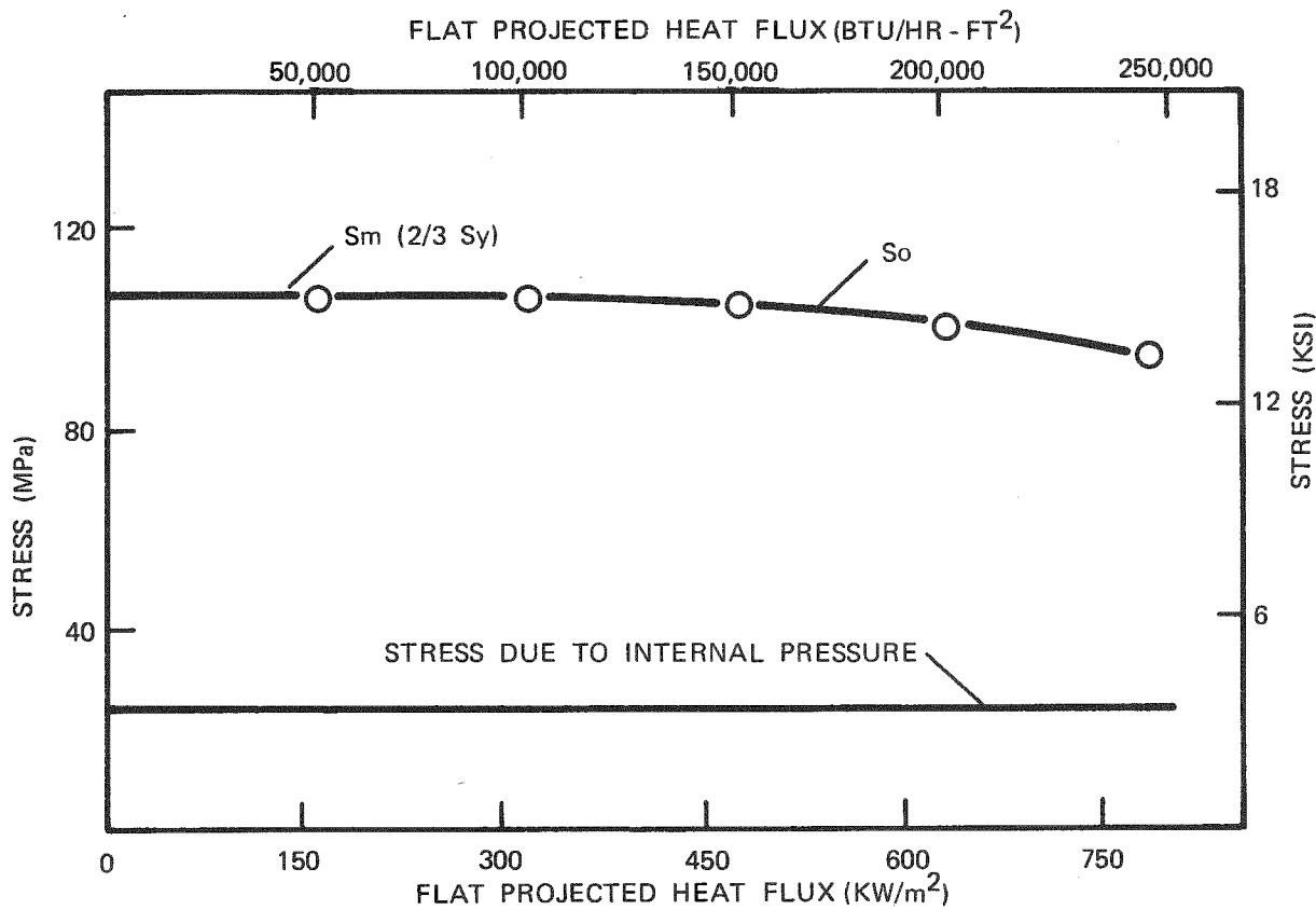
Figure D-1. Comparison of Stress Due to Pressure in the Boiler Section to the Allowable Stress
