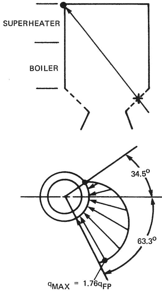
Figure E-3. Heat Flux Distribution on the Lower and
