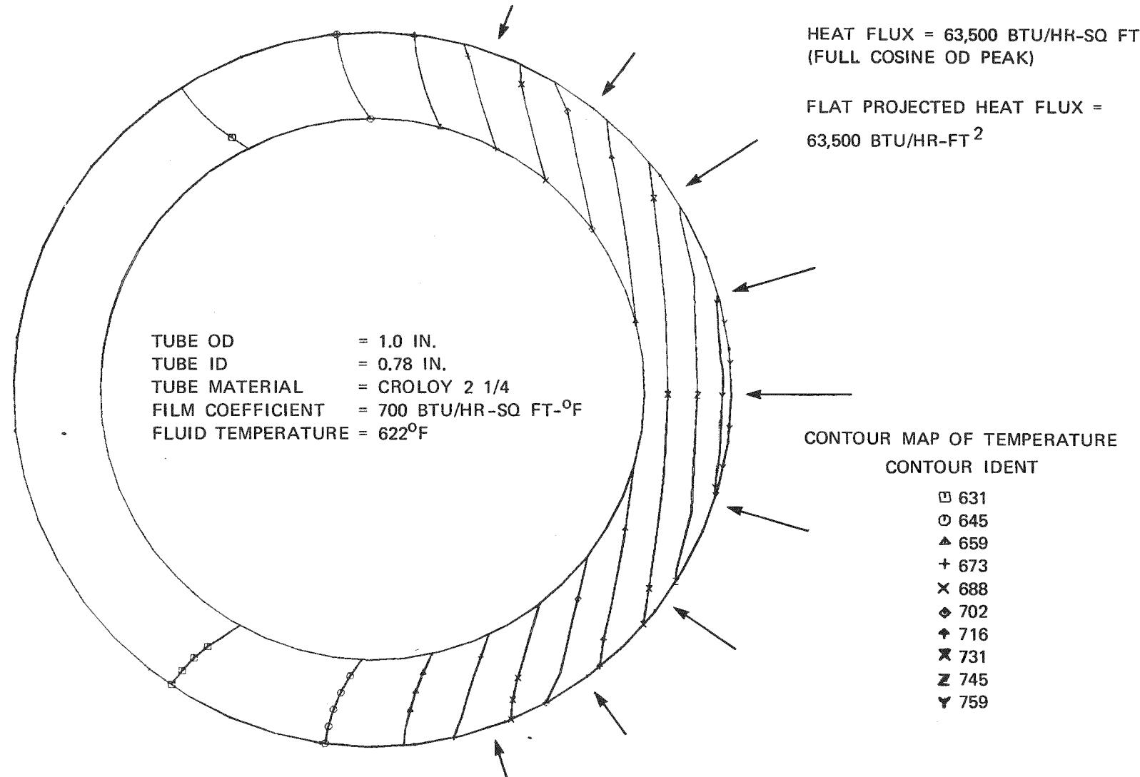
Figure D-15. Temperature Contour Lines in Pilot Plant Superheater Tubes
