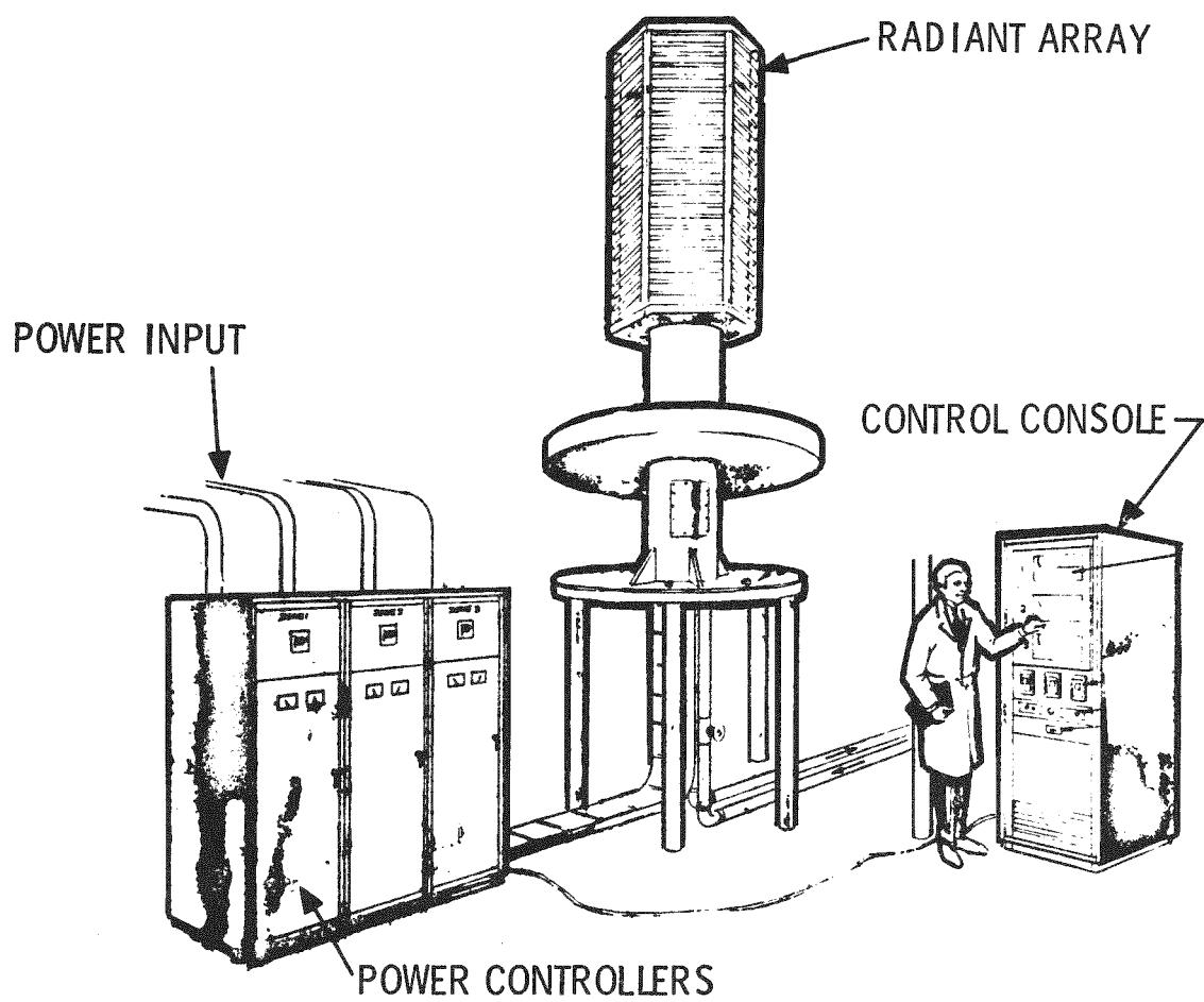
Figure 6-7. Solar Simulator System
