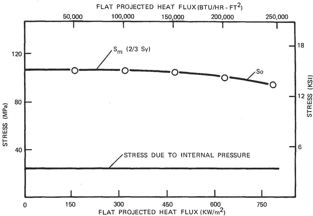
COMPARISON OF STRESS DUE TO PRESSURE IN THE BOILER SECTION TO THE ALLOWABLE STRESS
