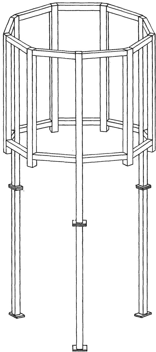
Figure 2-4. SRE Structural Support Frame
