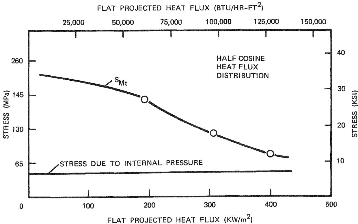
Figure D-8. Comparison of the Pressure Stress in the Pilot Plant Superheater Tubing to the Allowable Stress
