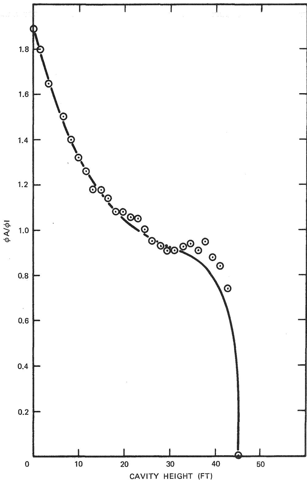
Figure A-2.  $\phi_A/\phi_I$  versus Cavity Height
