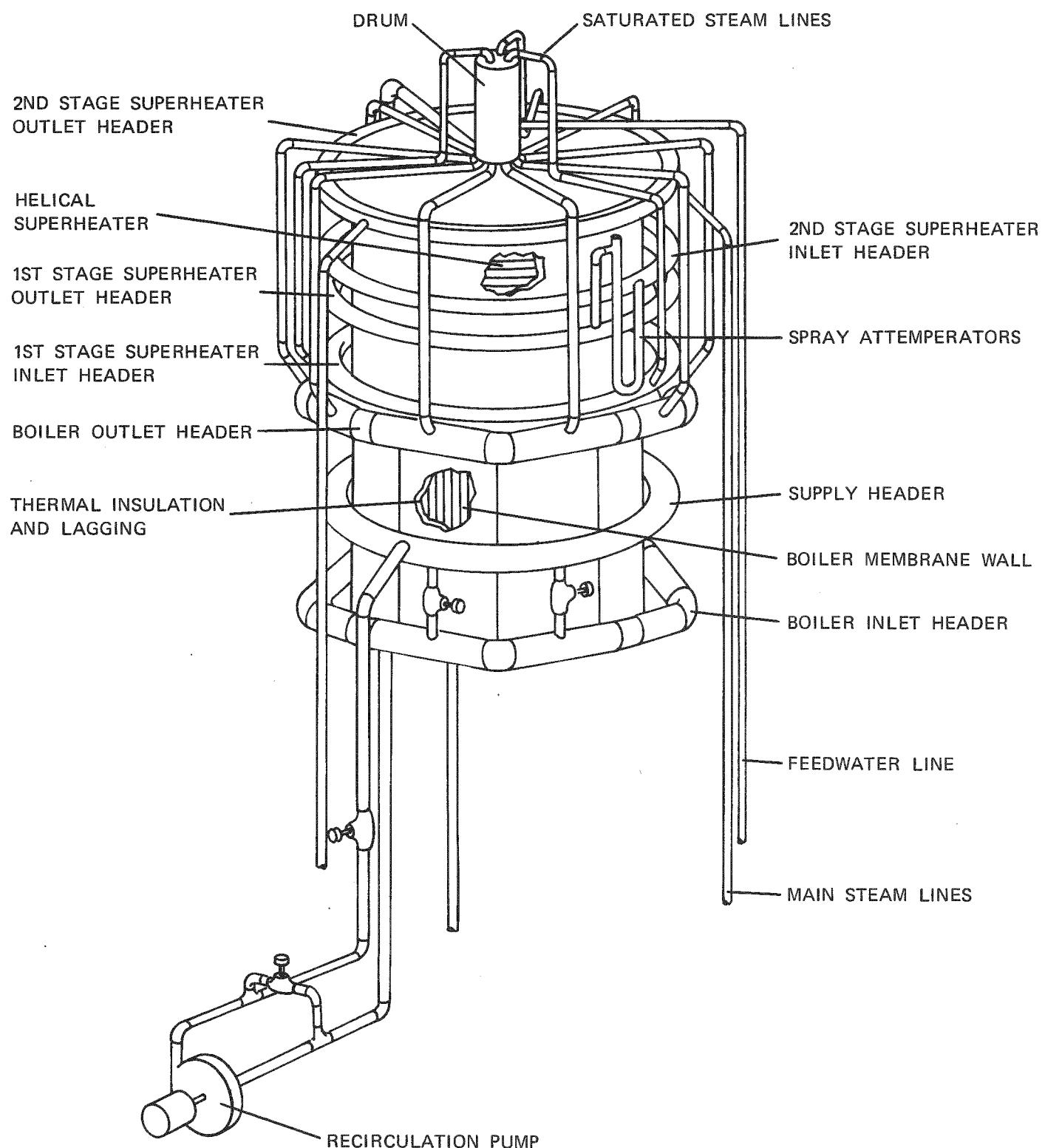
Figure 2-3. SRE Design Arrangement
