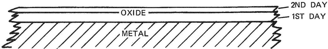
B) WHEN THE OXIDE REACHES A CRITICAL VALUE, IT CRACKS AND FLAKES OFF (SPALLING).
