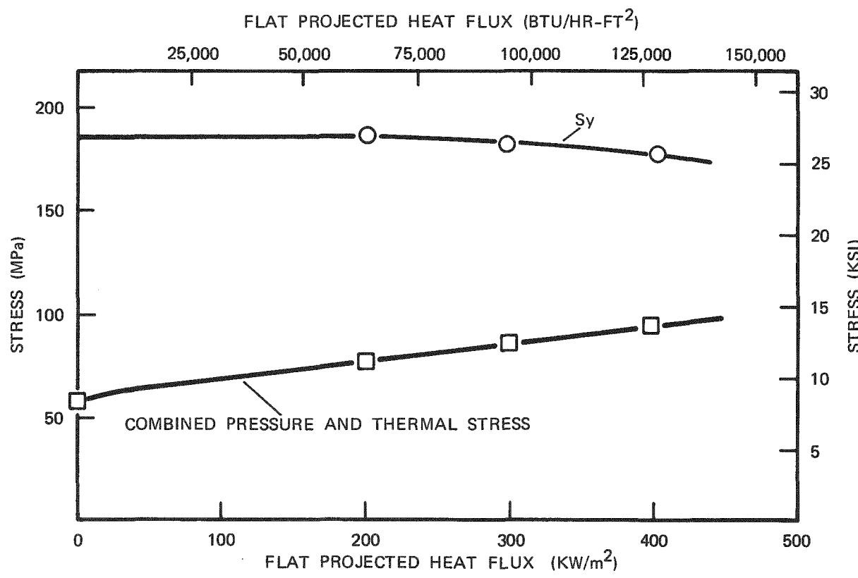
Figure 3-14. Superheater Stress Analysis - Pilot Plant
