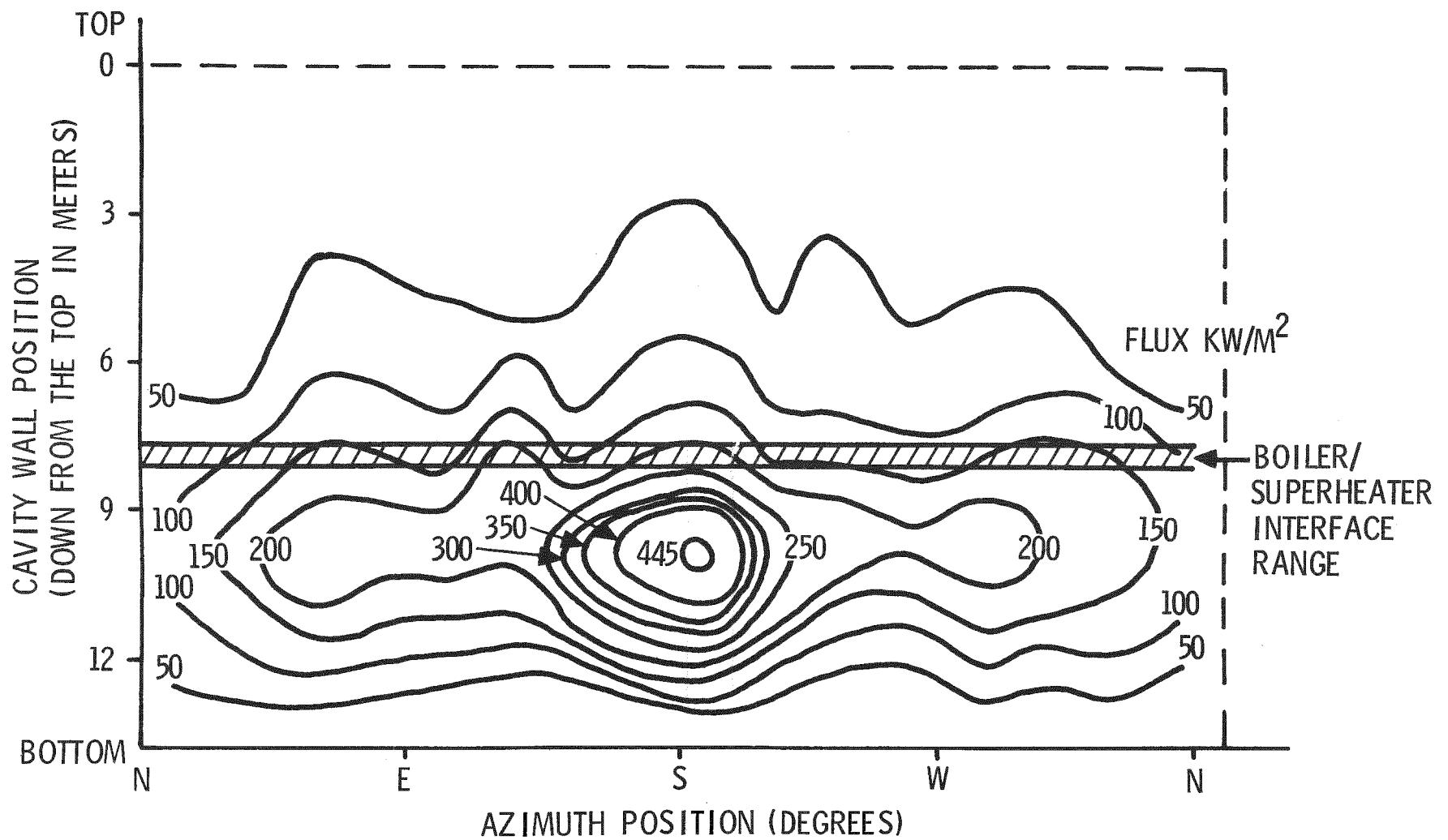
Figure J-2. Cavity Wall Incident Flux Map for 12/21 Noon
