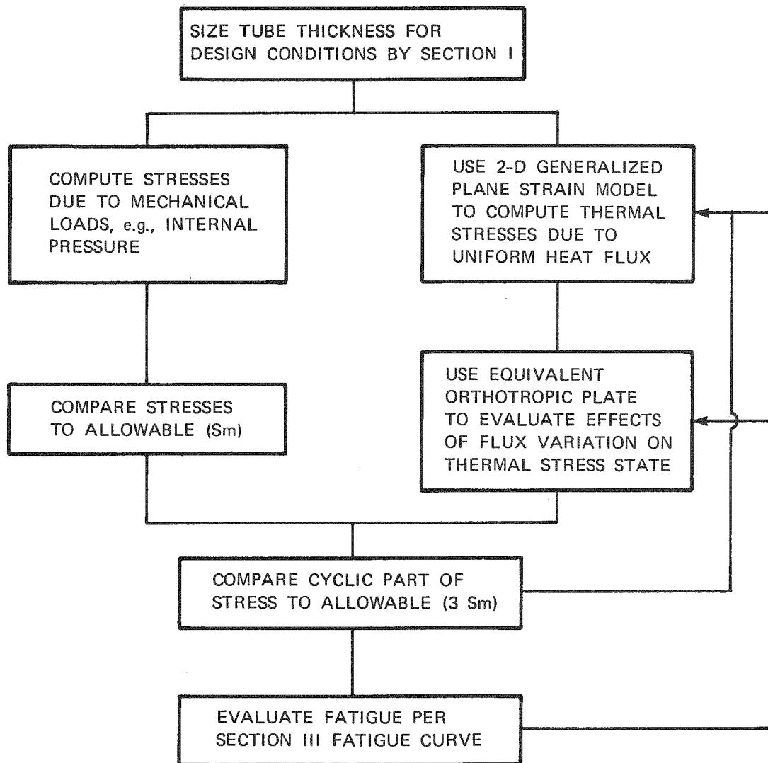
Figure C-1. Boiler Section Stress Analysis
