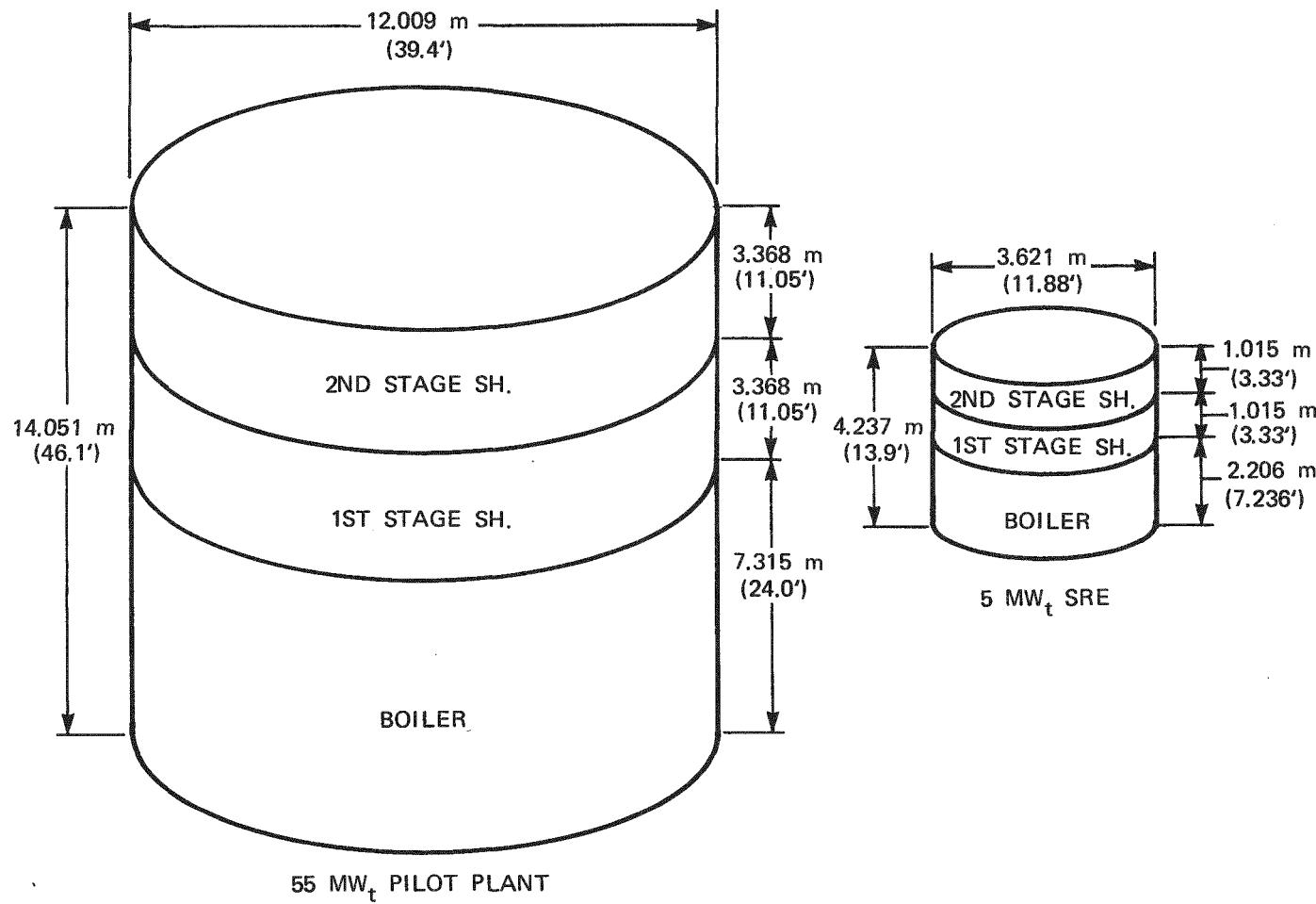
Figure 2-5. Cavity Size
