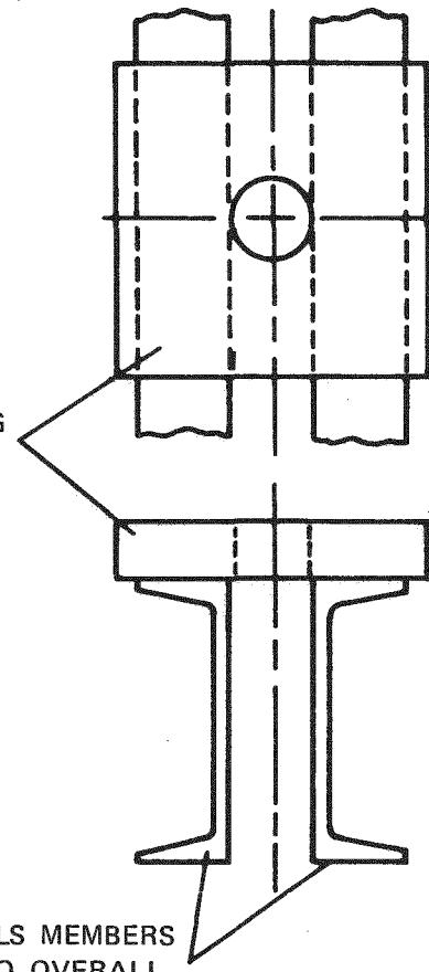
Figure F-3. Rocker and Bearing Plate Support
