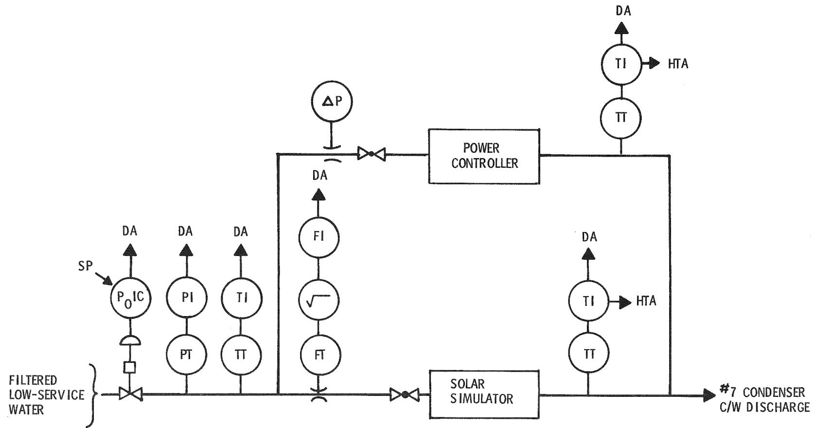
Figure 6-4. Solar Simulator Cooling Water Control Schematic
