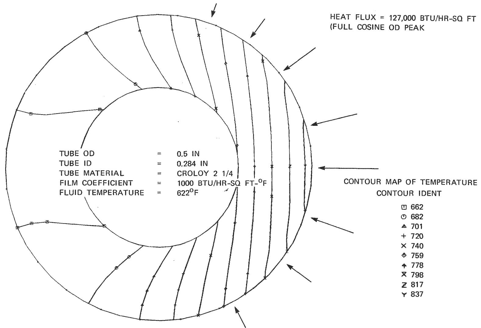
Figure D-9. Temperature Contour Lines in SRE Superheater Tubes Due to Heat Flux of 127,000 Btu/Hr-Sq Ft (Full Cosine OD Peak)
