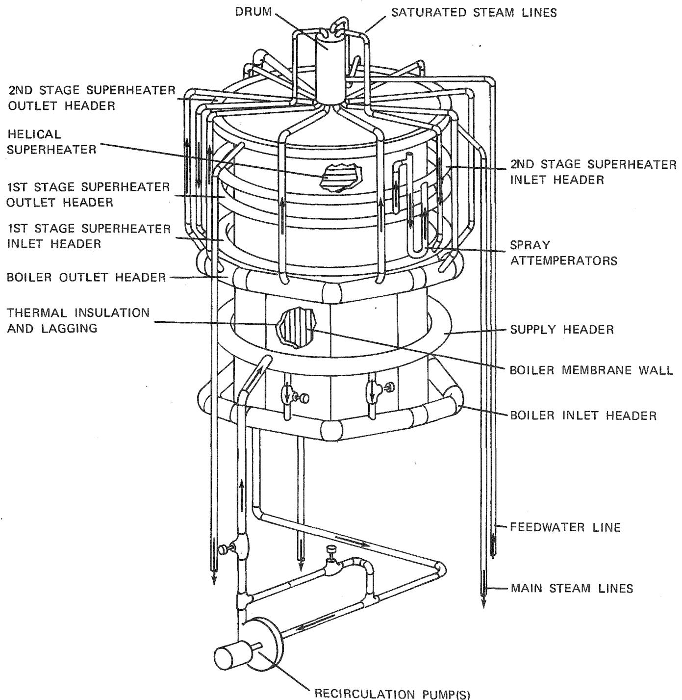
Figure 2-2. Pilot Plant Design Arrangement
