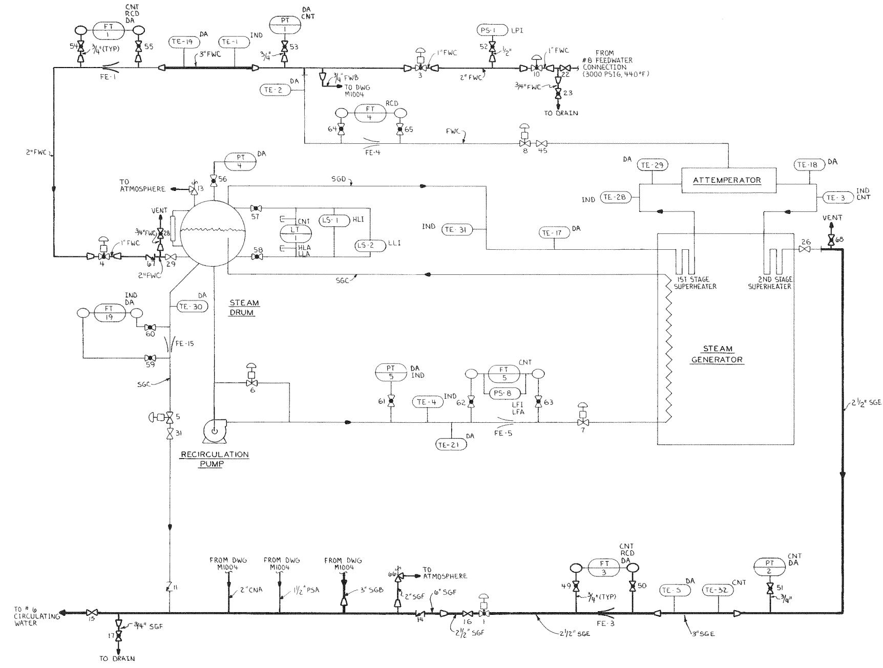
Figure I-2. Piping and Instrument Diagram Steam Generator SRE
