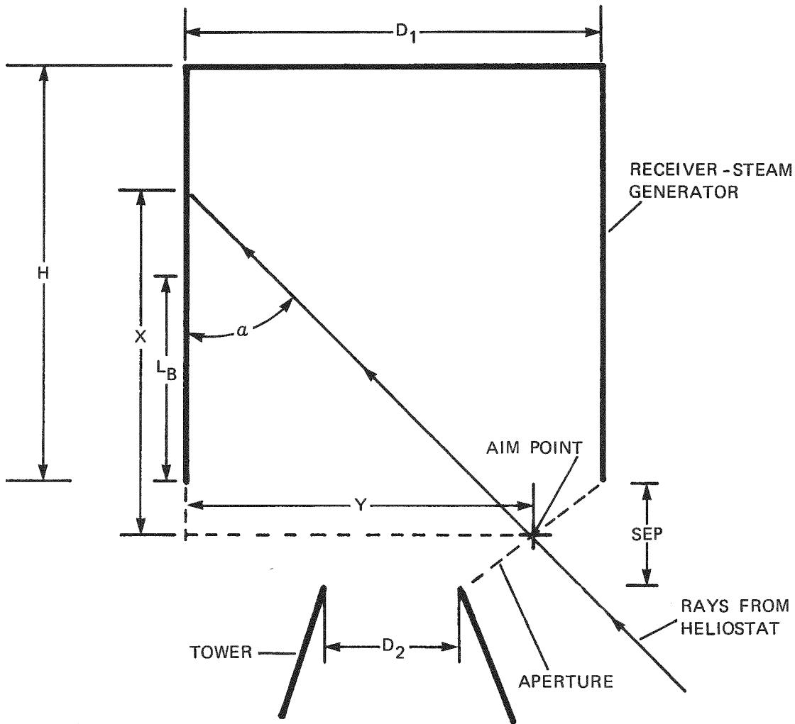
Figure E-1. Pilot Plant Receiver
