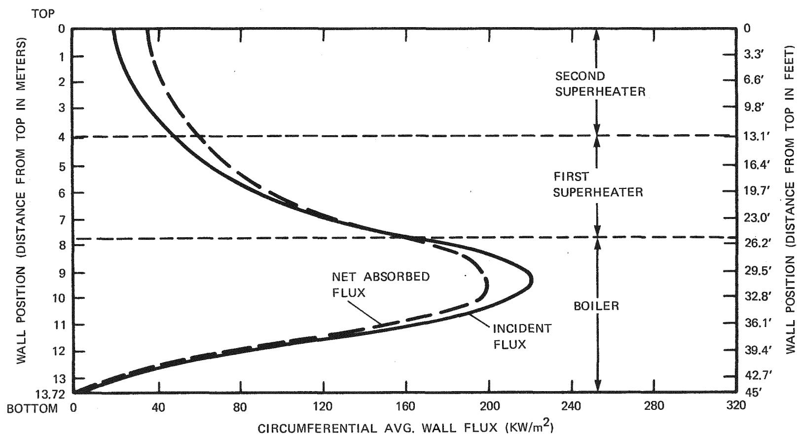
Figure A-3. Circumferential Average Flux for the Bare Ceiling Configuration at 6/21 Noon
