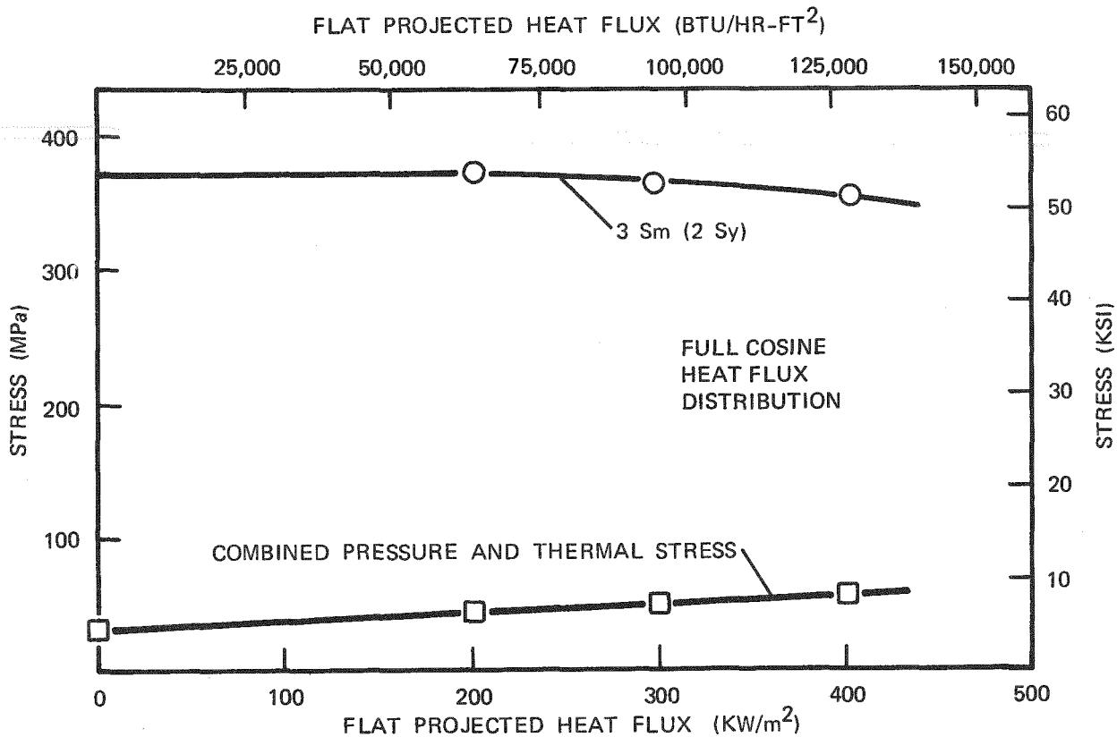
Figure D-12. Comparison of the Combined Pressure and Thermal Stress in the SRE Superheater Tubing to the Allowable Stress
