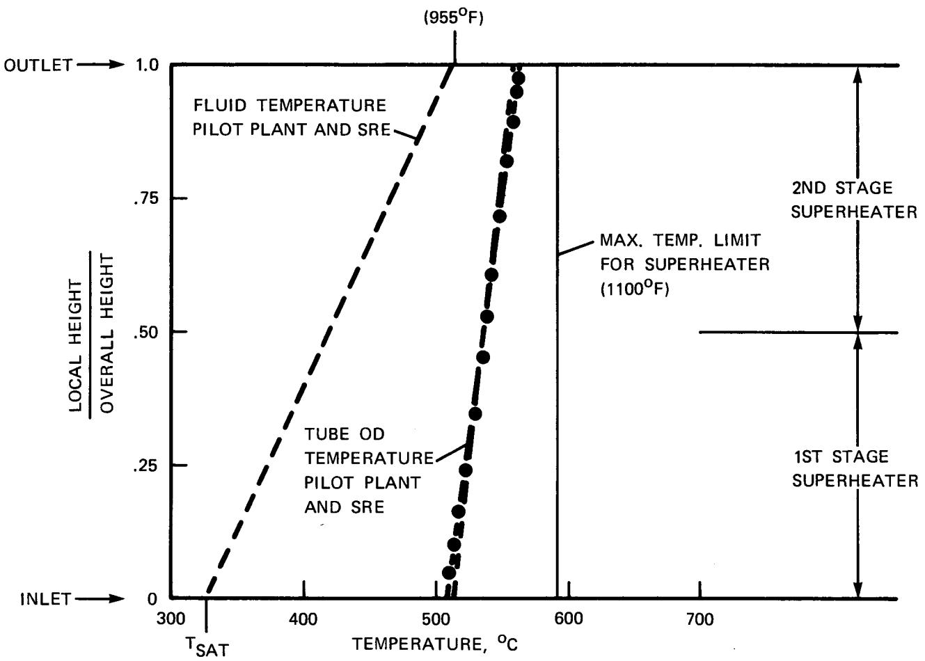
Figure 3-11. Fluid and OD Tube Temperatures - Superheater
