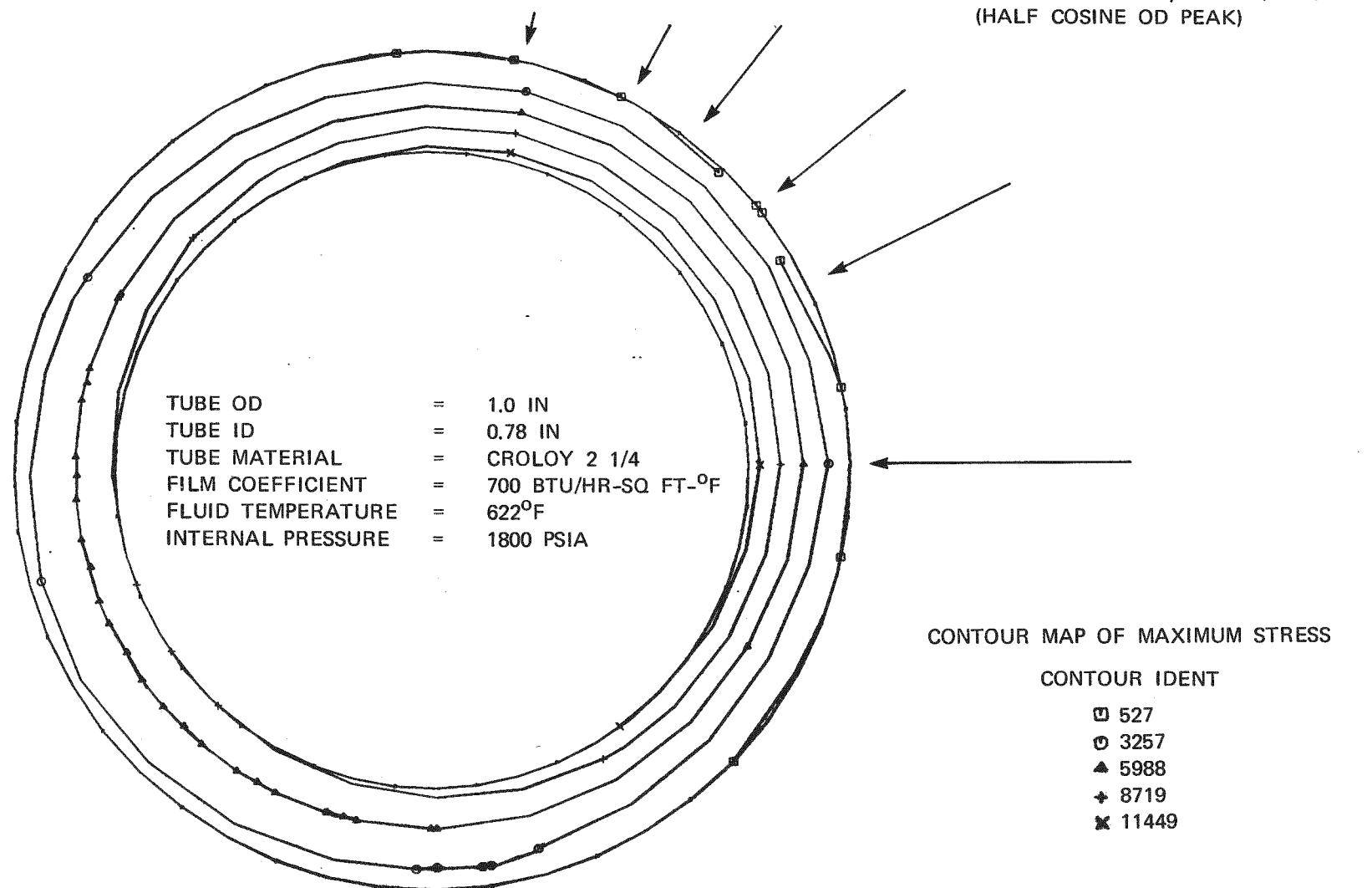
Figure D-11. Maximum Principal Stress Contour Lines in Pilot Plant Superheater Tube Due to Internal Pressure and Heat Flux of 127,000 Btu/Hr-Sq Ft
