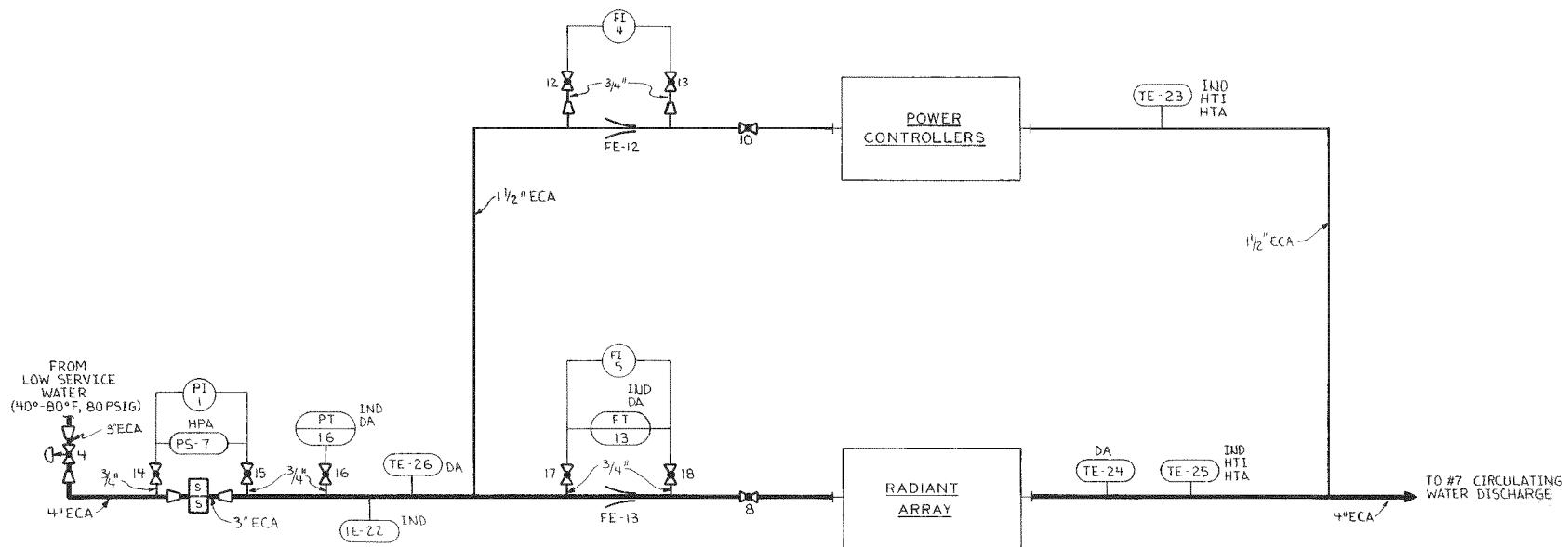
Figure I-1. Piping and Instrument Diagram Cooling Water System
