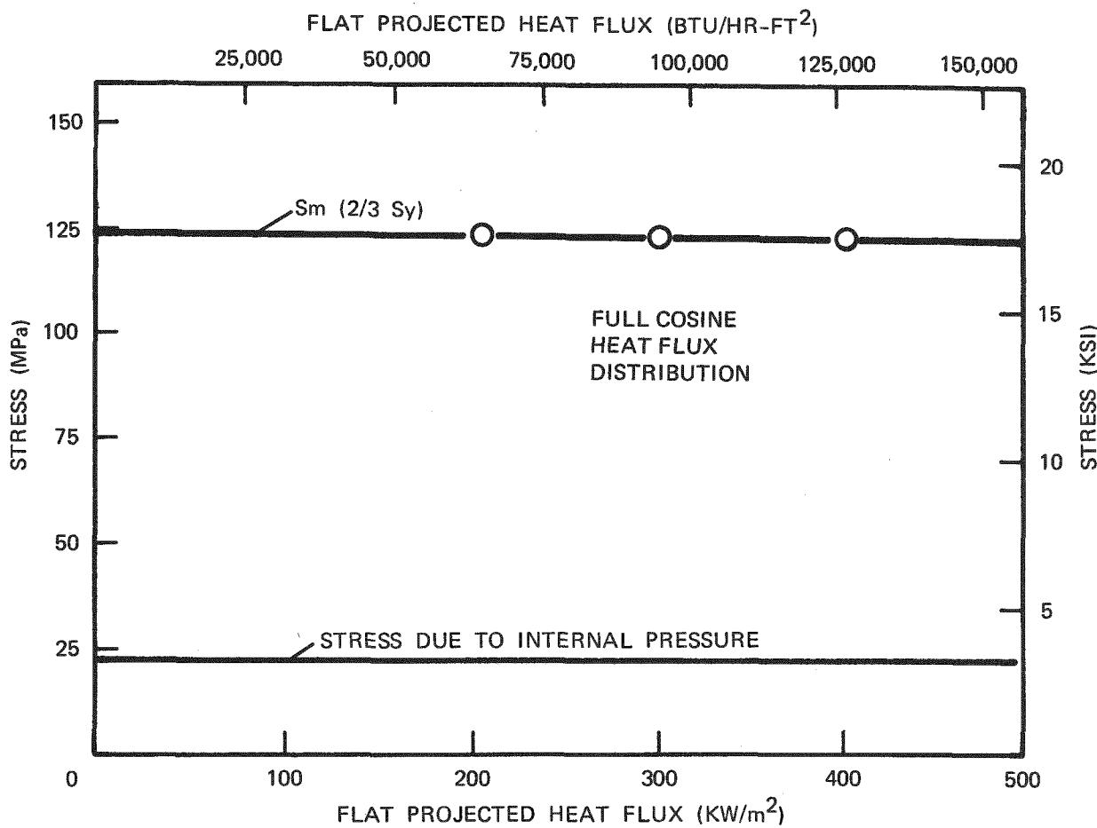
Figure D-7. Comparison of the Pressure Stress in the SRE Superheater Tubing to the Allowable Stress
