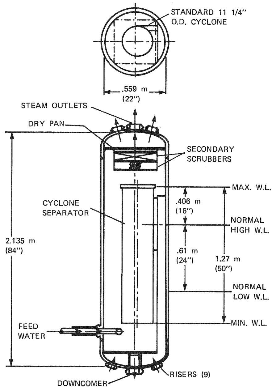
Figure 3-17. SRE Drum and Internals
