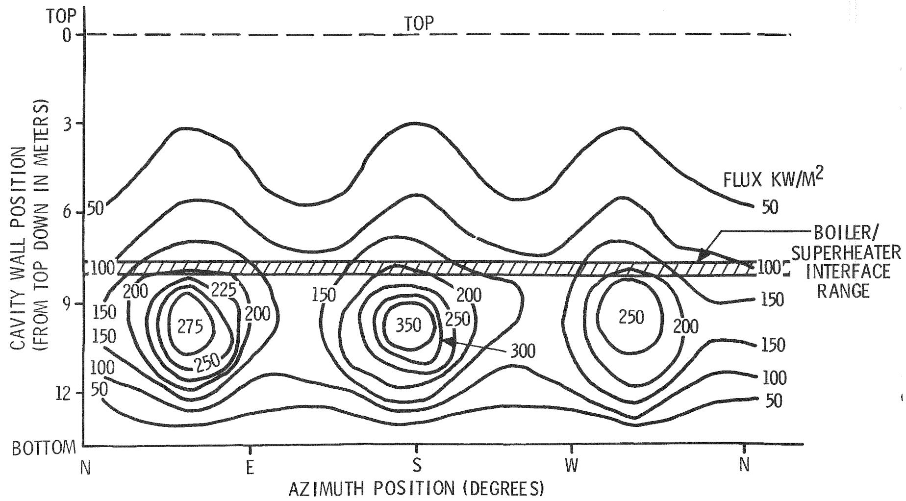
Figure J-1. Cavity Wall Incident Flux Map for 6/21 Noon
