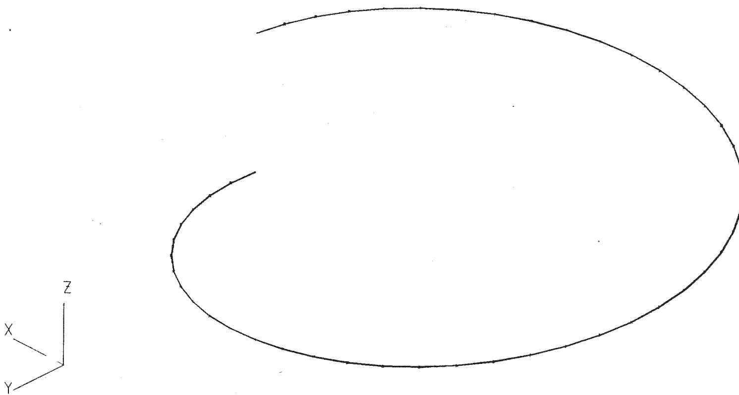
Figure D-17. Three Dimension Finite Element Model of Superheater Tube
