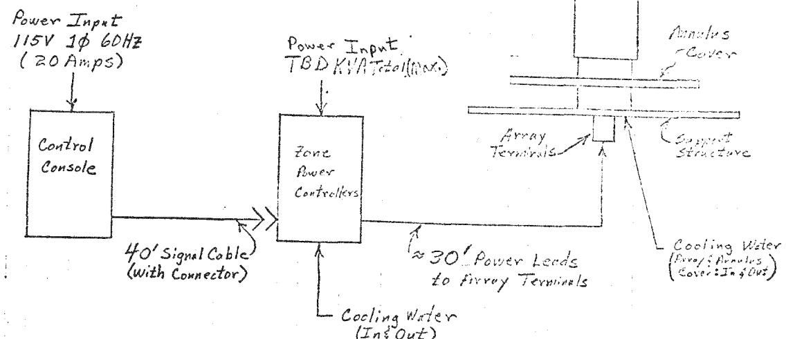
Figure 1 Solar Simulator System Schematic
