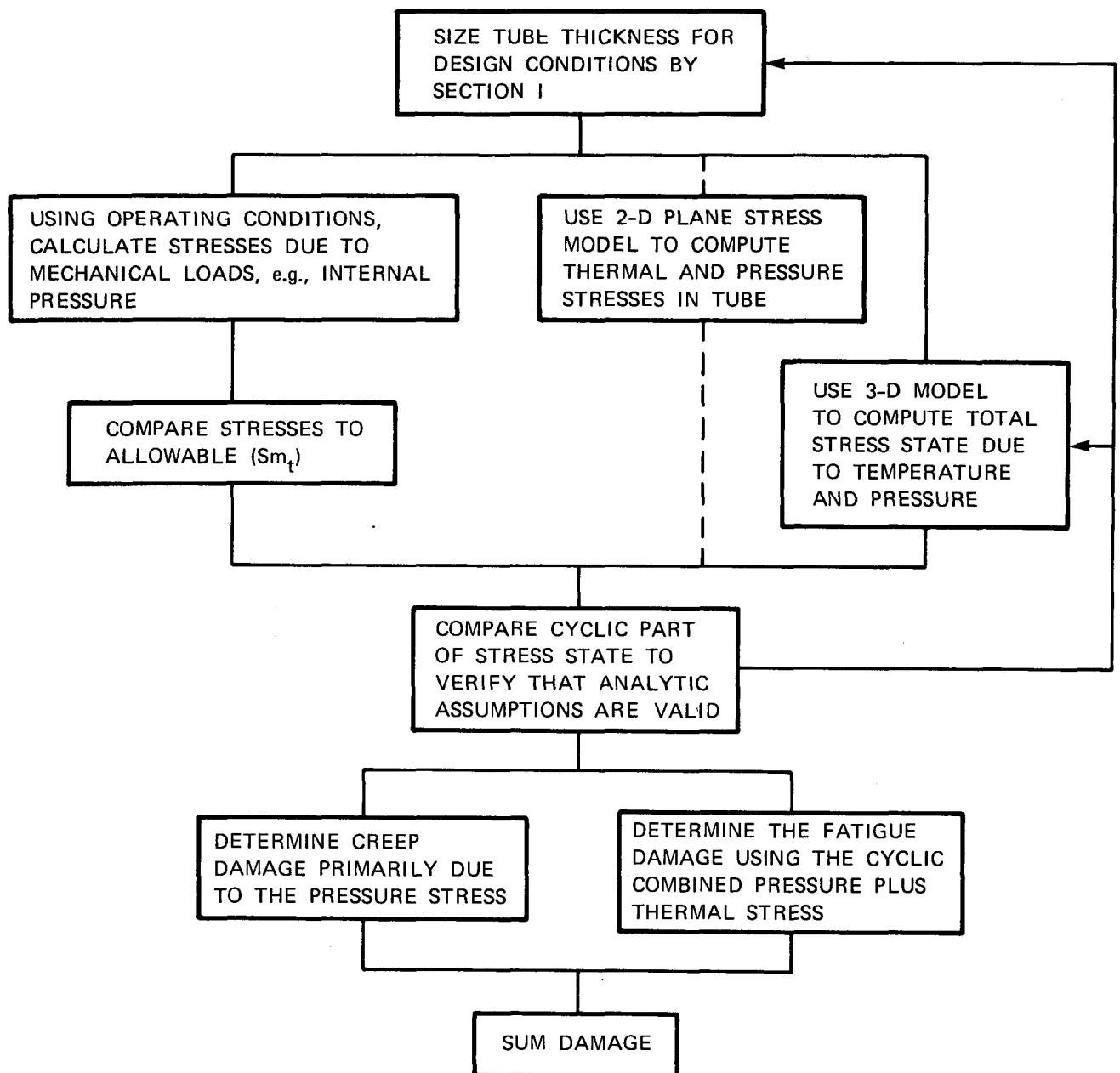
Figure 3-12. Superheater Stress Analysis
