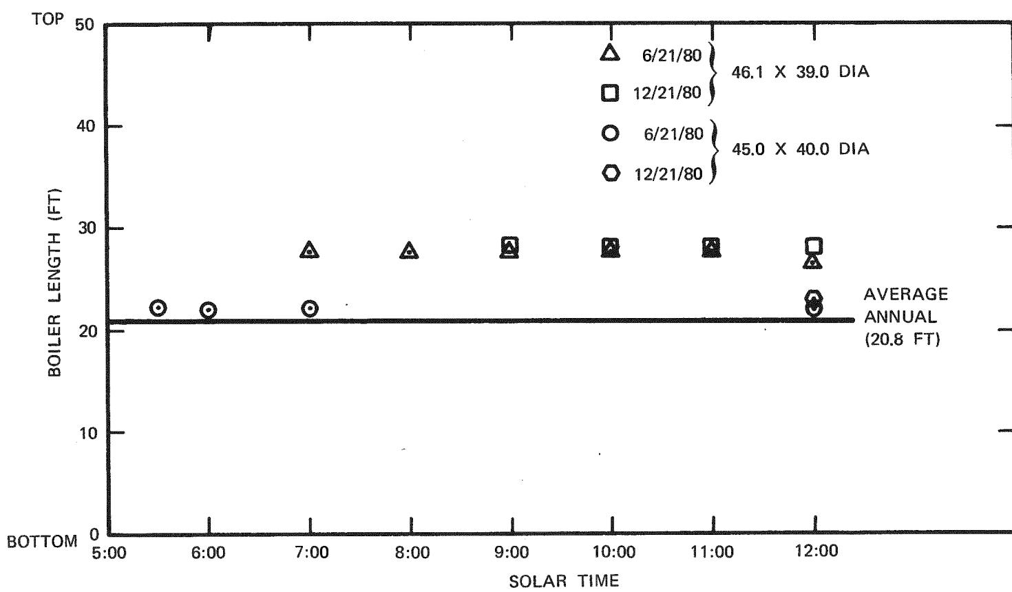
Figure A-5. Boiler Length versus Solar Time
