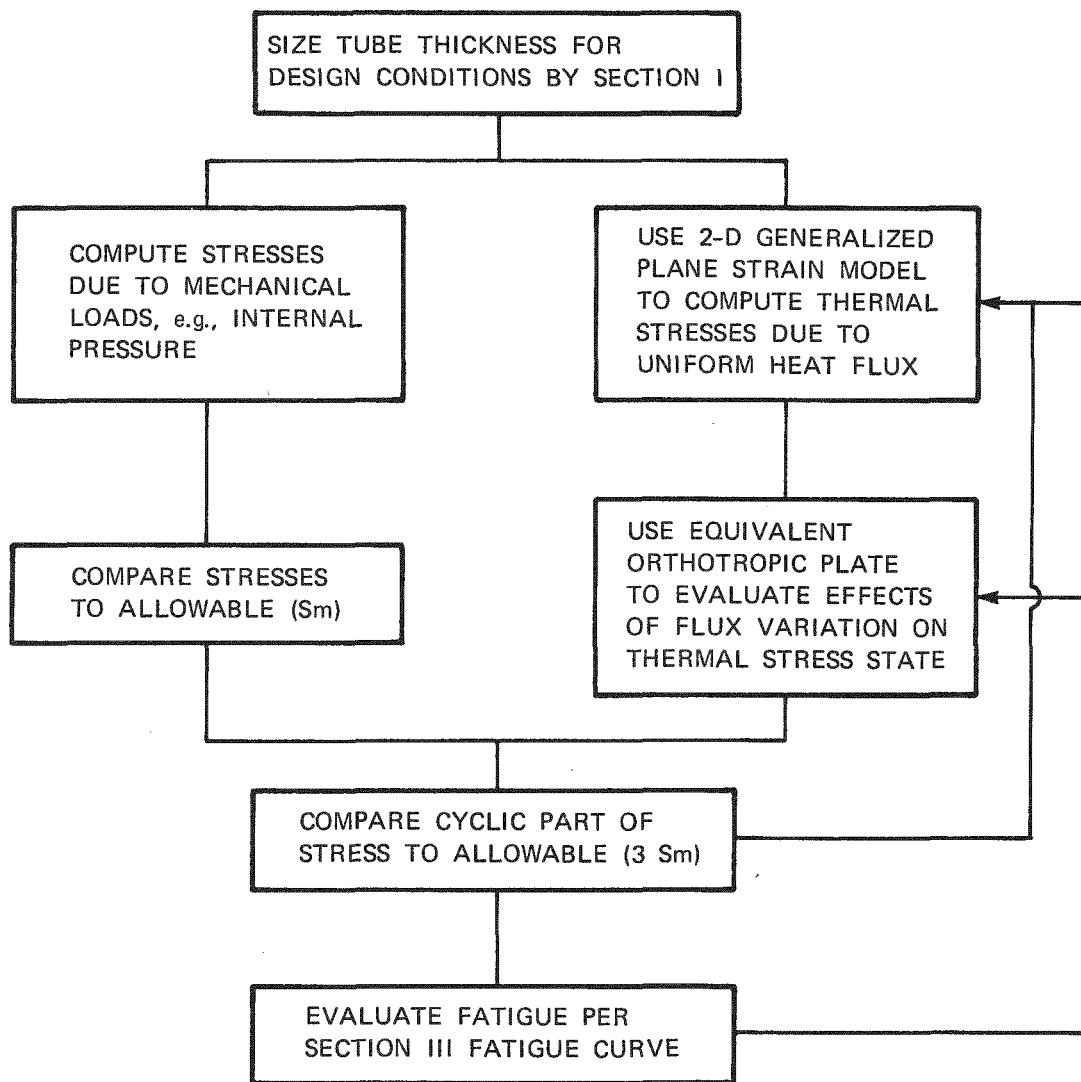
Figure 3-7. Boiler Section Stress Analysis
