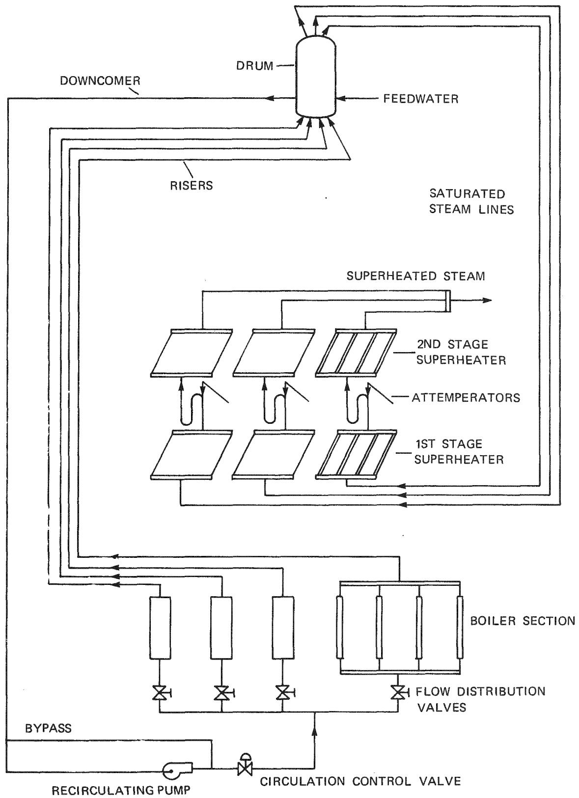
Figure B-1. Thermal and Hydraulic Model of the Solar Steam Generator
