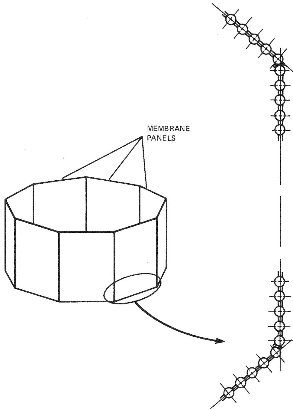
Figure 3-4. SRE Boiler Surface Arrangement
