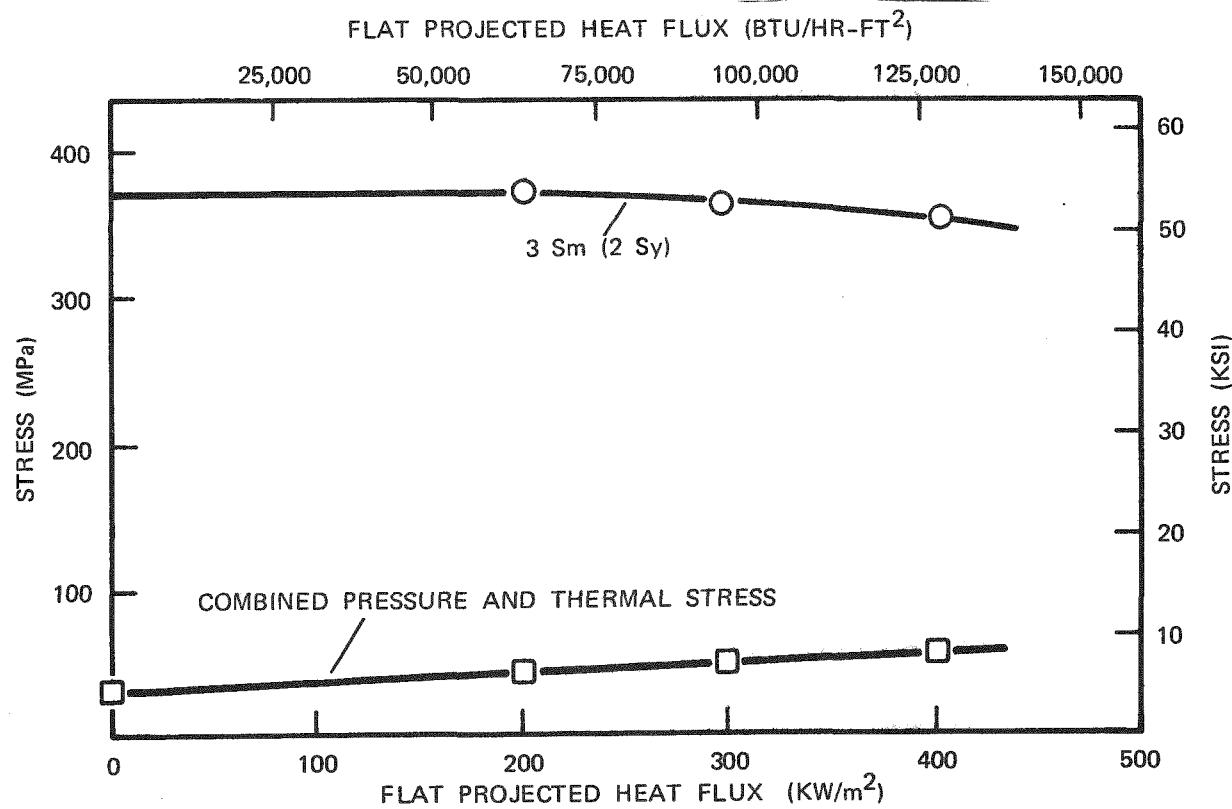
COMPARISON OF THE COMBINED PRESSURE AND THERMAL STRESS TO THE ALLOWABLE STRESS
