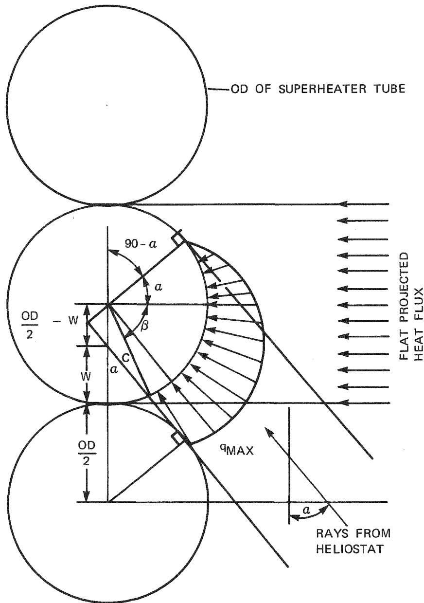
Figure E-2. Heat Flux Distribution - Superheater Tubes
