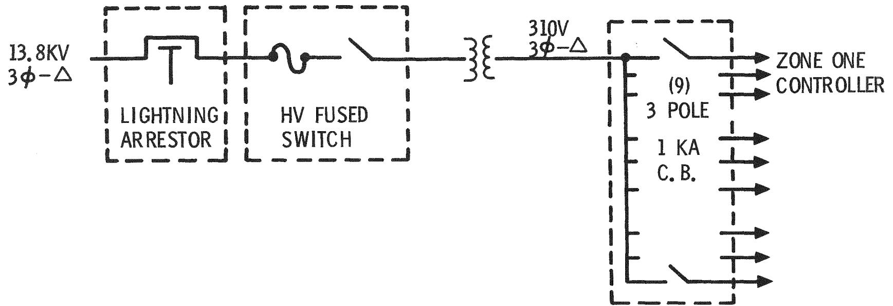
Figure 6-11. Solar Simulator Substation
