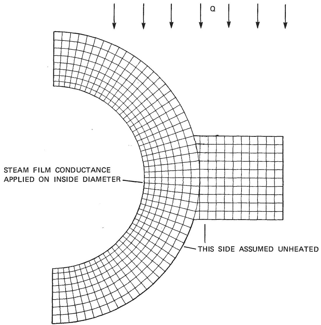
Figure D-2. Finite Difference Mesh used for Generalized Plane Strain Analysis of Boiler Section
