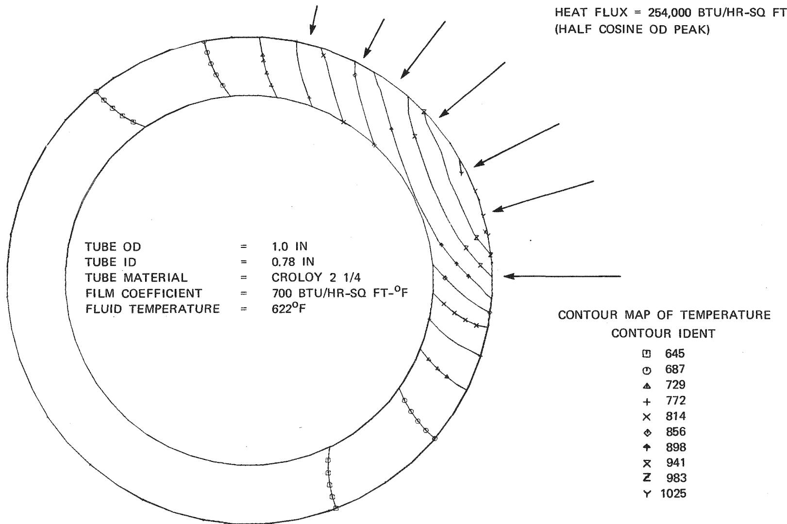
Figure D-10. Temperature Contour Lines in Pilot Plant Superheater Tubes
