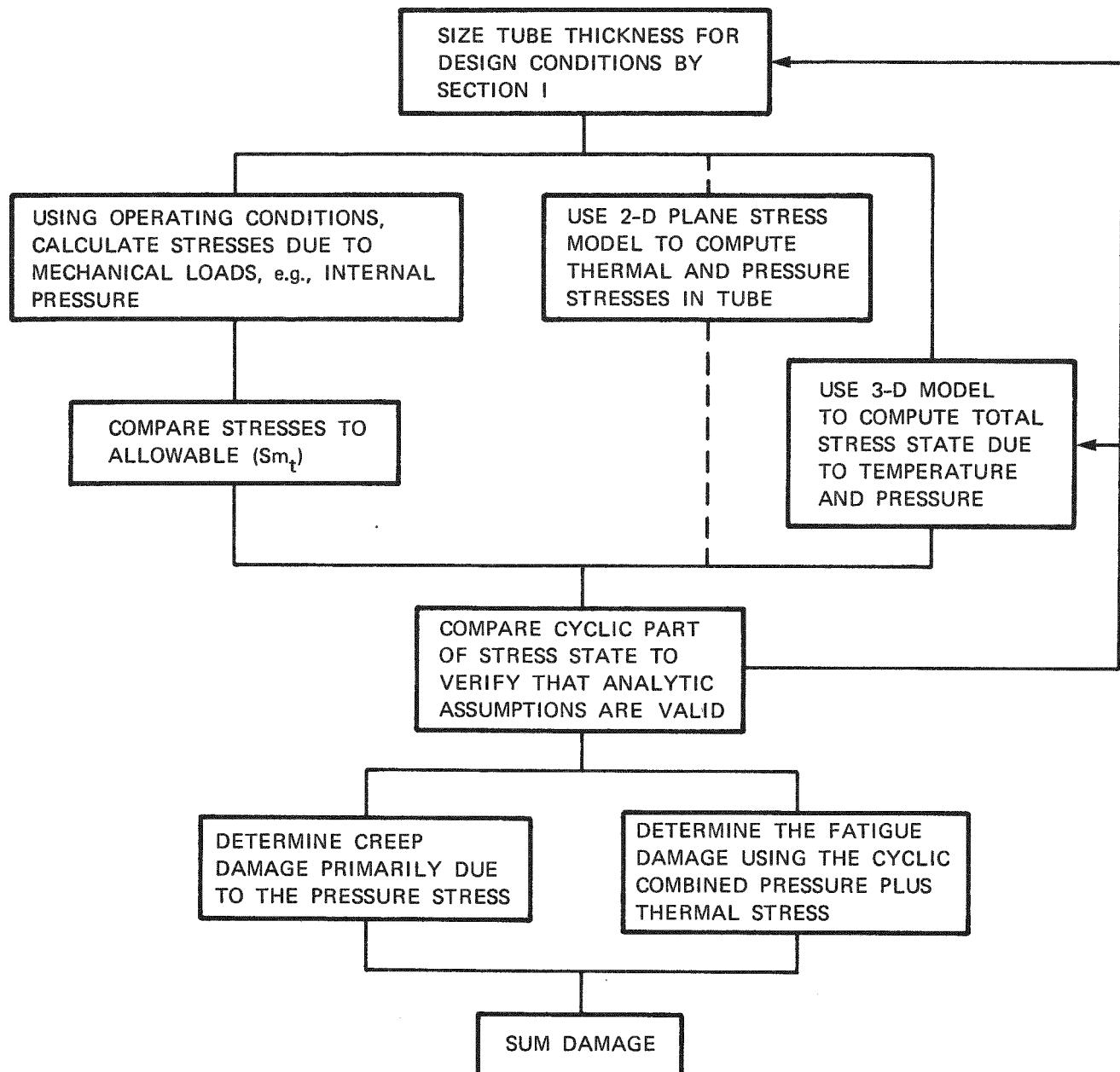
Figure C-2. Superheater Stress Analysis
