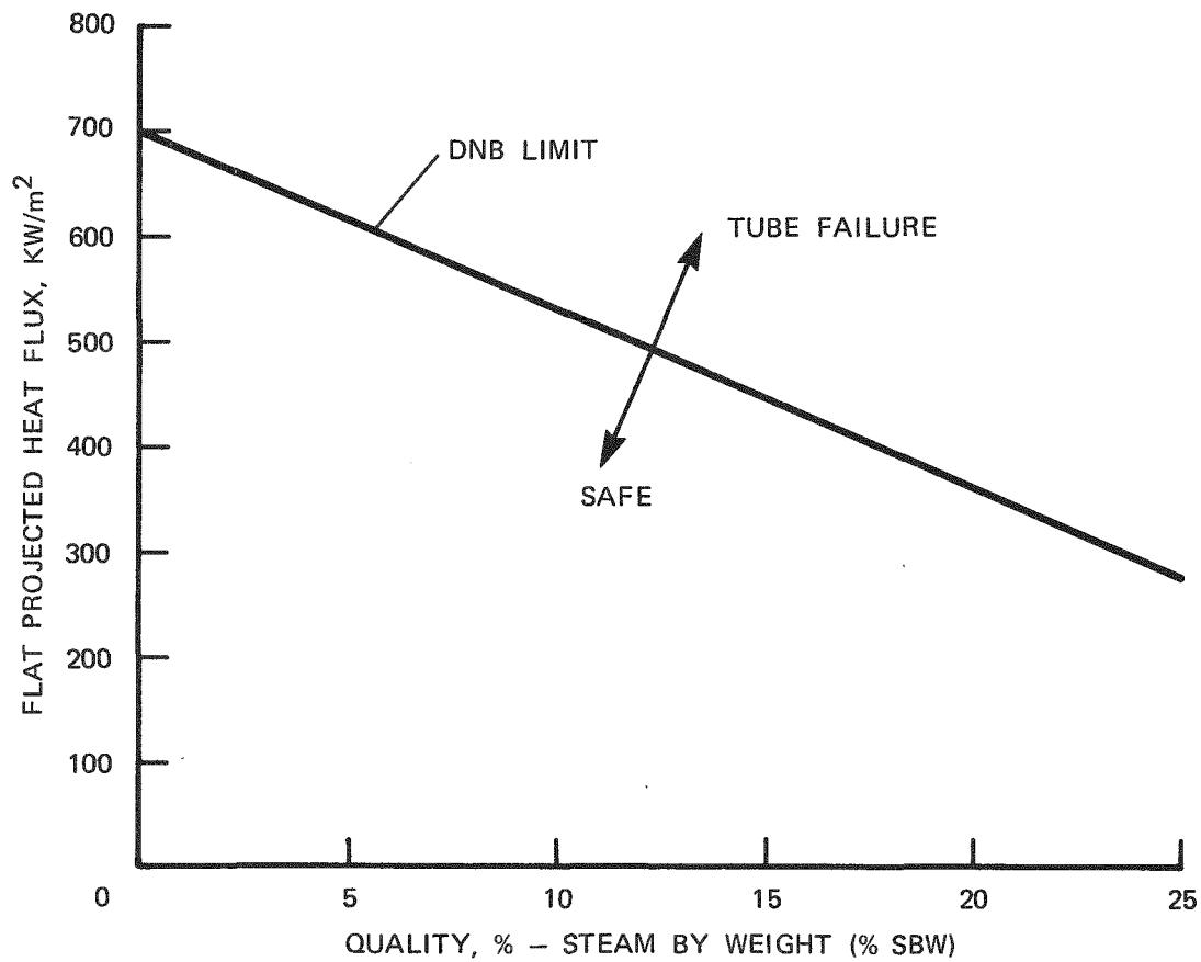
Figure 3-5. DNB Limit for the Boiler Section
