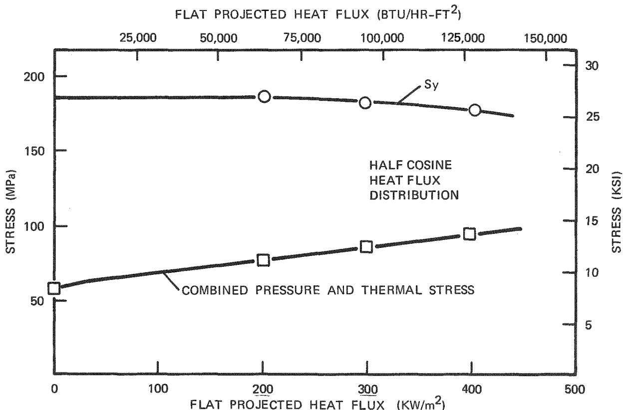
Figure D-13. Comparison of the Combined Pressure and Thermal Stress in the Pilot Plant Superheater Tubing to the Allowable Stress
