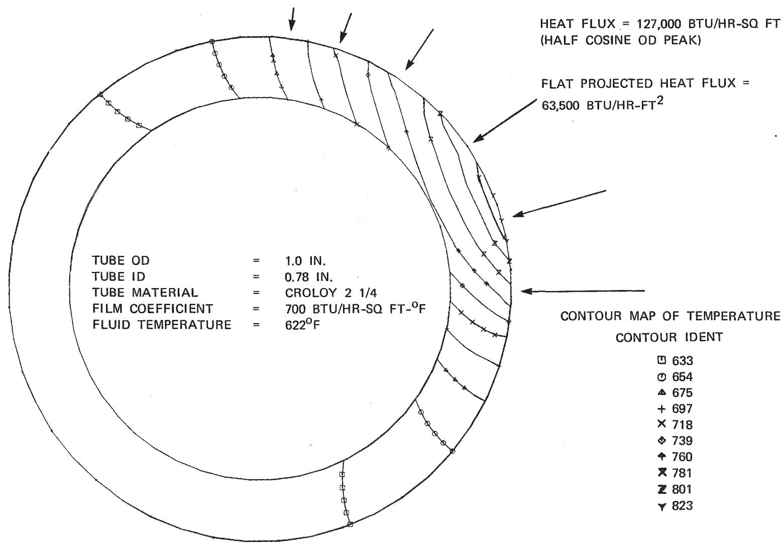
Figure D-16. Temperature Contour Lines in Pilot Plant Superheater Tube Due to Half Cosine OD Peak Heat Flux
