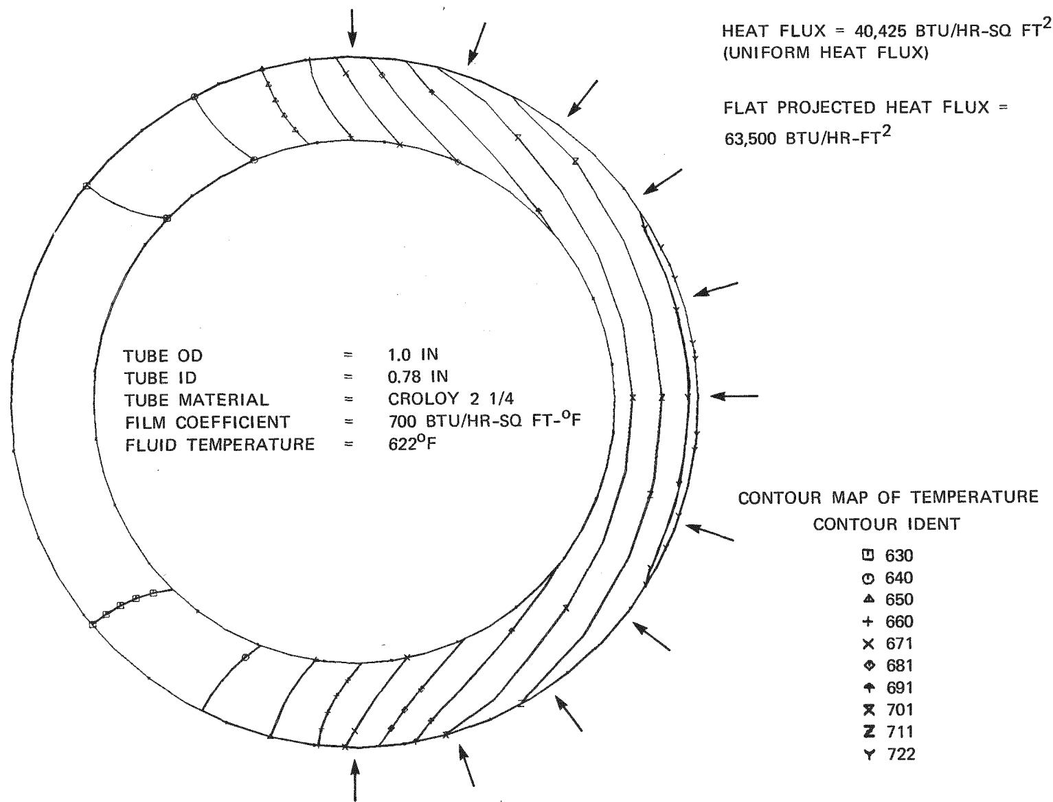
Figure D-14. Temperature Contour Lines in Pilot Plant Superheater Tube Due to Uniform Heat Flux
