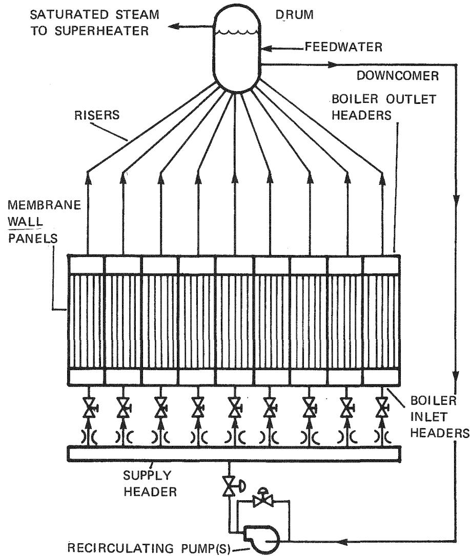
Figure 3-1. Boiler Flow Circuit
