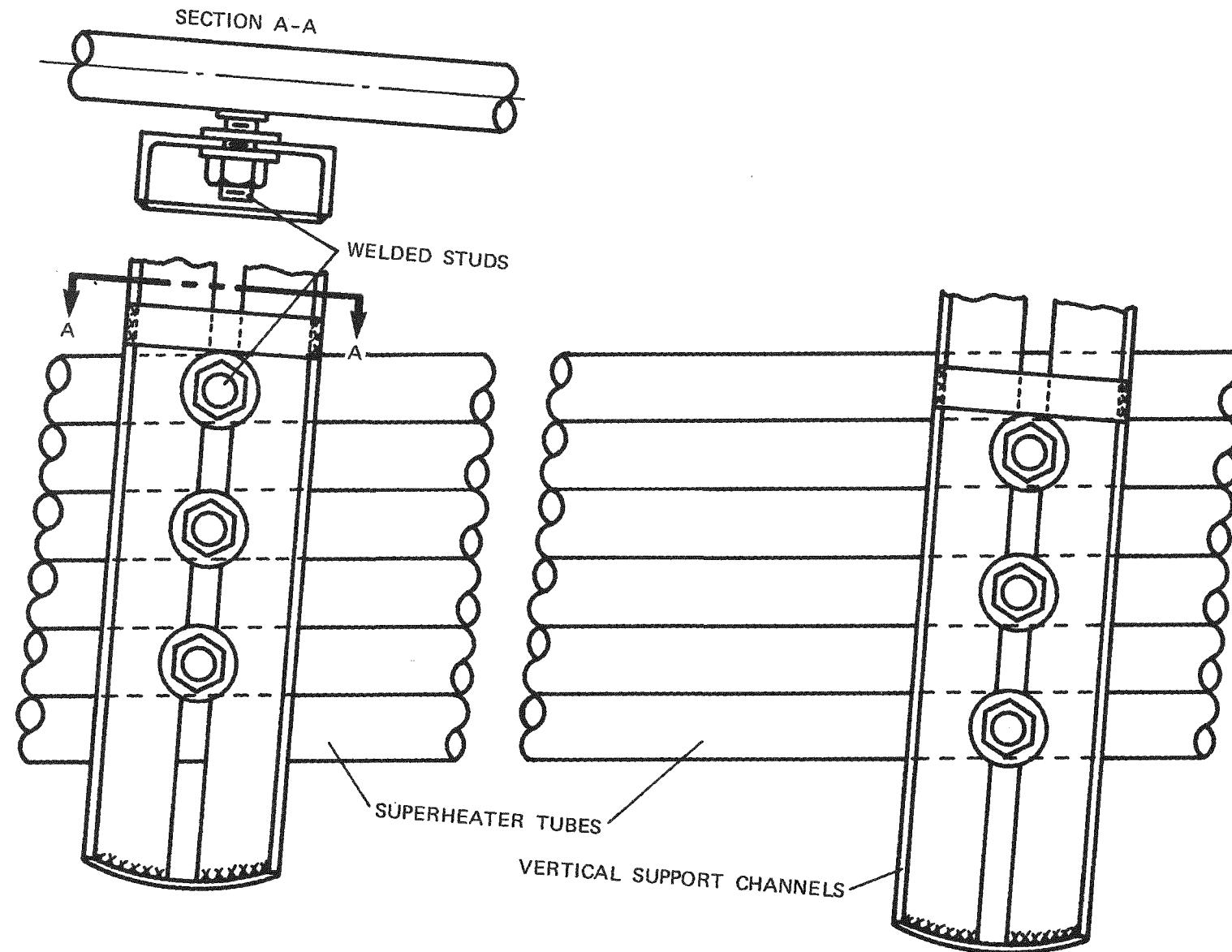
Figure 3-16. Superheater Tube Support Concept
