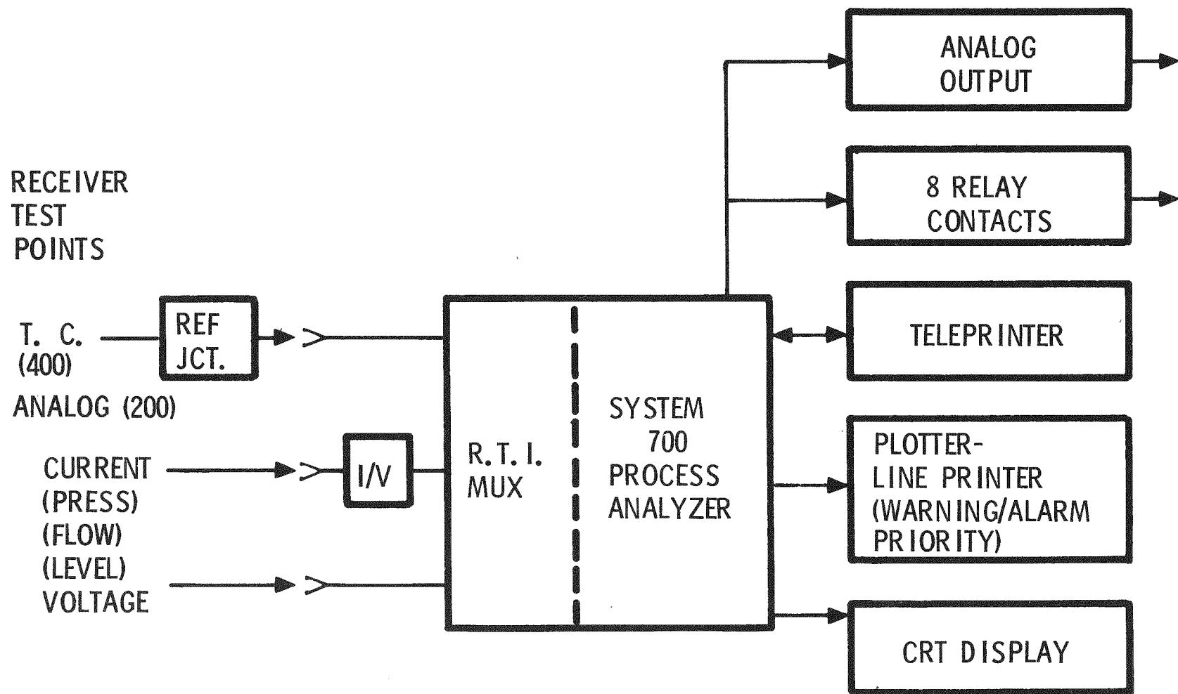
Figure 6-6. SRE Data Acquisition System Configuration
