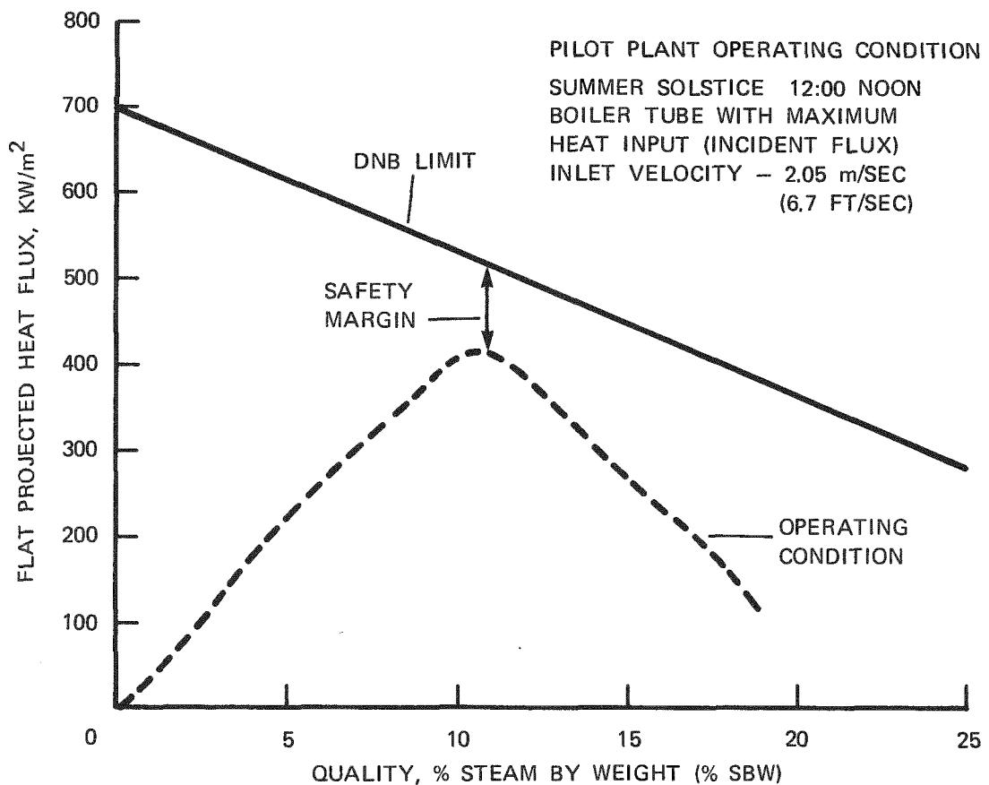
Figure 3-6. Comparison of an Operating Condition to the DNB Limit
