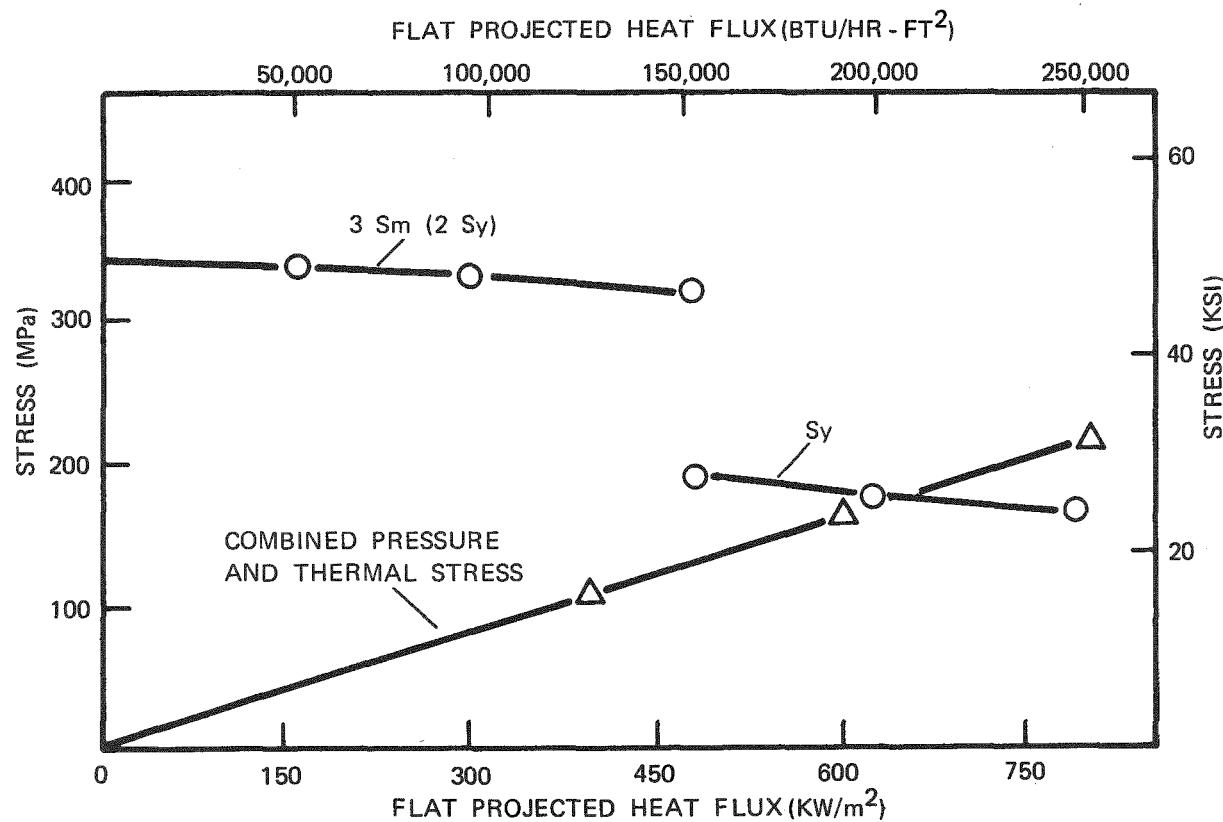
Figure D-5. Comparison of the Combined Pressure and Thermal Stress in Boiler Section to the Allowable Stress
