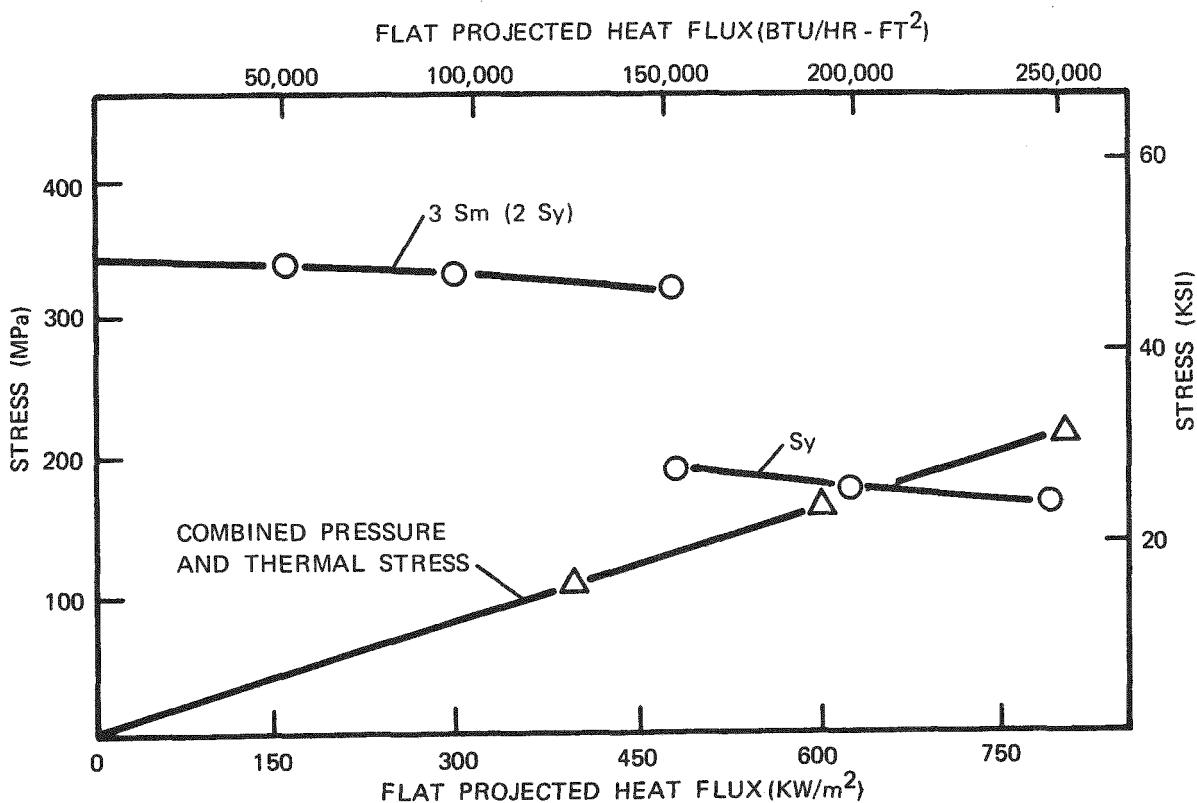
COMPARISON OF THE COMBINED PRESSURE AND THERMAL STRESS IN THE BOILER SECTION TO THE ALLOWABLE STRESS
