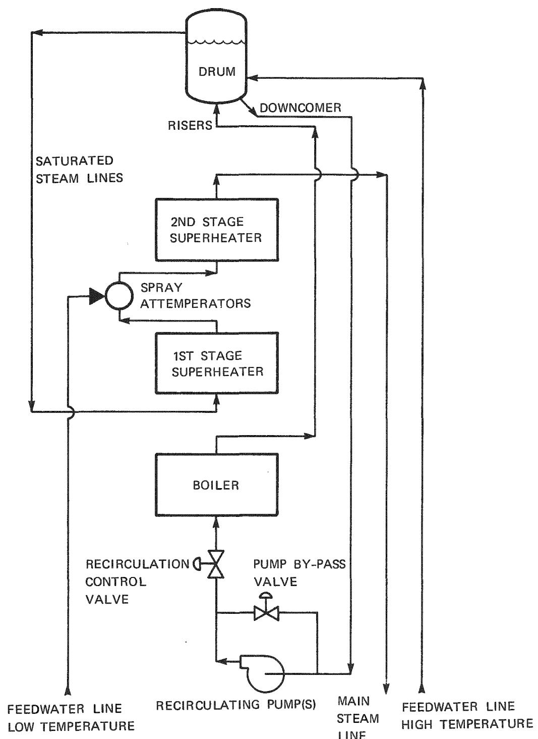
Figure 2-1. Solar Steam Generator - Flow Schematic
