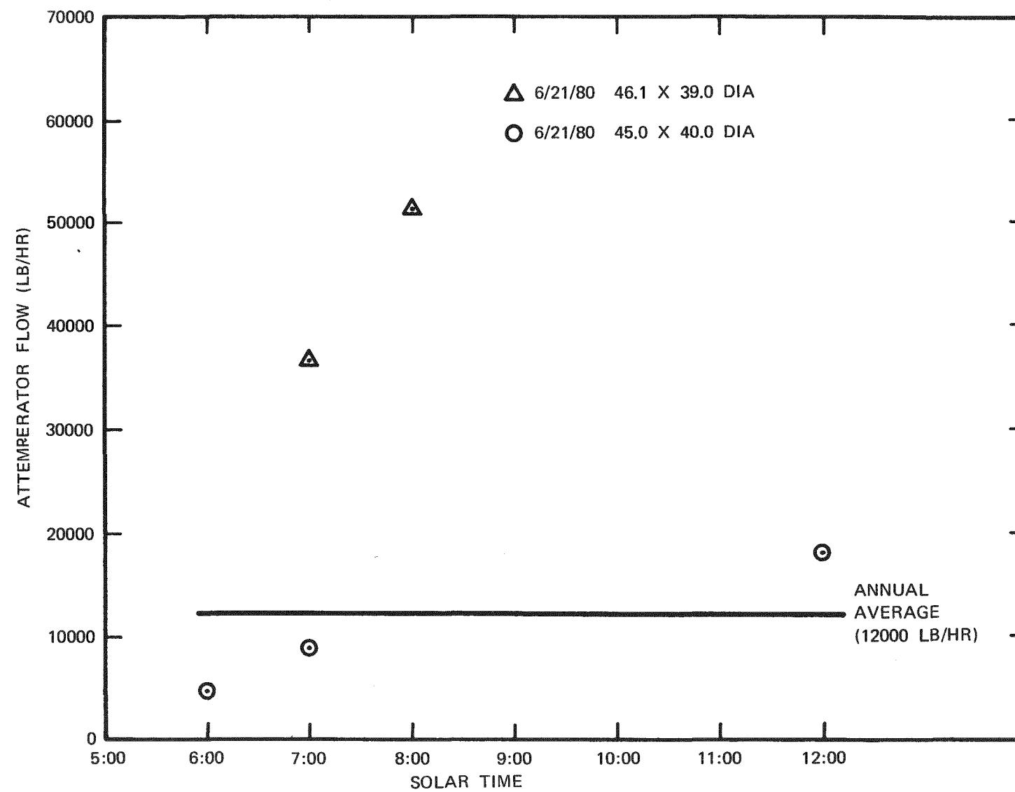
Figure A-6. Attemperator Flow versus Solar Time
