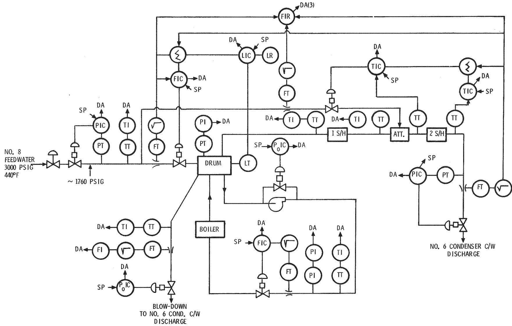
Figure 6-3. Steam Generator Control Schematic
