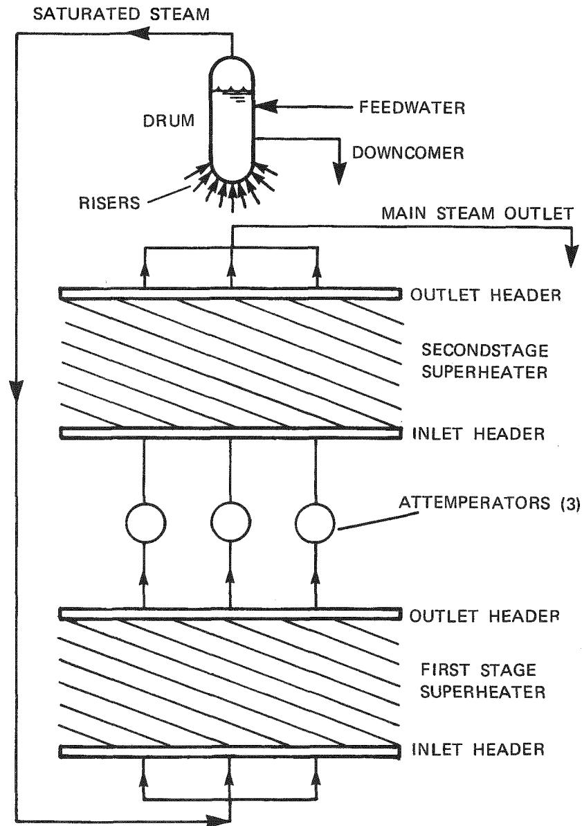
Figure 3-10. Superheater Flow Circuit
