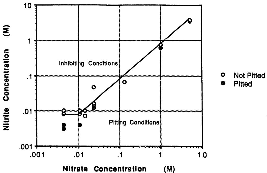
Figure 1. The corrosivity of simulated sludge slurry at 40°C containing the indicated concentrations of nitrate and nitrite. The boundary between inhibiting and pitting conditions was placed by hand. Data from Reference 1.
