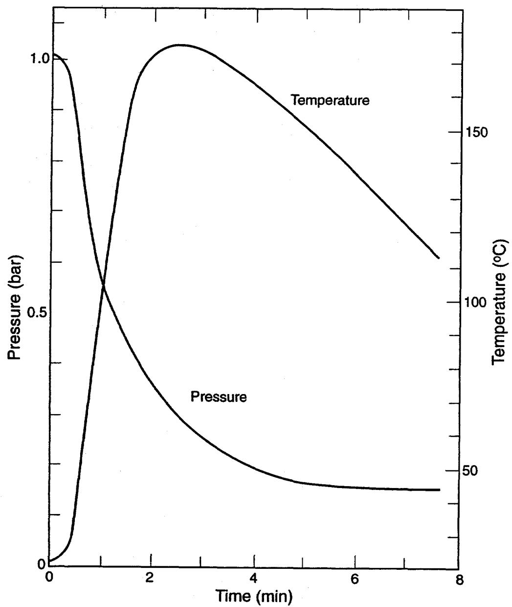
Figure 1. Time dependence of pressure and gas temperature for reaction of air with a mixture of 60% PuOH and 40% Pu in a closed system.
