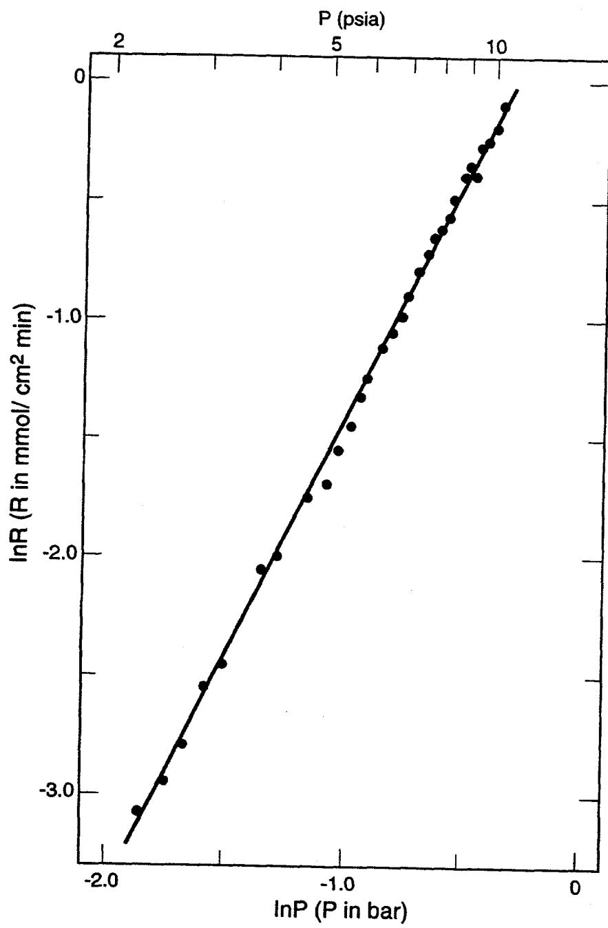
Figure 4. Dependence of  $\ln R$  on  $\ln P$  for reaction of air with a mixture of 60% PuOH and 40% Pu in a closed system.
