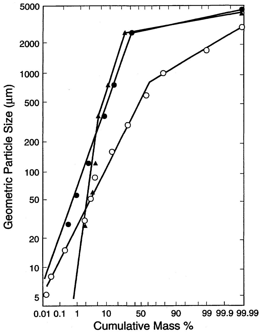
Figure 5: Cumulative mass-size distributions for products formed by corrosion of plutonium metal. Data for products of the  $\text{Pu}+\text{O}_2$  reaction at temperatures above the  $500^\circ\text{C}$  ignition point of the metal [21], the hydride-catalyzed oxidation of Pu by  $\text{O}_2$  [4], and the hydride-catalyzed corrosion of Pu by air [4] are indicated by open circles, filled circles, and triangles, respectively.
