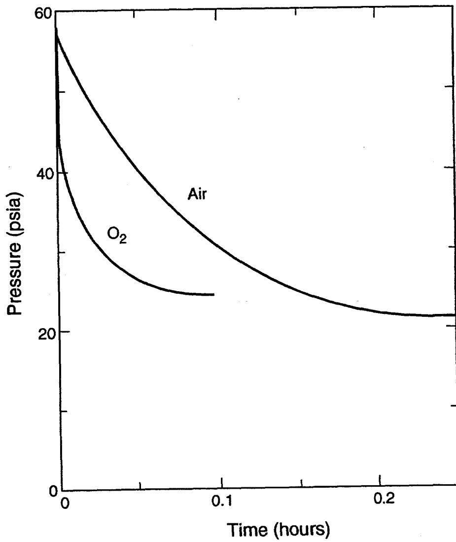
Figure 2. Time dependence of pressures for the reactions of air and oxygen with hydride-coated plutonium in a closed system [4].
