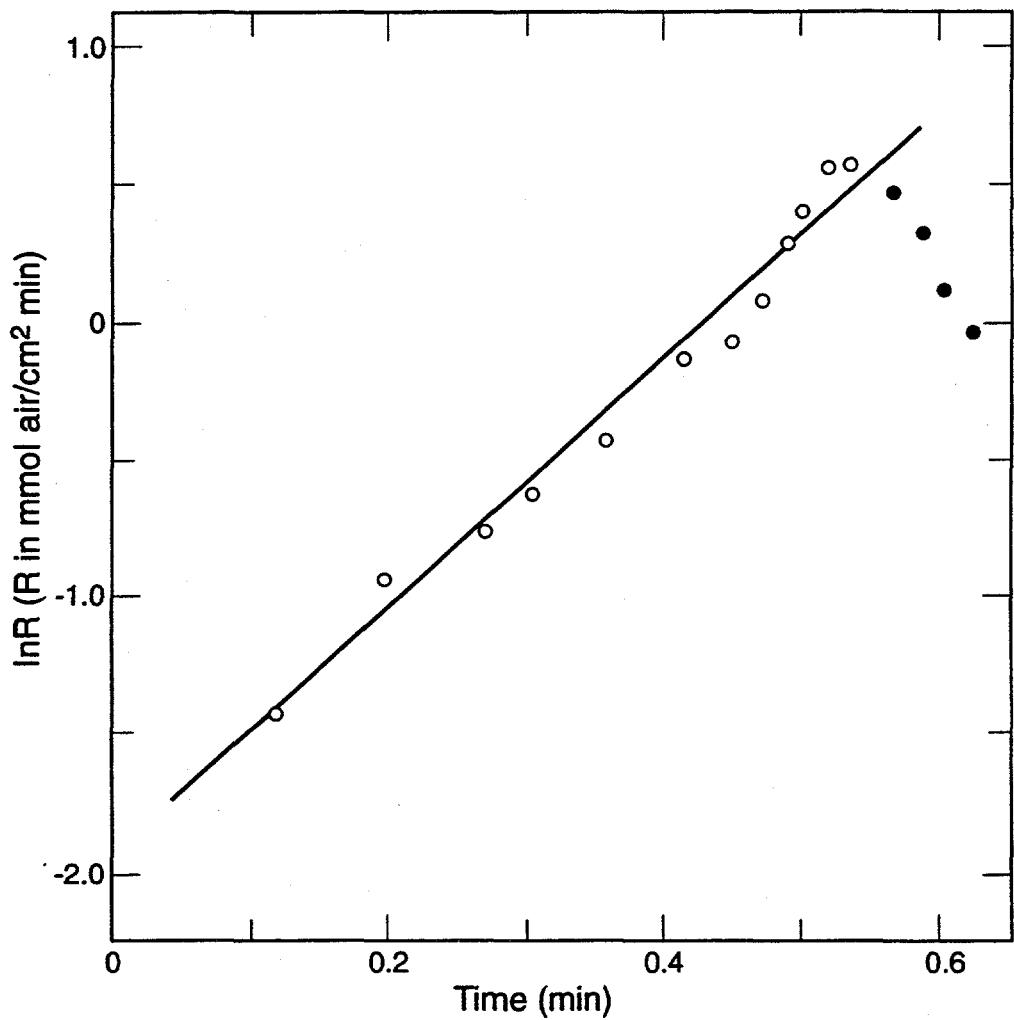
Figure 3. Time dependence  $\ln R$  for reaction of air with a mixture of 60% PuOH and 40% Pu in closed system. Corrosion rates measured during the initial first-order stage of reaction are indicated by open symbols; corrosion rates measured during the second stage of reaction are indicated by filled symbols.
