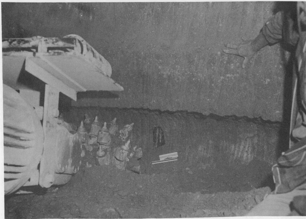
Fig. III-4 - View of Alpine Miner's Cutting Head and Uncovered Grout-Filled Fracture and Borehole.
