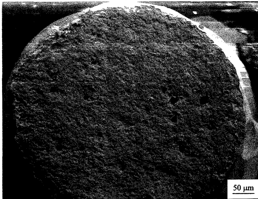
Figure 3.2-3. SEM micrograph of the fracture surface of a BGA sample assembled on soft Au/Cu pads and no flux (set 2).
