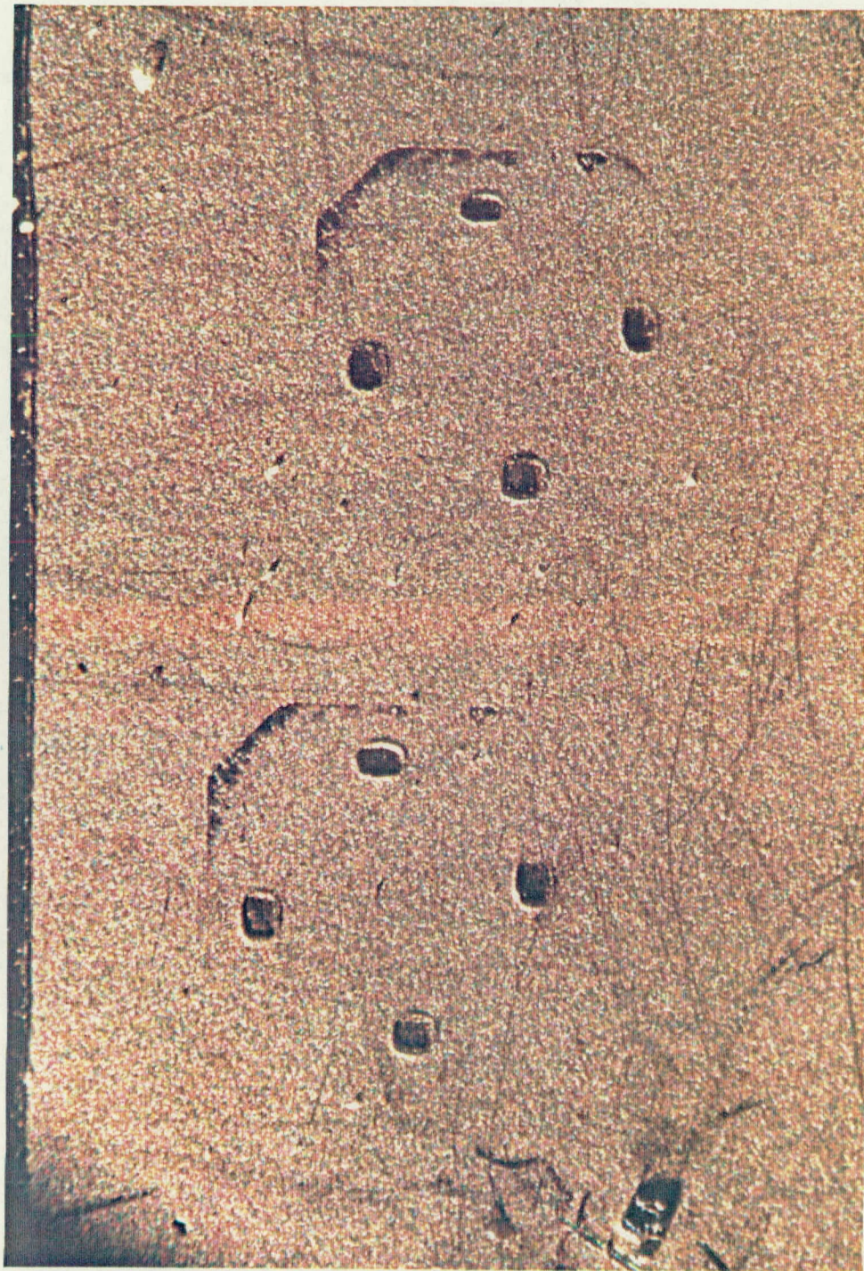
Figure 10. Evidence of Uneven Wobble Bonder Pressure
