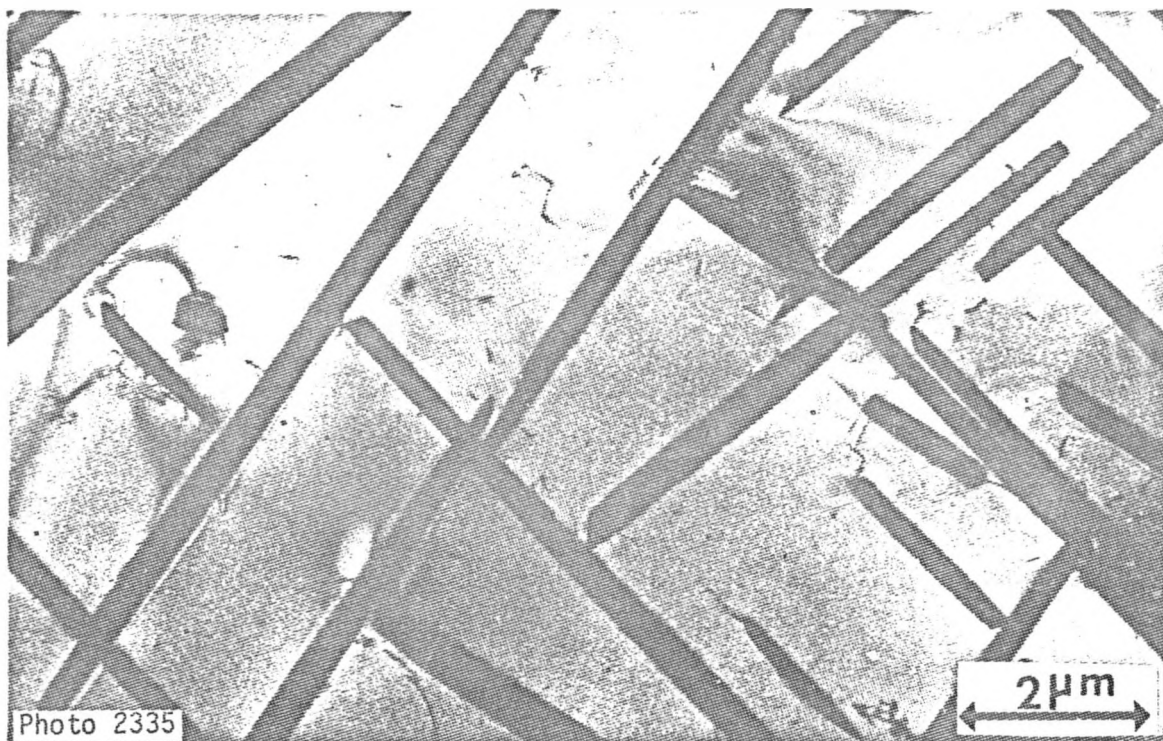
Widmanstätten \eta phase in Neutron Irradiated STA Inconel 706 After 3.4 \times 10^{22} n/cm 2 (E > 0.1 MeV) (6,700 Hours) at 735°C.
