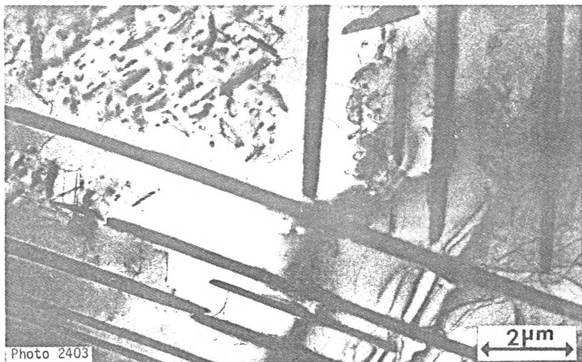
Thermally-Aged Inconel 706 Showing Widmanstätten \eta Phase and Undissolved \gamma' and \gamma'' After 7,000 Hours at 735°C.
